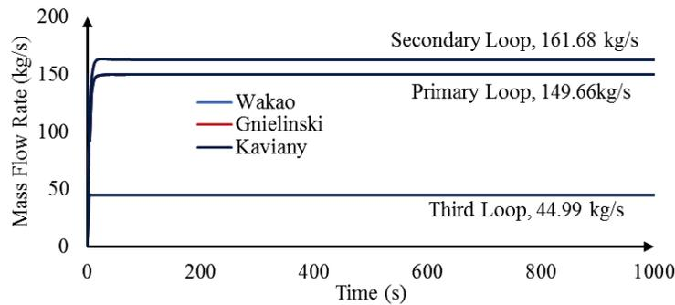
**Figure 4. Mass Flow Rate of the System at Steady State**
