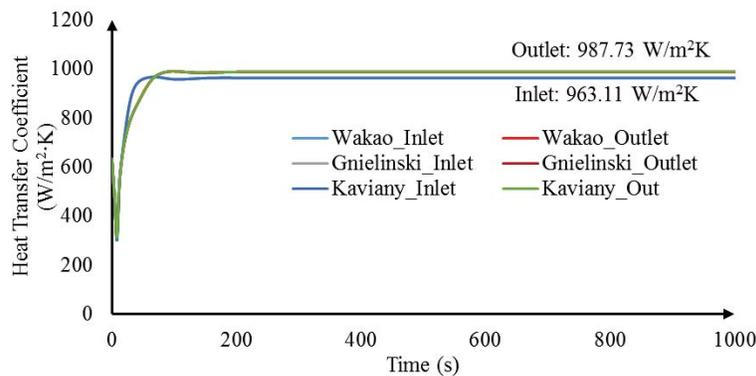
**Figure 6. Heat transfer coefficient of the Pebble Beds**
