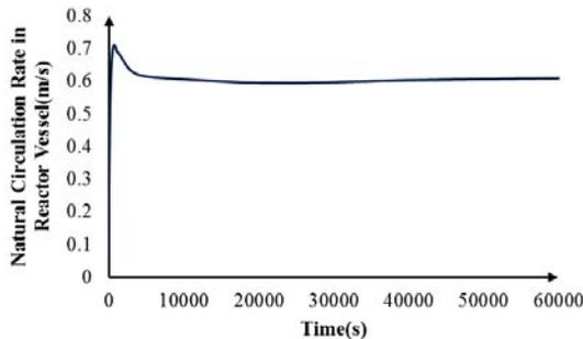
**Figure 11. Natural Circulation Rate in the Reactor Vessel**
