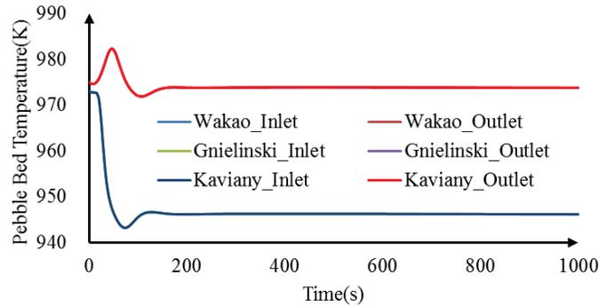
**Figure 3. Molten Salt Temperature at Pebble Bed Inlet/Outlet**
