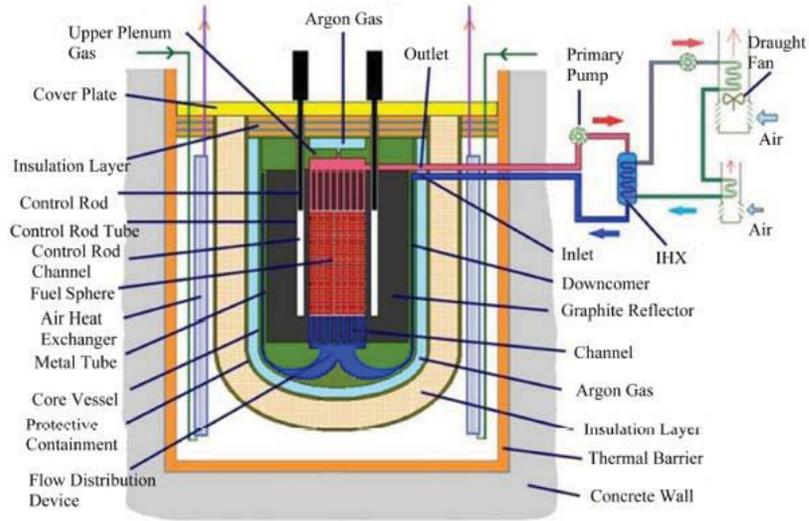
**Figure 1. Schematic of TMSR-SF1 System**
