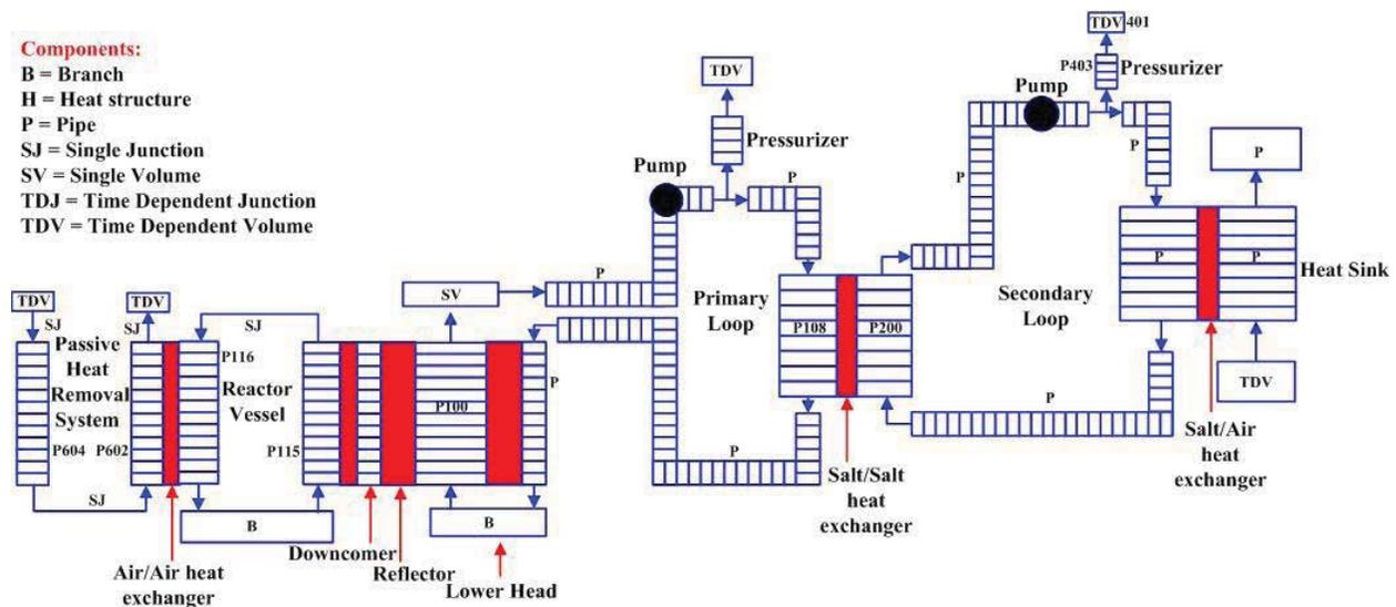
Figure 2. RELAP5/MOD4.0 Nodalization of TMSR-SF1 System
