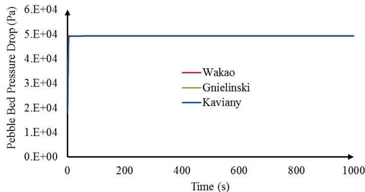
**Figure 5. Pebble Bed Pressure Drop at Steady State**
