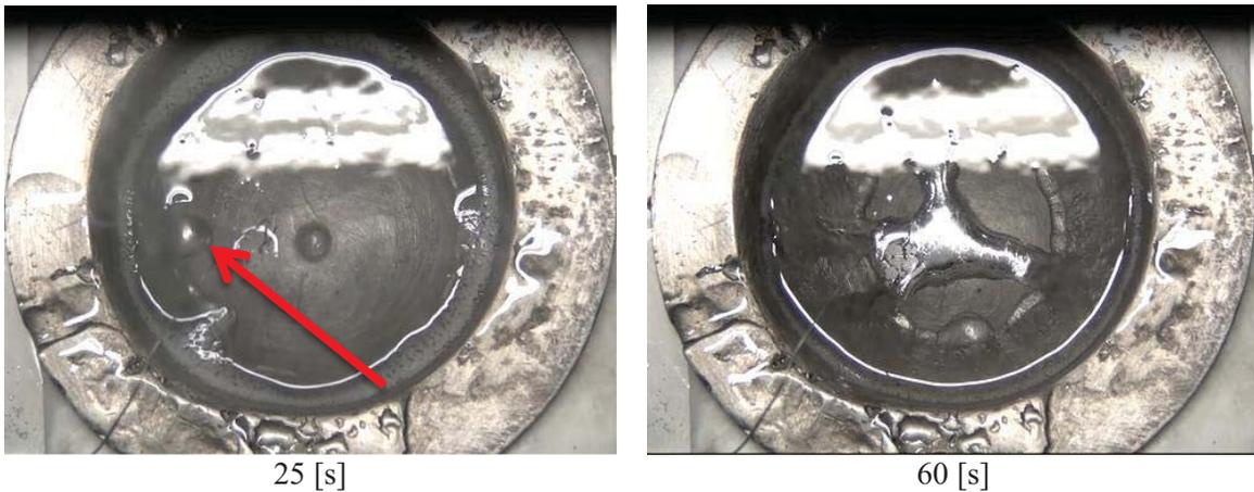
Figure 7. Picture of vessel wall ablation in the experiment.
