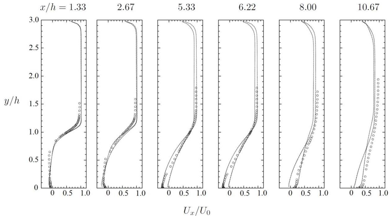
**Figure 4. Streamwise velocity component,  $\pm 3\sigma$ , maximum and minimum. Results using the binary ensemble (solid lines), the 2nd ensemble (dashed lines), and the 3rd ensemble (dotted lines). Measurements [17] (circles). The results from the three ensembles are indistinguishable.**
