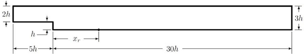
Figure 3. Backward-facing step geometry
