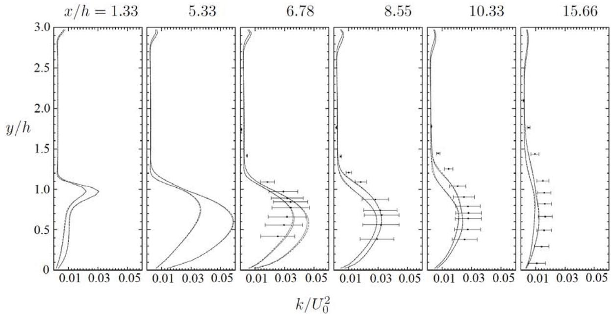
**Figure 5. Turbulent kinetic energy,  $\pm 3\sigma$ , maximum and minimum. Results using binary ensemble (solid lines), 2nd ensemble (dashed lines), and 3rd ensemble (dotted lines). Measurements [17] (uncertainty bars). Results from the three ensembles are for the most part indistinguishable.**
