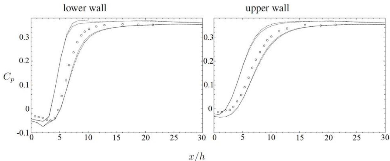
**Figure 6. Pressure coefficient distribution,  $\pm 3\sigma$ , on walls after the step. Results using binary ensemble (solid lines), 2nd ensemble (dashed lines), and 3rd ensemble (dotted lines). Measurements [17] (circles). The results from 2<sup>nd</sup> and 3<sup>rd</sup> ensemble are indistinguishable.**
