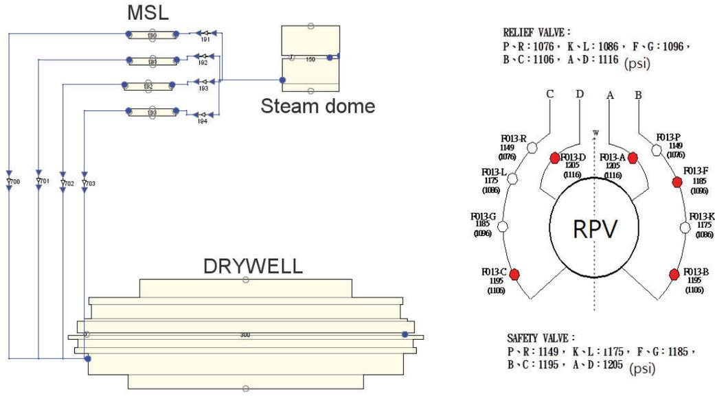
Figure 8. Main steam line and SRVs of the model
