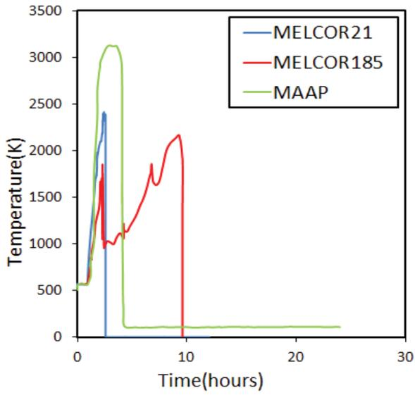
Figure 15. Max hot rod temperature
