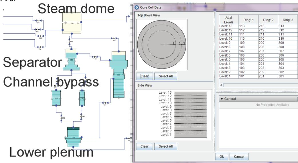
**Figure 6. Reactor pressure vessel of the model**
