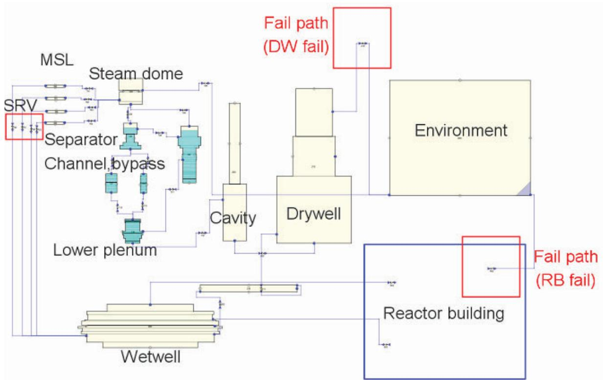
Figure 3. Chinshan NPP MELCOR2.1/SNAP model
