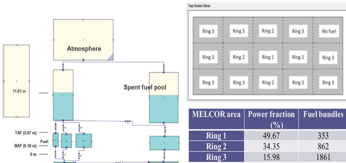
Figure 10. Chinshan NPP spent fuel pool model of MELCOR2.1/SNAP
