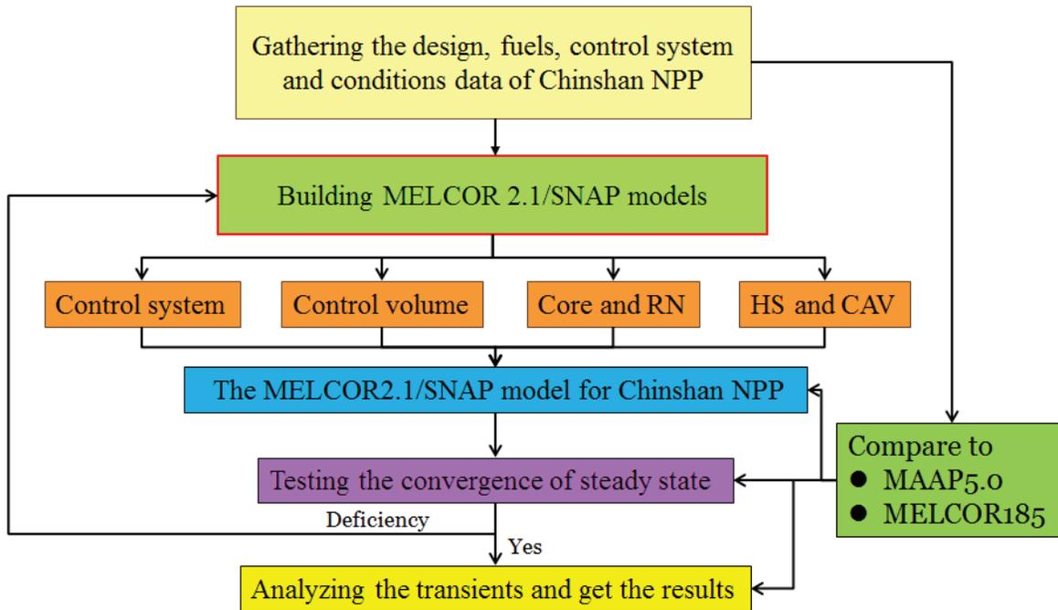
Figure 2. Flow chart to establish Chinshan NPP MELCOR2.1/SNAP model
