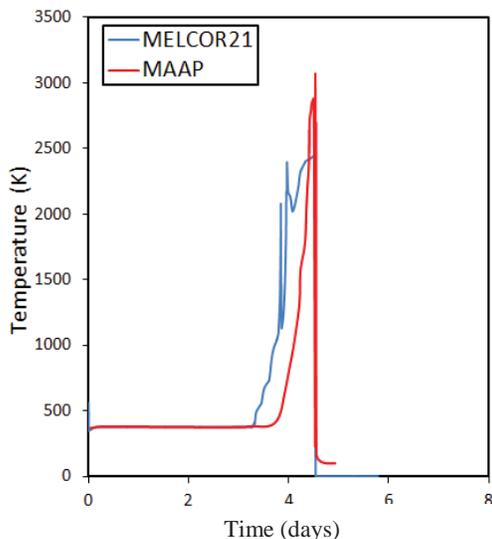
**Figure 21. Peak cladding temperature of spent fuel pool**
