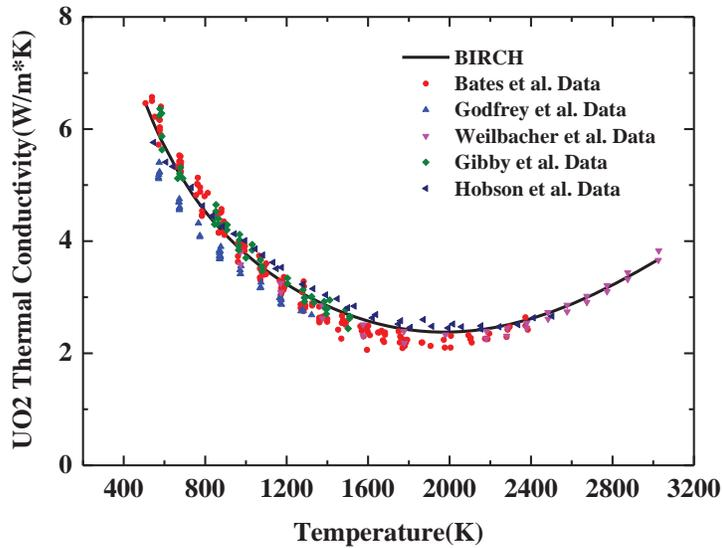
Figure 7 The Comparison of UO<sub>2</sub> Thermal Conductivity and Experimental Data
