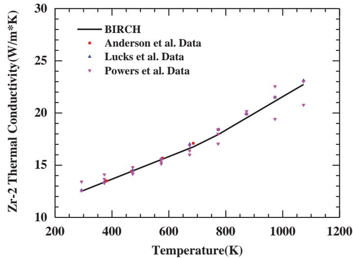
Figure 9 The Comparison of Zr-2 Thermal Conductivity and Experimental Data
