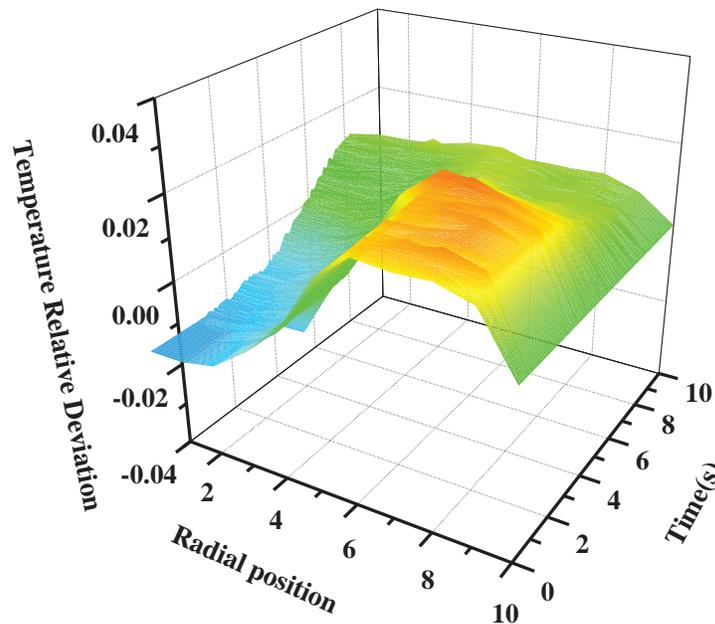
Figure 11 Pellet temperature relative deviation between FACTRAN and BIRCH
