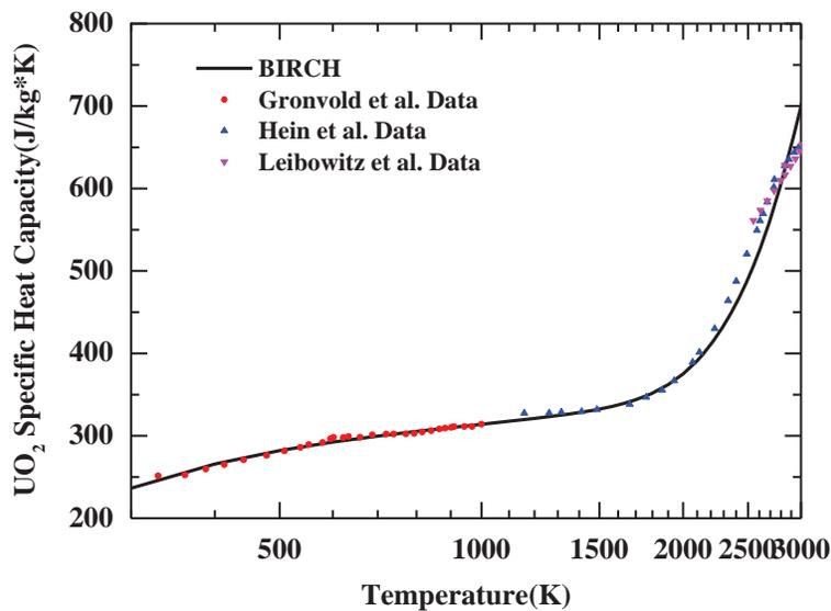
Figure 8 The Comparison of UO<sub>2</sub> Specific Heat Capacity and Experimental Data
