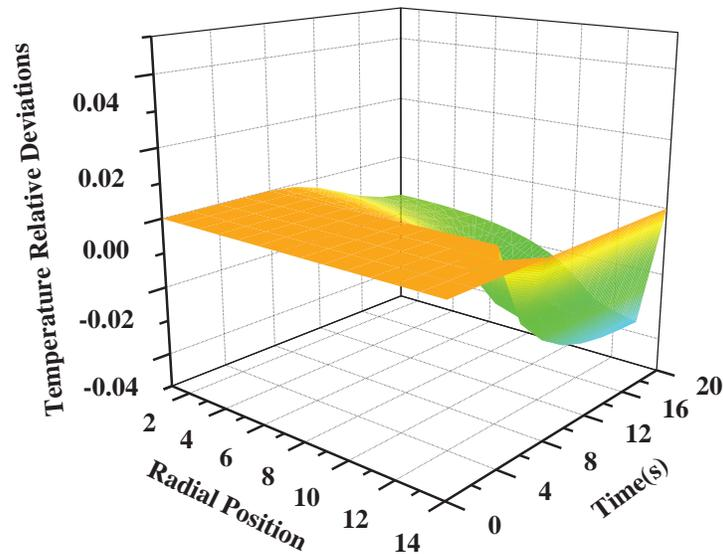
Figure 4 Temperature Relative Deviations of Unsteady-State Heat Conduction Test
