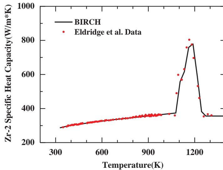
Figure 10 The Comparison of Zr-2 Specific Heat Capacity and Experimental Data
