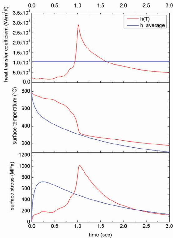
**Figure 3.** (a) comparisons of heat transfer coefficient, surface temperature (calculated), and surface stress (calculated) with surface temperature dependent heat transfer coefficient  $h(T_s)$  [31] and with the average heat transfer coefficient  $h(T_s)_{avg}$  for 5mm thick  $Al_2O_3$  of 800°C quenched into 20°C water bath.
