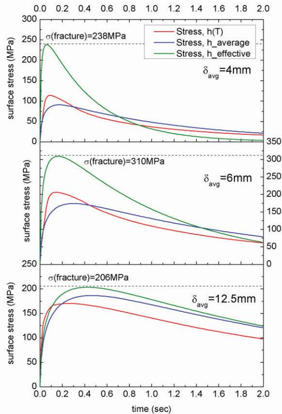
**Figure 4.** Surface stress evolution with different inputs of heat transfer coefficients ( $h(T_s)$  [31],  $h(T_s)_{\text{avg}}$ , and  $h_{\text{eff}}$ ) for increasing material thicknesses of  $\text{Al}_2\text{O}_3$  quenched from the critical temperatures for thermal shock fracture.  $h_{\text{eff}}$  were calculated from Eq.(1) with inputs from experiments ( $\text{Al}_2\text{O}_3$  experimental data: 4mm [5], 6mm [10], and 12.5mm [13]).
