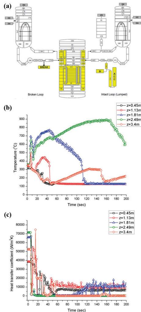
**Figure 6.** RELAP-5 3D results for the reference LBLOCA: (a) RELAP-5 3D LBLOCA nodalization scheme [Figure in courtesy of R. Hu [34]] (b) cladding outer surface temperature and (c) local heat transfer coefficients with respect to axial location  $z$
