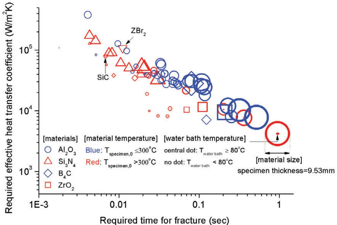
**Figure 1.** Required effective heat transfer coefficients and time for fracture obtained with Eq.(1) and (2), respectively, from various past thermal shock experimental data that provide fracture stress, critical temperature difference, water bath temperature, and specimen size. Presented specimens are selected from past studies [2,4-6,9,10,13,14,19,20-22]
