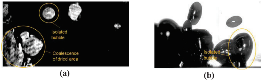
Figure 3. Measurement principle of bubble parameters such as nucleation site density, bubble departure diameter, bubble departure frequency and wait time.
