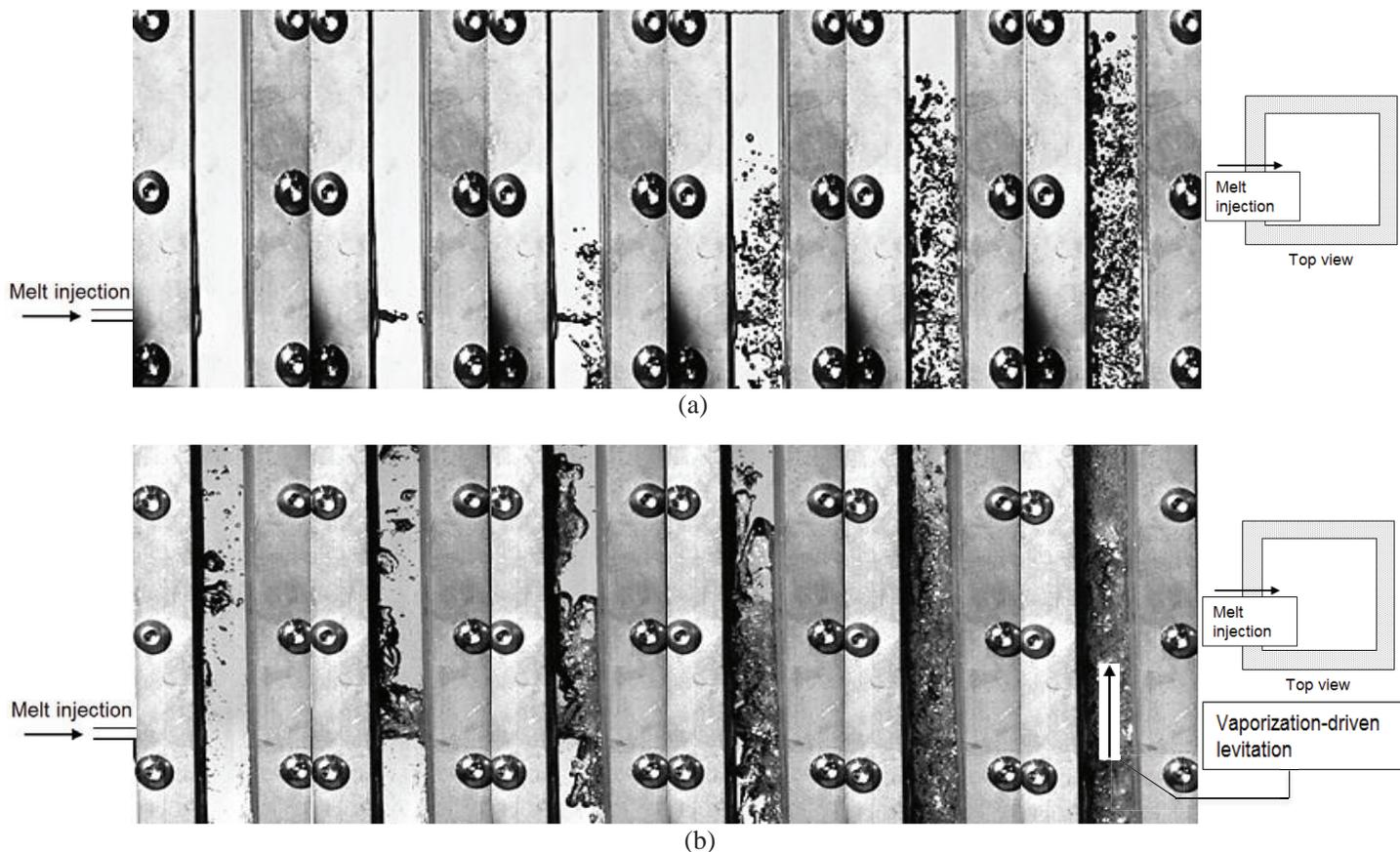
**Figure 3. FCI behavior of melt in (a) unvoided water channel in test 3, and (b) unvoided R123 channel in test 4.**
