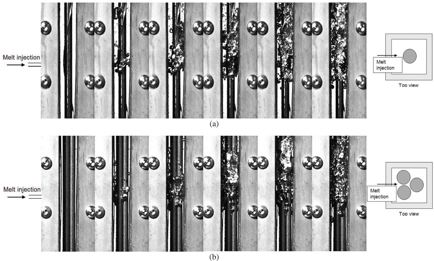
**Figure 2. FCI behavior of melt in (a) single pin-inserted water channel in test 1, and (b) three pins-inserted water channel in test 2.**
