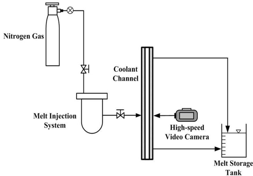
**Figure 1. Schematic of experimental apparatus.**
