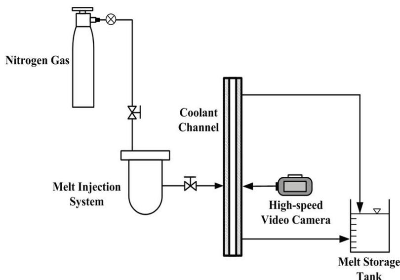
**Figure 1. Schematic of experimental apparatus.**
