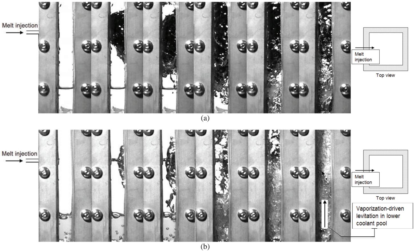
**Figure 4. Melt behavior in (a) air voided water channel in test 5, and (b) air voided R123 channel in test 6.**
