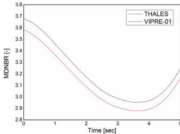
**Figure 6. Comparison of MDNBR profiles of hot channel between THALES and VIPRE-01 for total loss of reactor coolant flow.**
