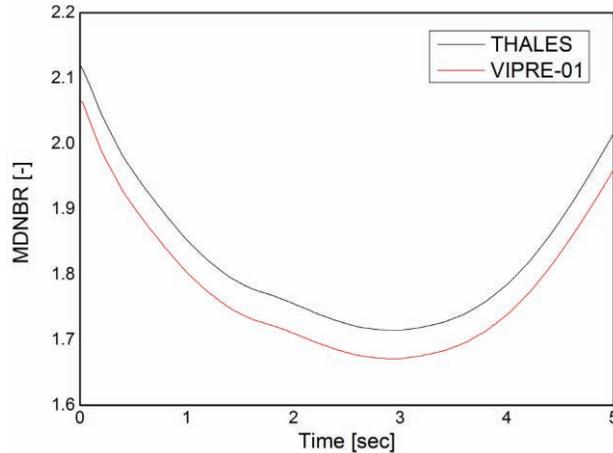
**Figure 8. Comparison of MDNBR profiles of hot channel between THALES and VIPRE-01 for RCP rotor seizure with loss of offsite power.**
