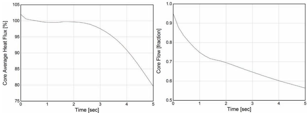
**Figure 7. Thermal-hydraulic profiles of hot channel for RCP rotor seizure with loss of offsite power.**
