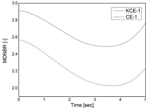
Figure 9. MDNBR profiles of hot channel for total loss of reactor coolant flow by CHF correlations.
