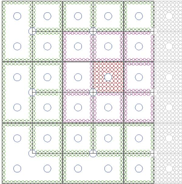
Figure 2. Configuration of subchannels and nodes using THALES single-stage model.
