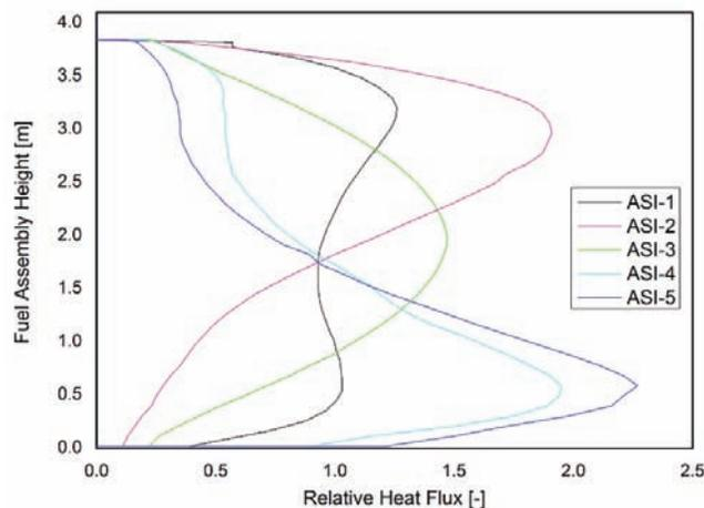
Figure 10. Several types of ASI used in the thermal-hydraulic design for subchannel analysis.
