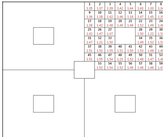
**Figure 1. Typical Rod radial power factors in hot assembly quadrant for DNB analysis in Shinkori 3&4 and its application using THALES single-stage model.**
