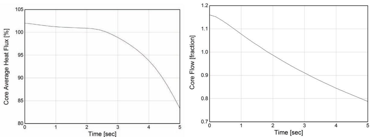
**Figure 5. Thermal-hydraulic profiles of hot channel for total loss of reactor coolant flow.**
