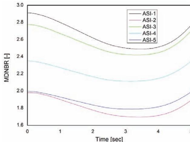
**Figure 11. MDNBR profiles of hot channel for total loss of reactor coolant flow by ASI types.**
