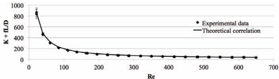
**Figure 11. Friction number correlation for the CIET 1.0 annular heater.**
