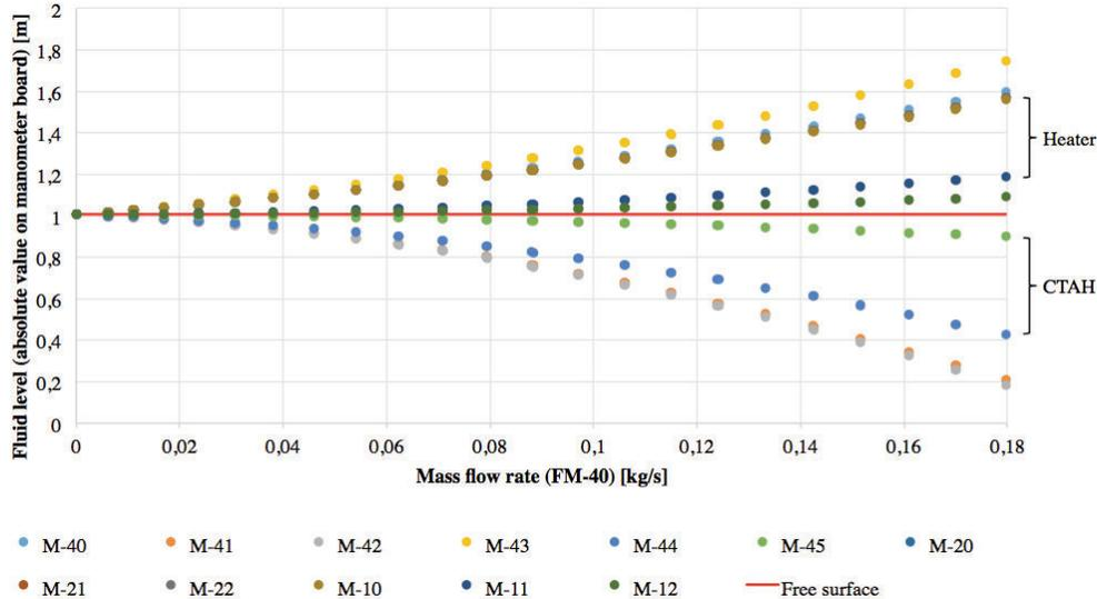
**Figure 10. Fluid levels in the CTAH and heater branches at various flow rates.**
