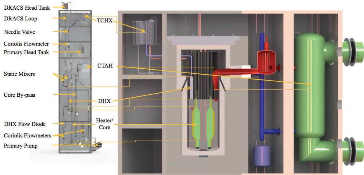
**Figure 3. CIET 1.0 (left) 50% height scaling reasonably matches the Mk1 PB-FHR (right) design.**
