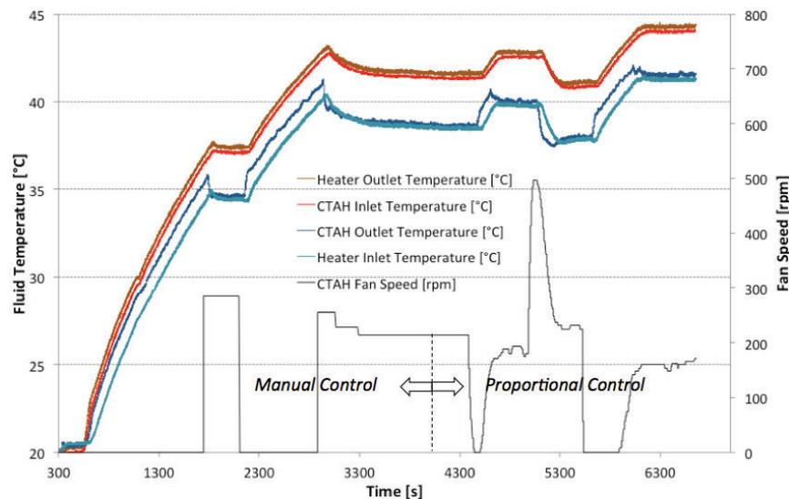
Figure 12. CTAH proportional feedback control test.
