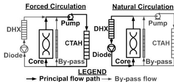
**Figure 1. FHR primary coolant flow paths for forced circulation (left) and natural circulation (right) operational modes [3].**
