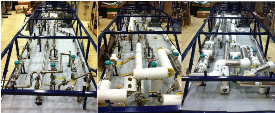
Figure 7. CIET 1.0 piping insulation in progress, February 2014 (left), March 2014 (center) and April 2014 (right).
