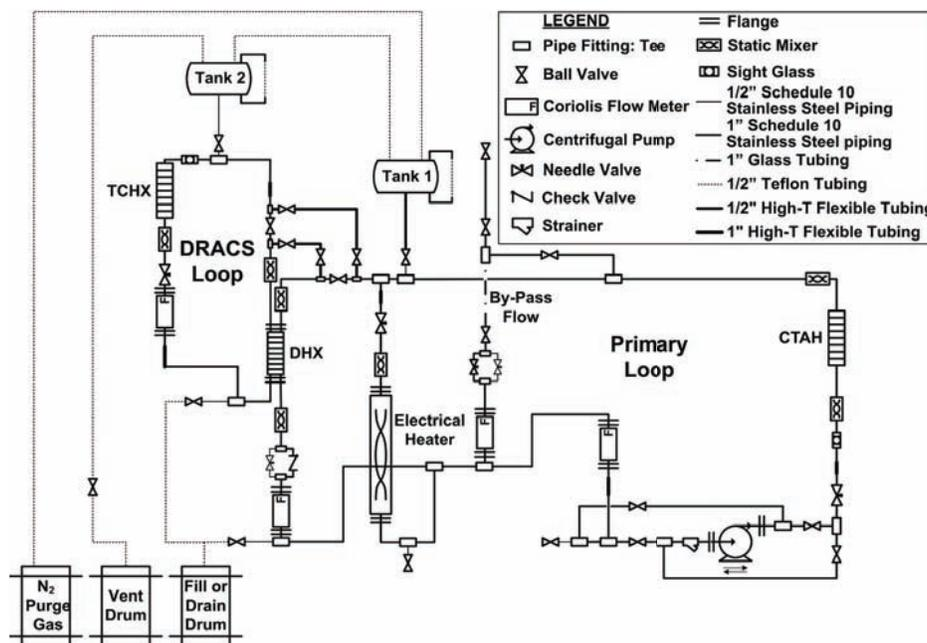
Figure 4. Simplified CIET 1.0 piping and instrumentation diagram [9].
