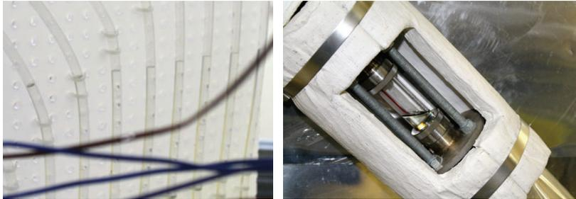
Figure 9. CIET 1.0 transparent sections monitored during fill-up to verify absence of gas bubbles.
