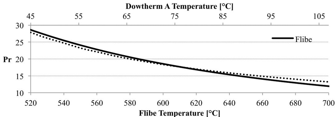
**Figure 2. Impact of temperature on Pr in the prototypical and model systems.**
