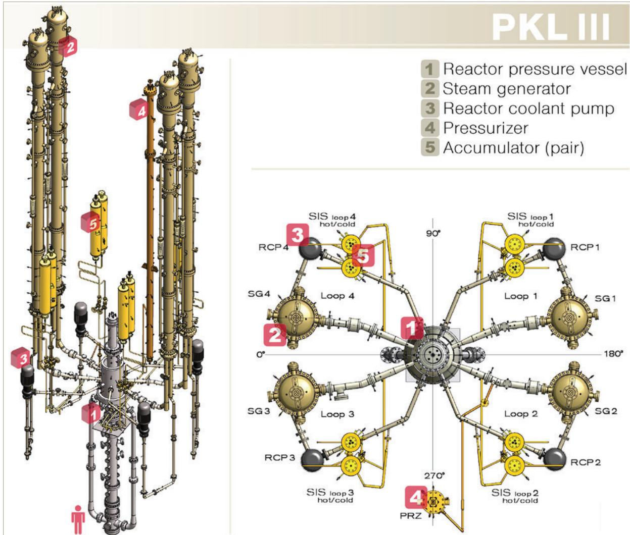
Figure 2. PKL III Test Facility
