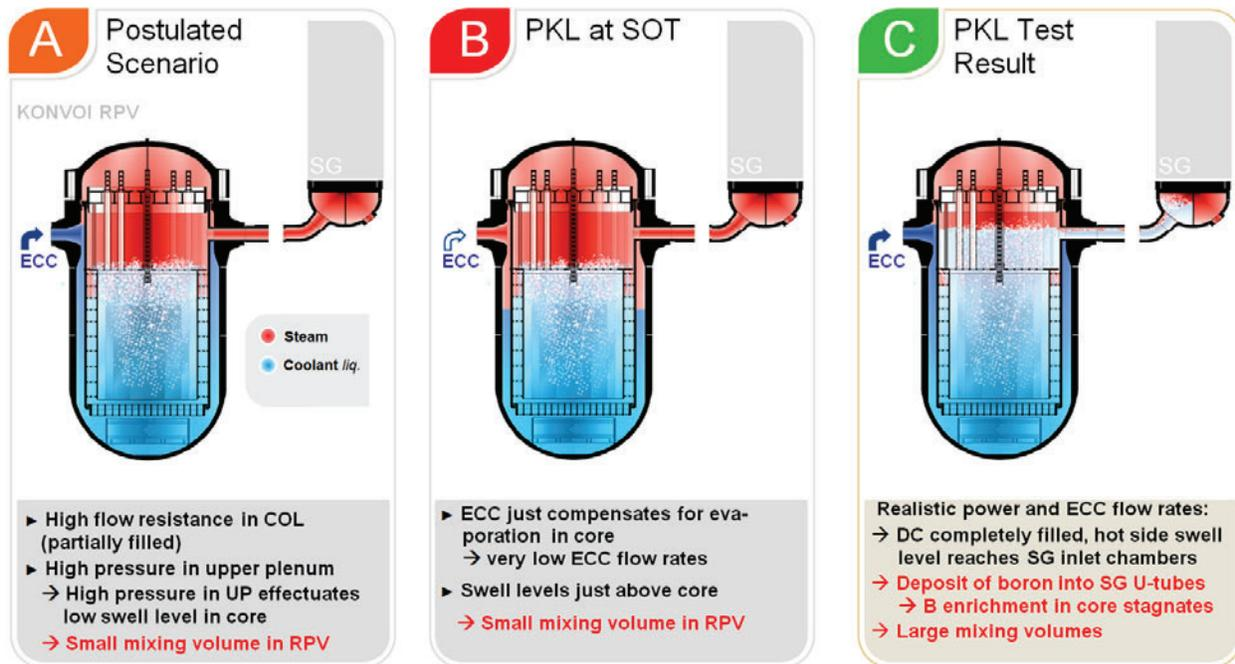
**Figure 6. Postulated Scenario vs. Results for Low Flow Resistances (KONOVI geometry) without the employment of additional butterfly valves in the cross-over legs**
