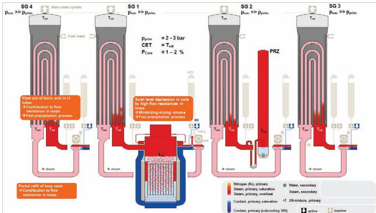
**Figure 1. Postulated Scenario: Long-Term Cooling Phase Following LB-LOCA**
