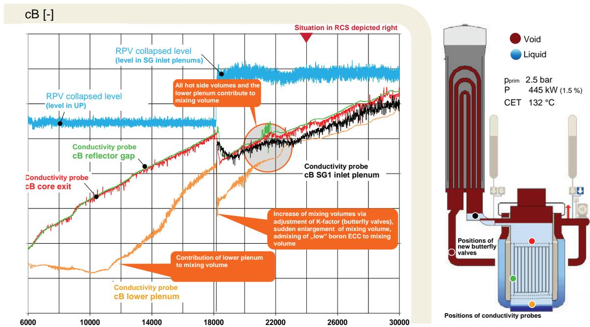
**Figure 4. Increase of cB in RCS Sections During Core Cooling with Two-Phase Mixture.**
