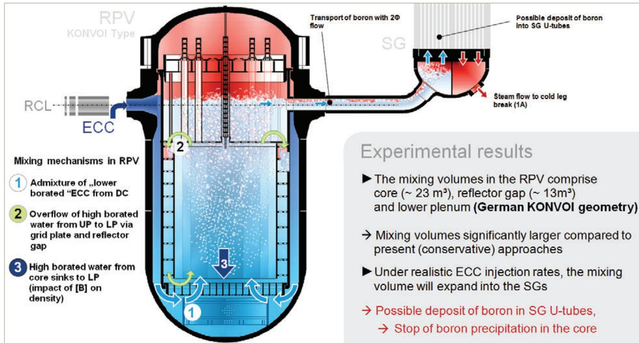
Figure 5. Mechanisms Interconnecting the Hot-Side Volumes (experimental results applied to PWR).
