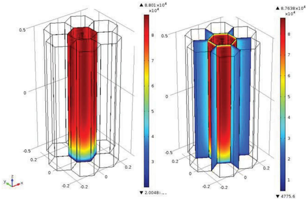
**Figure 9 Surface radiosity ( $W/m^2$ ) (left) and surface irradiation ( $W/m^2$ ) (right).**
