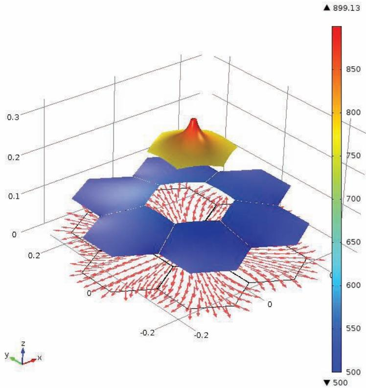
Figure 3 Temperature profile ( $^{\circ}\text{C}$ ) at middle of graphite section ( $z = 0.5\text{m}$ ): Radiation only case, Pressure = 10 bar, Input Power = 16,000 W.
