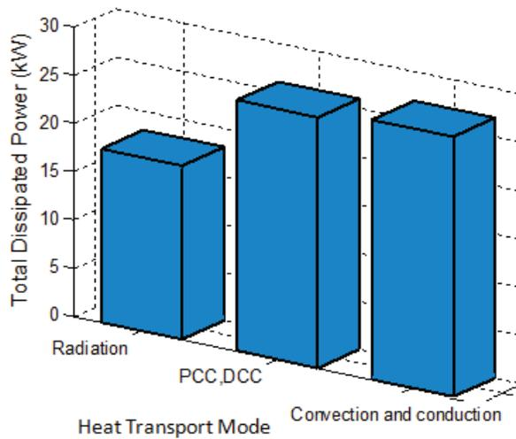
**Figure 5 Heat dissipation rates for different heat transport modes when the maximum graphite temperature is kept at 1,176 K and outer wall temperature at 773 K.**
