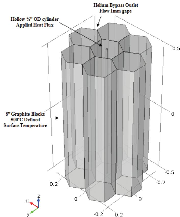
**Figure 1 Physical model consisting of 7 hexagonal prisms and a central prism containing a hollow cylinder with a uniform surface heat flux defined on its inner surface.**
