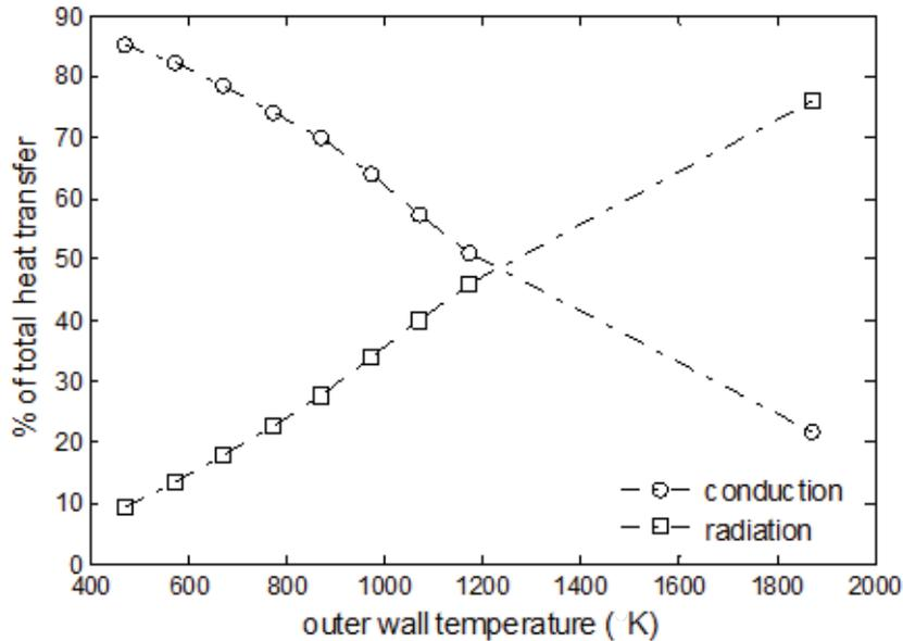
Figure 11 Sensitivity study on outer wall temperature: input power 10kW
