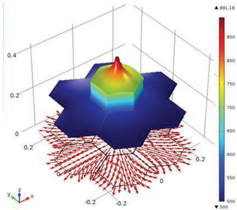
Figure 4 Temperature Profile ( $^{\circ}\text{C}$ ) at middle of graphite section ( $z = 0.5\text{m}$ ): Stagnant gas case, Pressure = 10 bar, Input Power = 26,000W.
