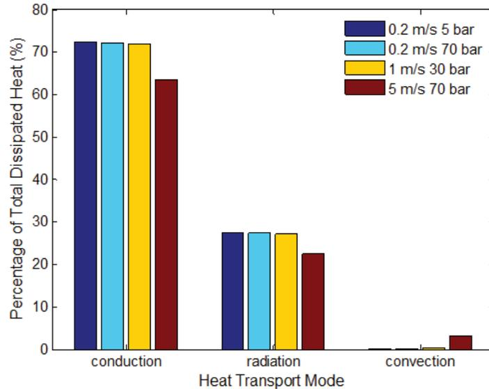
Figure 6 Fractional contributions of individual heat transport modes for various helium flow conditions.
