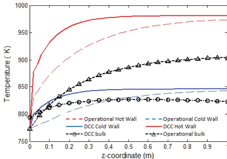
Figure 7 Centerline graphite temperature for DCC conditions (5 bar, 0.2 m/s (solid line)) and operational conditions (70 bar, 5 m/s (dashed line)) for parallel graphite walls; also gas bulk temperatures shown with symbols for both conditions.
