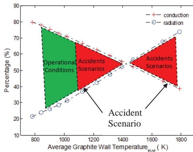
**Figure 10 Conduction and radiative heat transfer contributions in total heat dissipation under PCC conditions as a function of average graphite wall temperature.**
