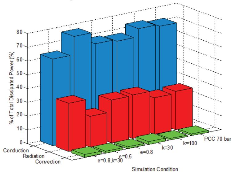
**Figure 8 Fractional contributions of different heat transport modes for various coolant flow conditions.**
