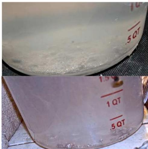
**Figure 2. Fragmentation results from VG and G type spontaneous explosions in 10 w/o aqueous NaCl with 0.3 w/o (top) and 5 w/o (bottom) Al-GaInSn alloys respectively**
