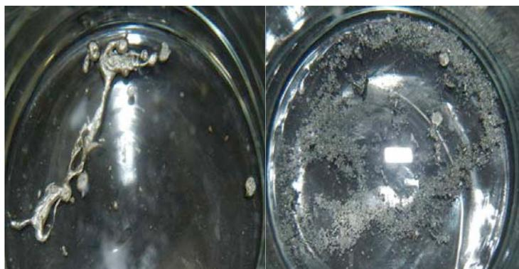
**Figure 4. Fragmentation of Sn melts exposed to variable amplitude shock pulses from detonation of a submerged electrical bridgewire. The left and right photos correspond to capacitor energies of 25 J and 32 J respectively.**
