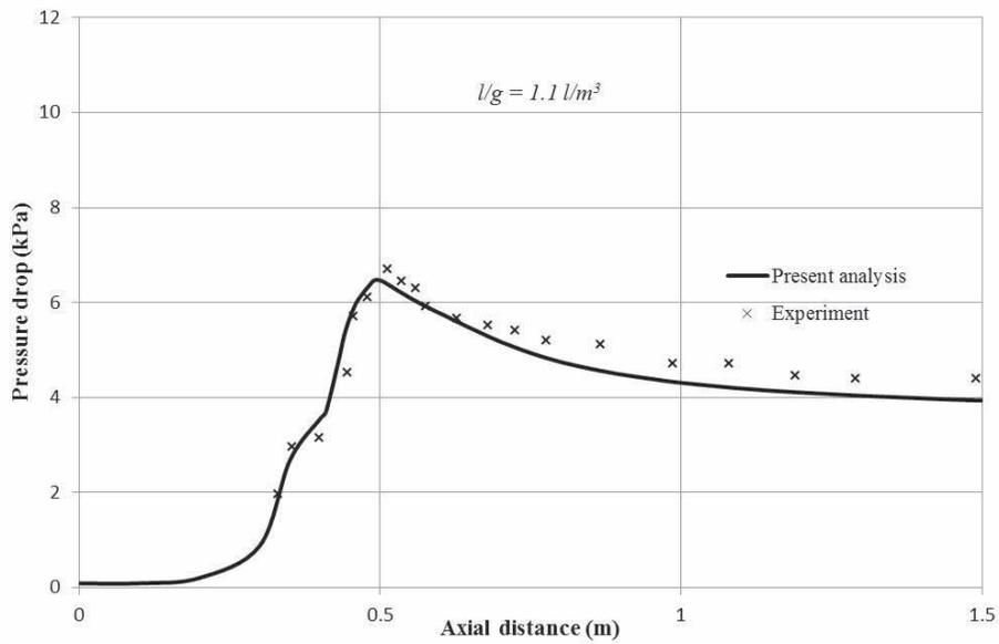
Figure 3. Pressure drop profiles as a function of axial distance when  $V_{g,th}=70 \text{ m/s}$  and  $l/g=1.1 \text{ l/m}^3$
