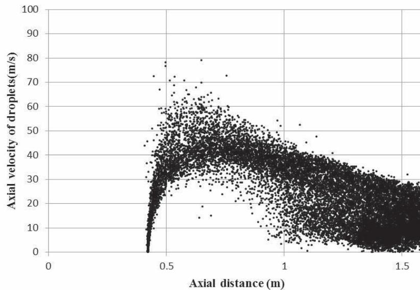
**Figure 4. Droplet axial velocity as a function of axial distance when  $V_{g,th}=70 \text{ m/s}$  and  $l/g=1.1 \text{ l/m}^3$**
