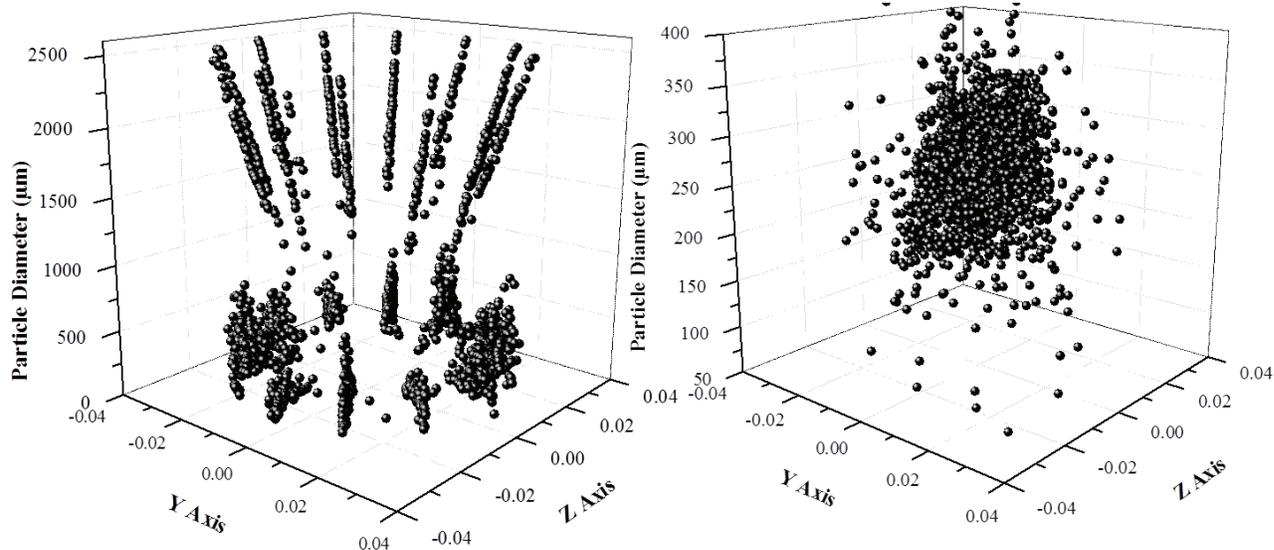
**Fig 5. Droplet diameter distribution just after injection( $x=0.423$ ) (left) and at the throat end( $x=0.493m$ ) (right).**
