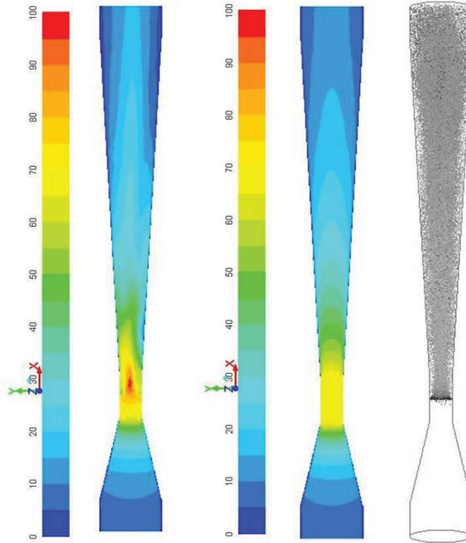
Figure 2. Contours of (a) gas only flow velocity (b) three phase gas velocity for  $l/g=1.1$ ; (c) Droplet distribution for  $l/g=1.1 \text{ l/m}^3$
