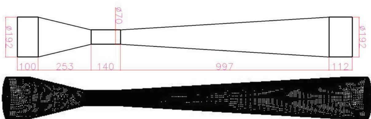
Fig 1: Geometry and computational mesh of circular Venturi scrubber (unit:mm)
