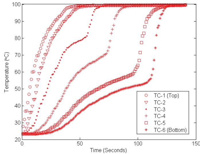
**Figure 5. Thermocouple responses for slow injection experimental run.**
