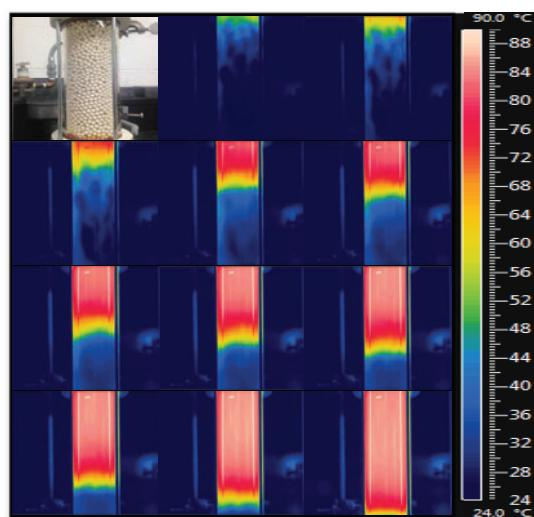
**Figure 4. (TOP LEFT)** Picture of experimental packed bed vessel. **(THE REST)** Time step images from FLIR software for an experimental run at 50 psi for; 5, 10, 15, 20, 30, 35, 40, 45, 50, 60, 70 seconds after steam injection, respectively.
