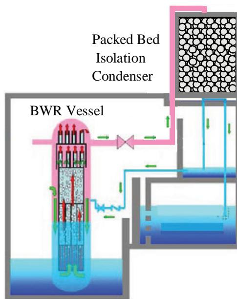
**Figure 2. Schematic of alumina packed bed isolation condenser for a BWR.**
