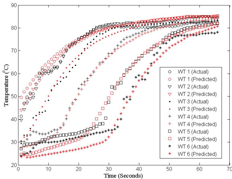
**Figure 11. The comparison of actual and estimated wall temperatures for the second experiment using the polynomial model found from the first experiment.**
