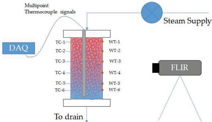
**Figure 3. Schematic of experimental setup of packed bed heat sink consisting of a clear fused quartz tube, alumina particles, multi-point thermocouple, steel piping, steam supply, and FLIR camera.**
