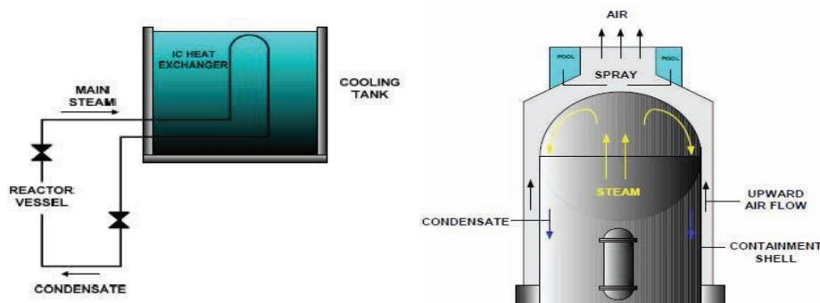
**Figure 1. Schematic of isolation condenser for a BWR (left) and passive safety spray system and natural cooling draft air system (right) [7].**
