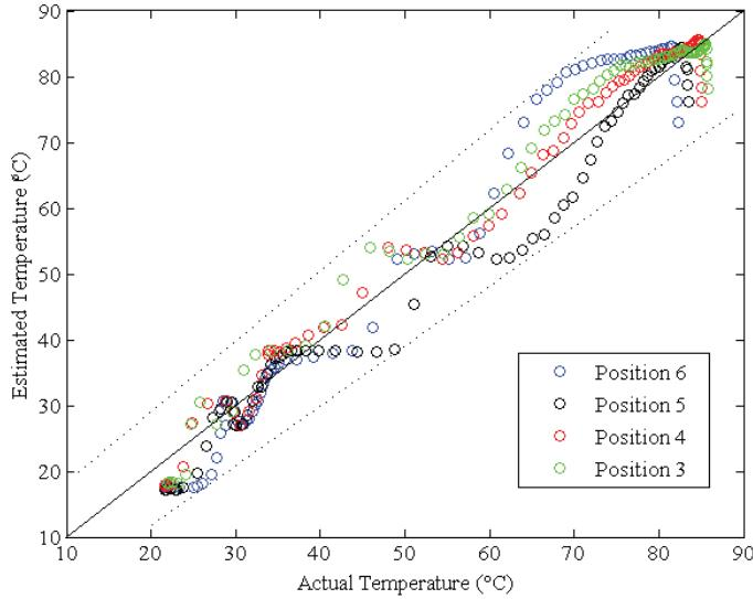
**Figure 9. Actual wall temperature to estimated wall temperature for different positions using polynomial found for position 1.**
