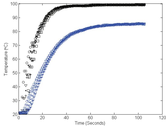
**Figure 8. Thermocouple and wall temperature (Blue) responses for fast injection experimental run.**
