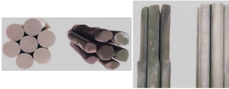
Figure 14. Top and side views of two assemblies of graphite test pieces demonstrating the effects of oxidation.
