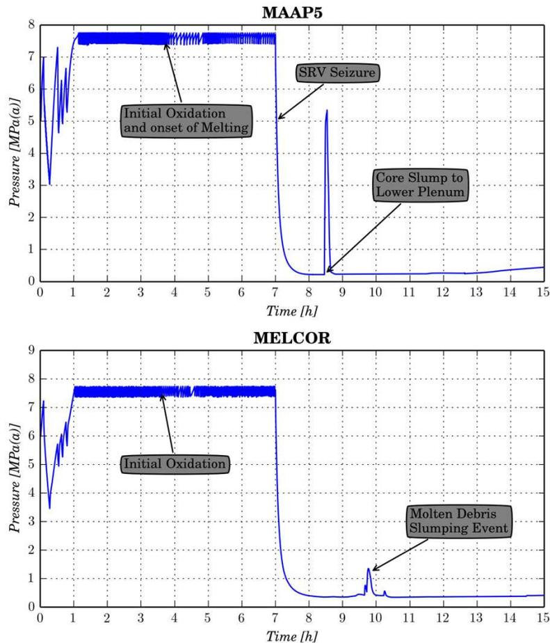
**Figure 1. Comparison of RPV Pressure Transient Simulations**
