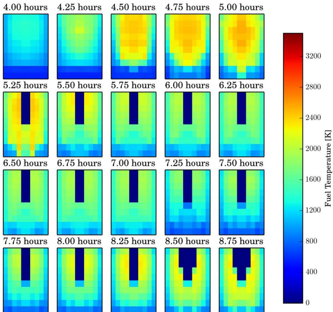
**Figure 4. Distribution of Active Fuel Region Fuel Temperatures at different times in MELCOR Simulation**
