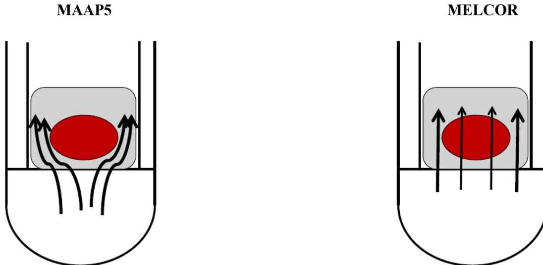
**Figure 9. Illustration of Different Flow Geometries through a Degraded Reactor Core**
