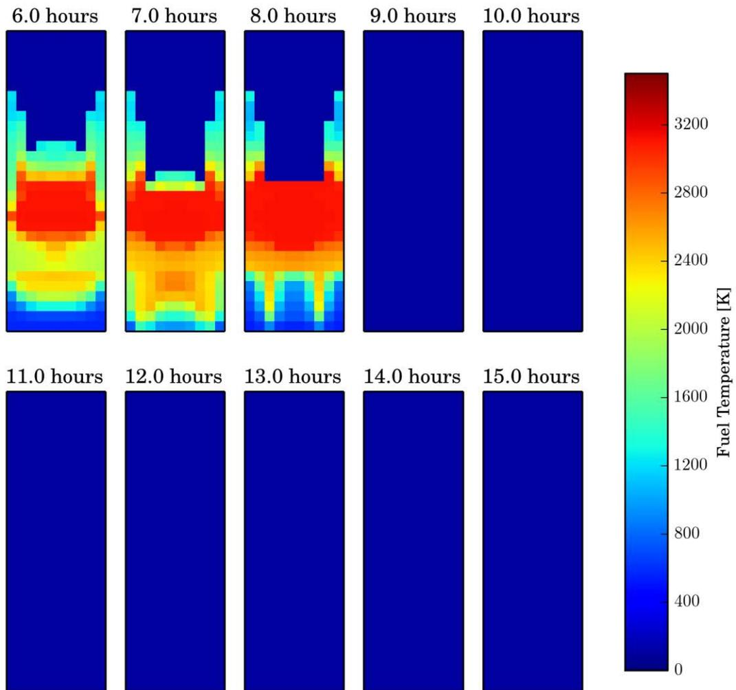
**Figure 5. Distribution of Active Fuel Region Fuel Temperatures to End of MAAP5 Simulation**
