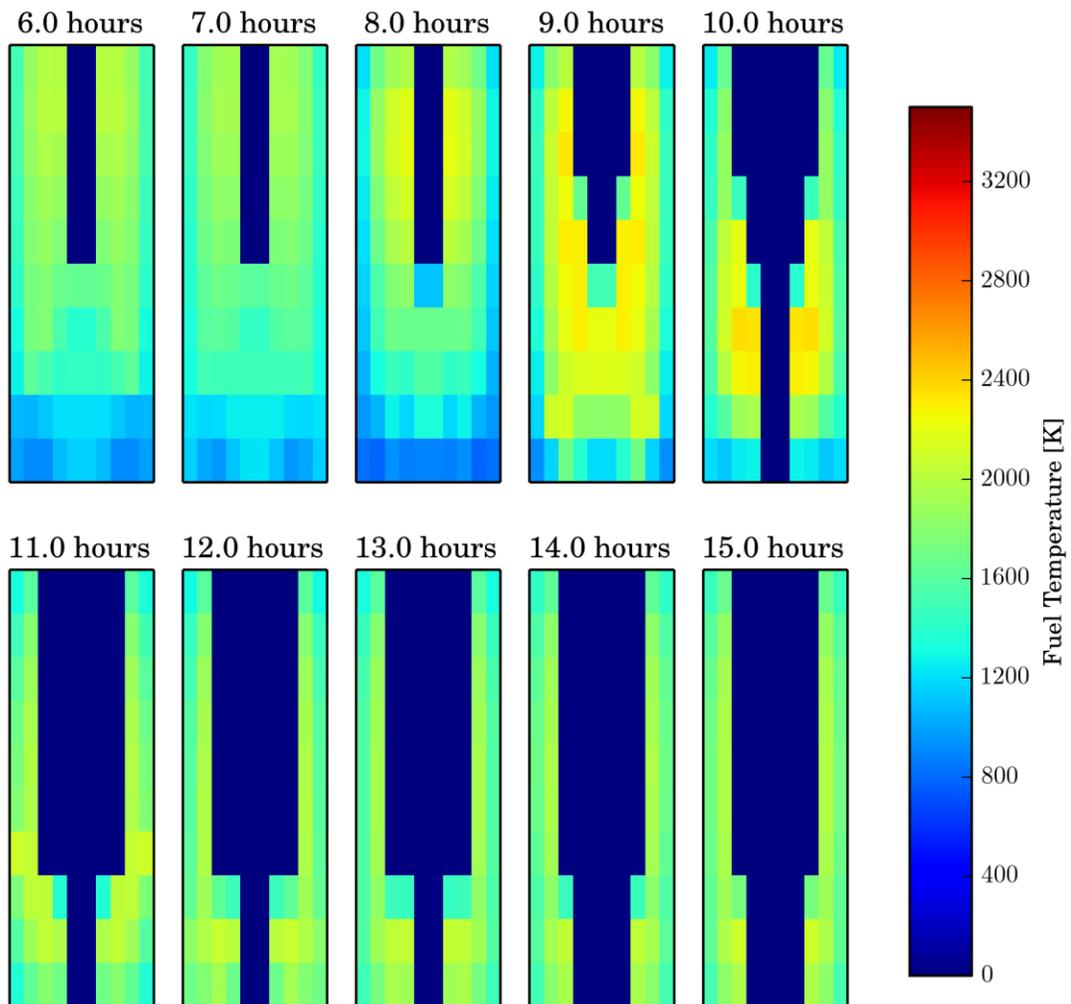
**Figure 6. Distribution of Active Fuel Region Fuel Temperatures to End of MELCOR Simulation**
