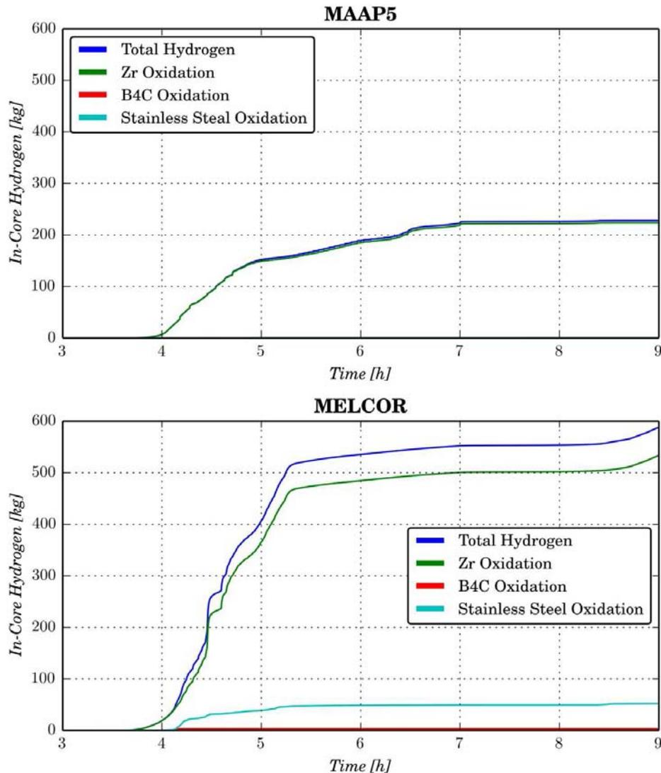
**Figure 8. Comparison of In-Vessel Hydrogen Generation Transient**
