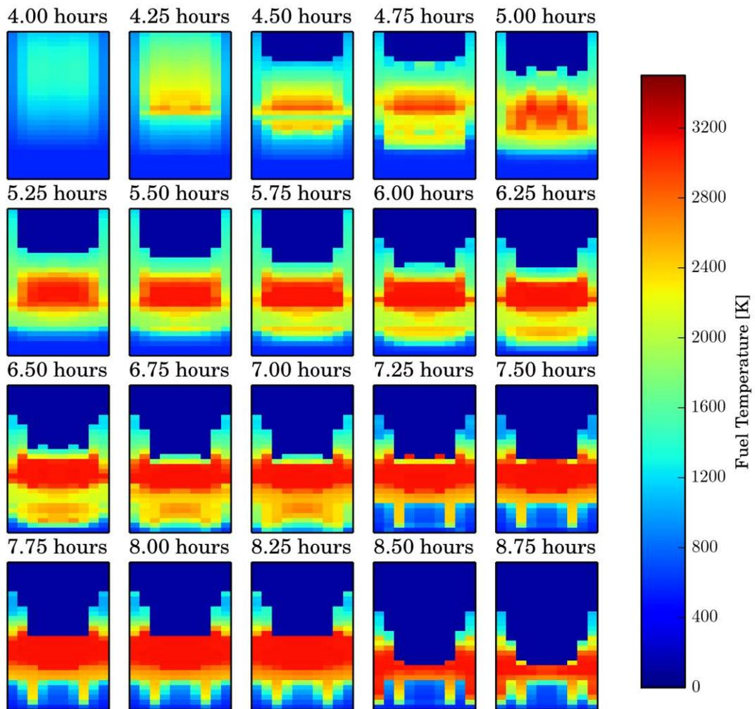
**Figure 3. Distribution of Active Fuel Region Fuel Temperatures at different times in MAAP5 Simulation**
