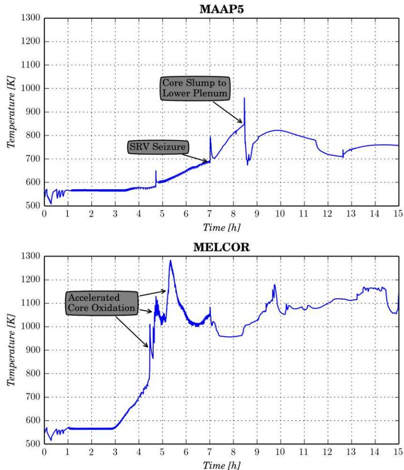
**Figure 7. Comparison of RPV Steam Dome Temperature Transient Simulations**
