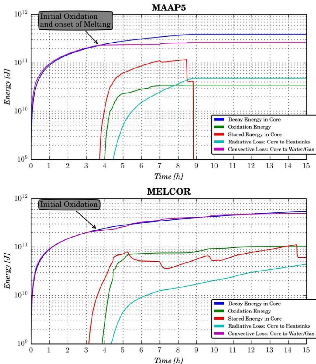
Figure 2. MAAP5 and MELCOR Simulation of Decay and Chemical Heat Transport from Core/Core Debris
