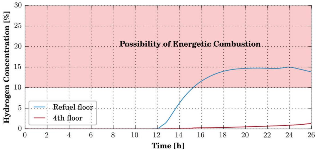
**Figure 5. MAAP5 Unit 1 Simulation of Hydrogen Build-up in Reactor Building**
