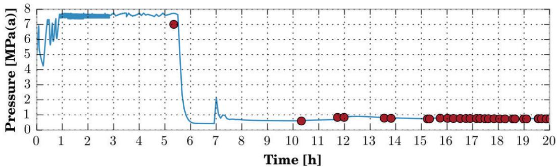
Figure 1. MAAP5 Simulation of Unit 1 RPV Pressure Transient
