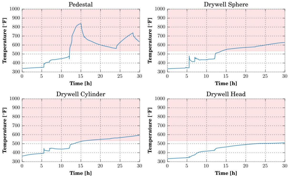
Figure 4. MAAP5 Unit 1 Simulated Drywell Temperature Distribution
