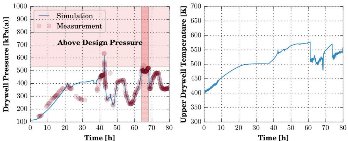
Figure 12. MAAP5 Unit 3 Simulation of Drywell Response
