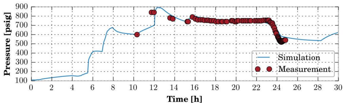
**Figure 3. MAAP5 Simulation of Unit 1 Containment Pressure Transient**
