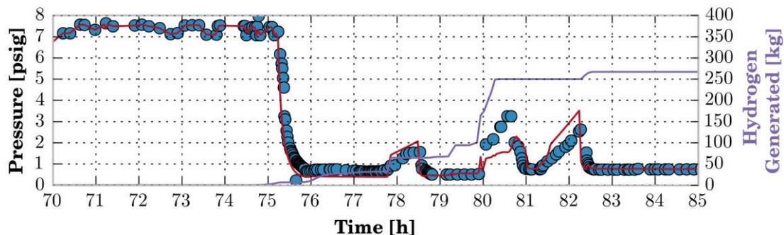
**Figure 8. MAAP5 Unit 2 Simulation of Late-Phase RPV Pressure Transient**
