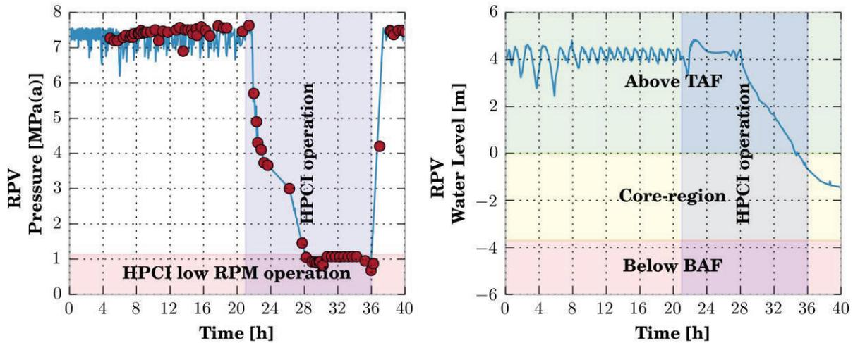
Figure 11. MAAP5 Unit 3 Simulation of Reactor Response
