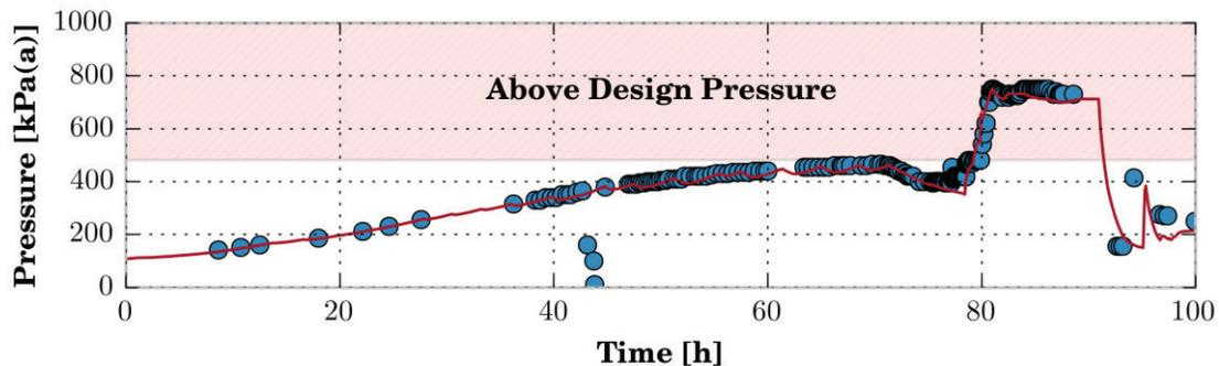
Figure 9. MAAP5 Unit 2 Simulation of Containment Pressure Transient
