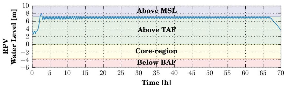
**Figure 6. MAAP5 Unit 2 Simulation of RPV Water Level**
