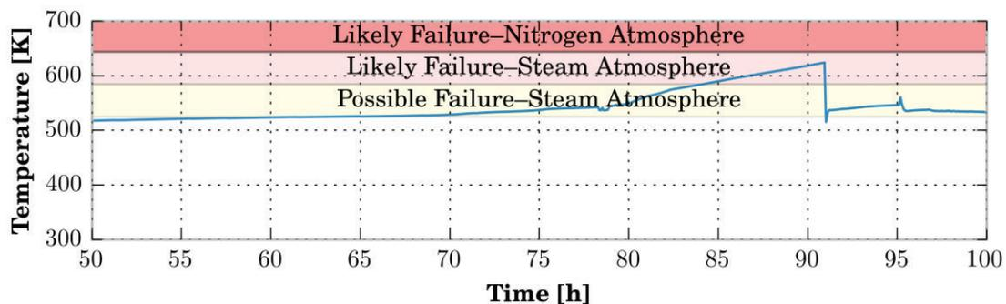
Figure 10. MAAP5 Unit 2 Simulation of Upper Drywell Temperature Transient
