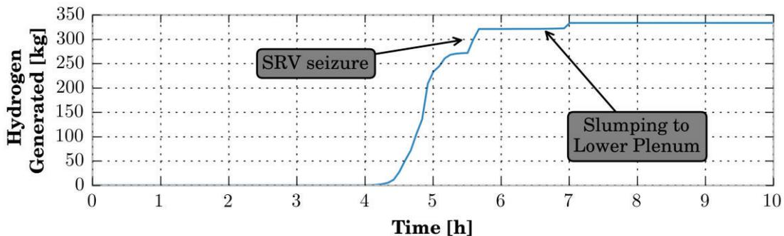
Figure 2. MAAP5 Unit 1 Simulation of In-Vessel Hydrogen Generation
