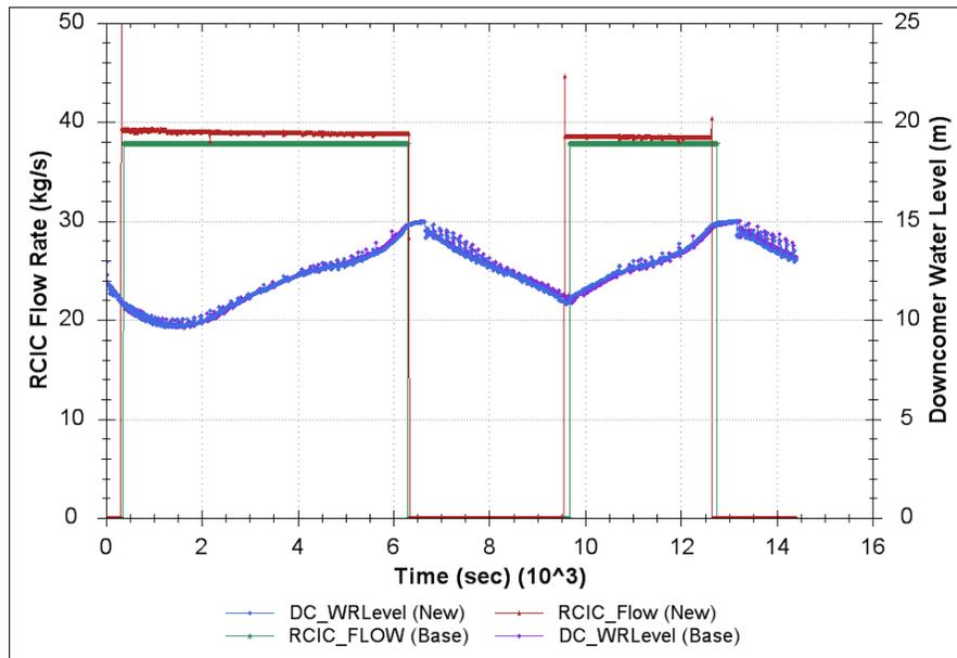
**Figure 9. Case 1 RCIC Flow and RPV Level**
