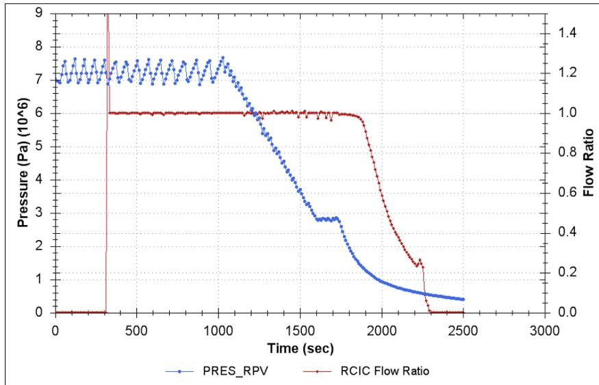
**Figure 11. Case 3 RPV Pressure and RCIC Flow**
