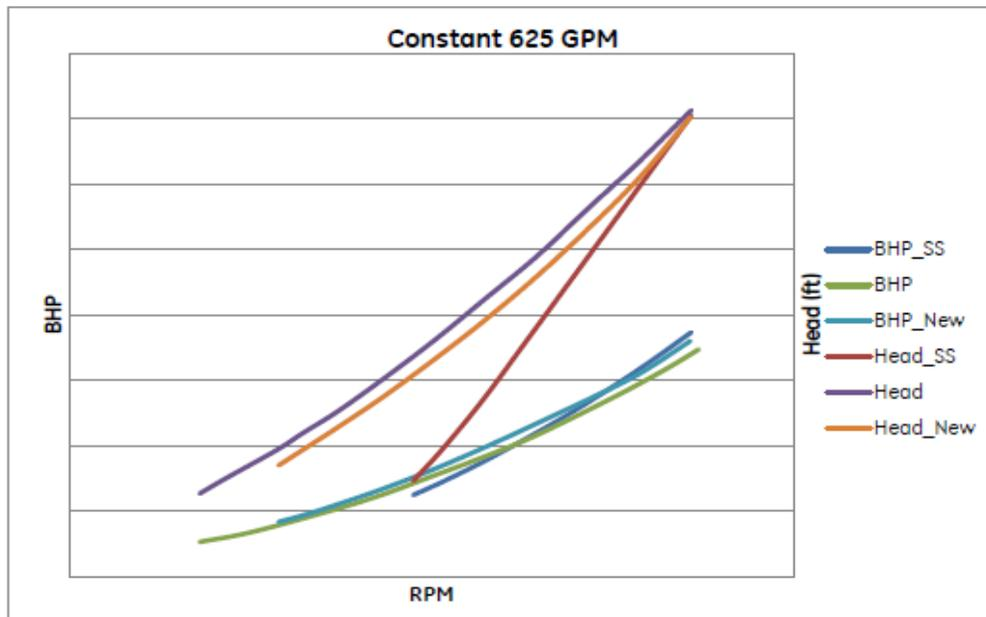
**Figure 4. RCIC Pump Behavior at Constant Flow**
