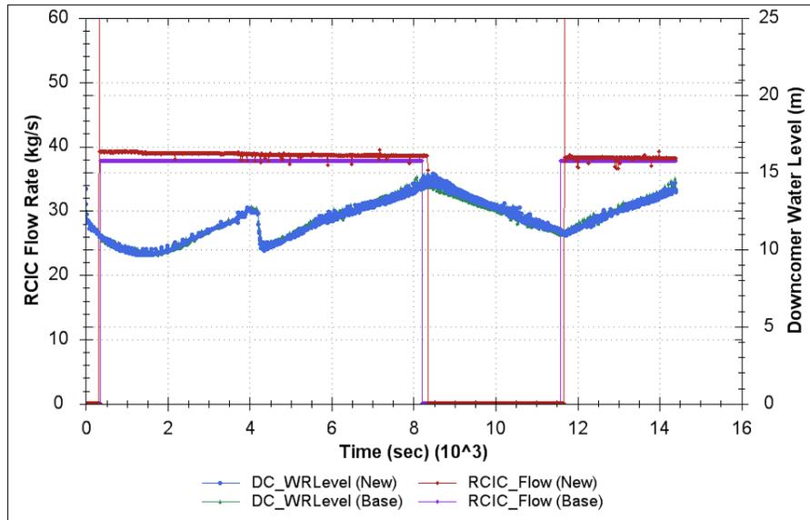
**Figure 10. Case 2 RCIC Flow and RPV Level**
