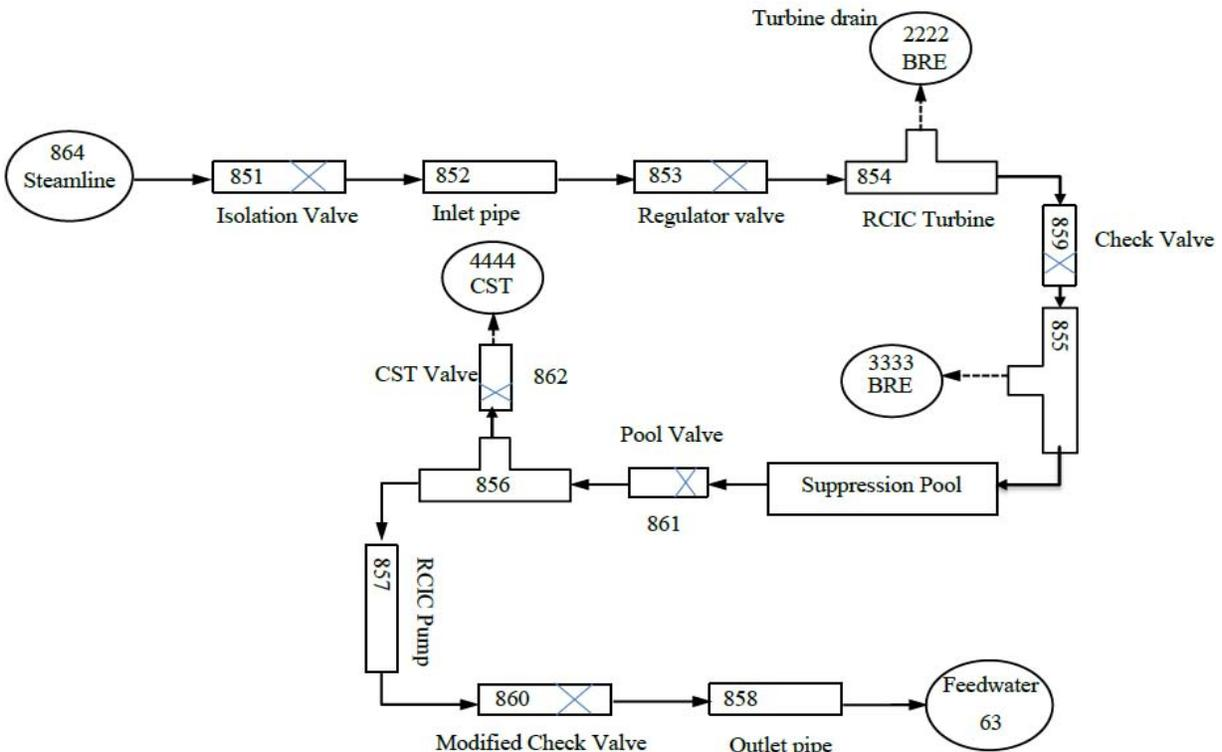
Figure 2. TRACG RCIC Component Model
