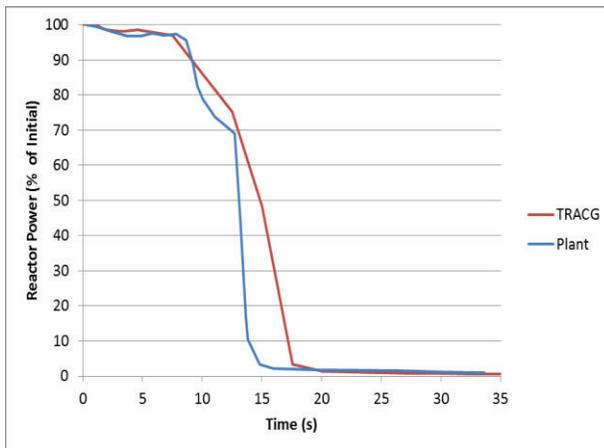
**Figure 3. Reactor Power**
