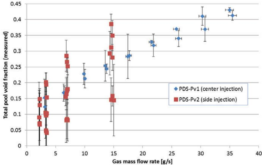
**Figure 3: Measured total void fraction in the pool for tests without particles (two-phase flow). The measurement error of the gas flow rate does not exceeds 2% (horizontal error bars are not shown).**
