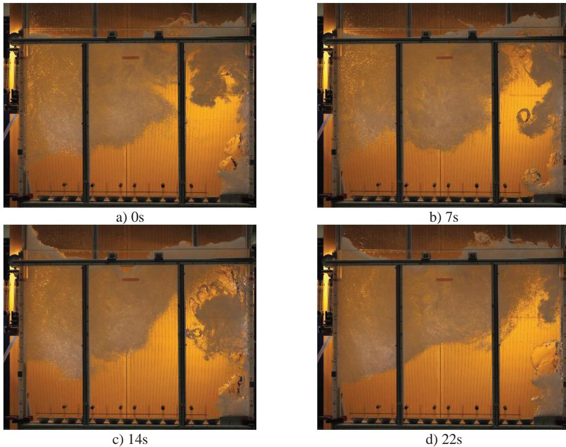
Figure 6: Snapshots of the particles-free test NOPs-28 with highest air flow rate of 15 g/s,  $H_{pool} = 0.9$  m pool depth and  $L_{pool} = 1.6$  m pool length. The relative to image (a) time offset in seconds of each snapshot is indicated below each subfigure.
