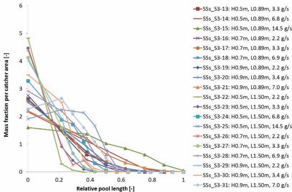
Figure 7: Spatial particle mass distribution from tests performed with 3 mm stainless steel particles.
