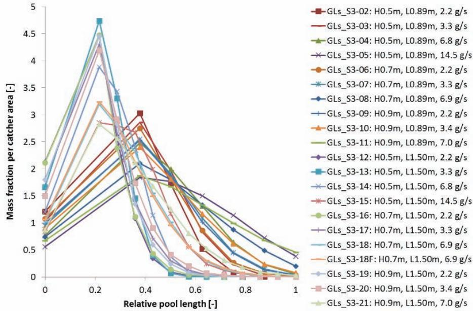
Figure 8: Spatial particle mass distribution from tests performed with 3 mm glass particles.
