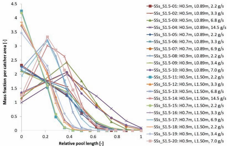
Figure 9: Spatial particle mass distribution from tests performed with 1.5 mm stainless steel particles.
