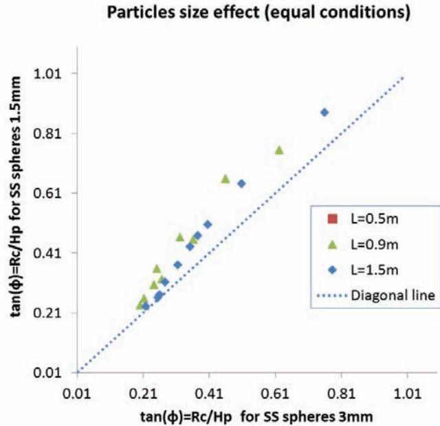
**Figure 12: Particle size effect: comparison of the average spreading angle of the corresponding experiments performed at equal test conditions except for the size of the particles (1.5 mm vs 3 mm).**
