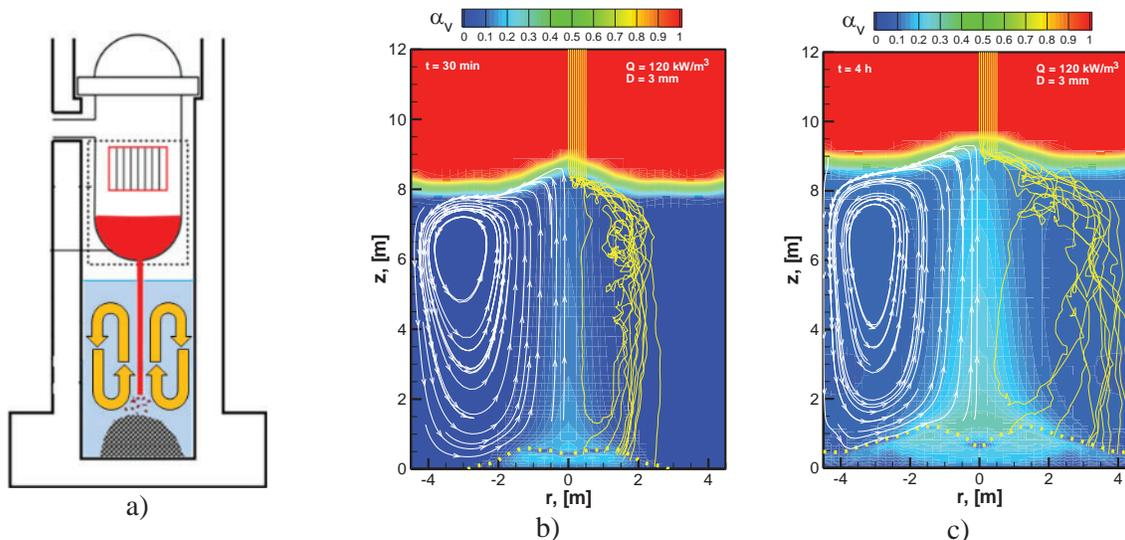
**Figure 1: Illustration of the large turbulent currents during corium debris release in RV cavity under SA conditions (a) and simulation of particle trajectories affected by the circulation in the saturated pool at 30 min (b) and 4h (c), after [2]. See explanation in the text.**
