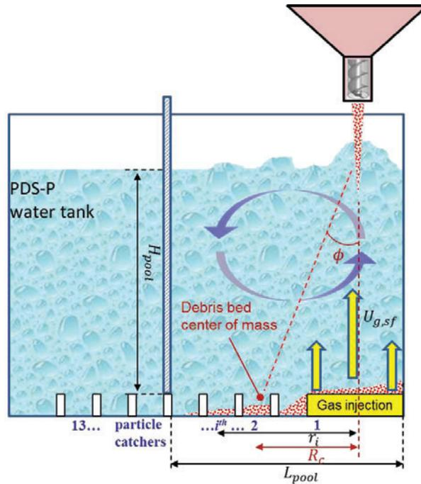
Figure 10: Schematics of the particle spreading in the PDS-P pool with defined characteristic spreading angle  $\phi = \tan^{-1} \frac{R_c}{H_{pool}}$  depending on center of mass  $R_c$  (or average spreading distance  $R_{spr}$ ) and pool depth  $H_{pool}$ .
