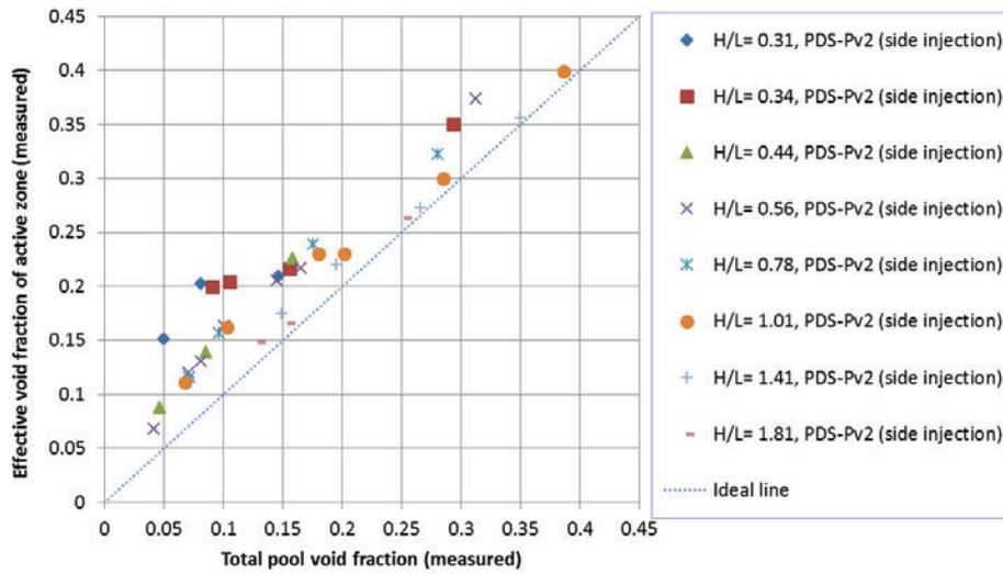
Figure 5: Comparison of the measured total vs effective void fractions in the pool.
