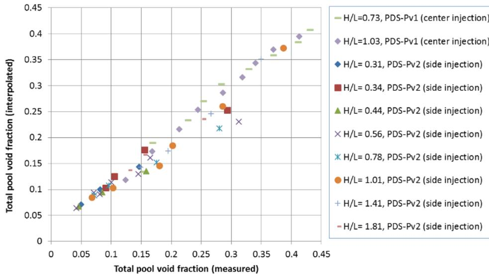
**Figure 4: Interpolated void fraction versus experimentally measured values. Short notation  $H/L$  in the legend is the ratio of the pool depth to its length  $H_{pool}/L_{pool}$ .**
