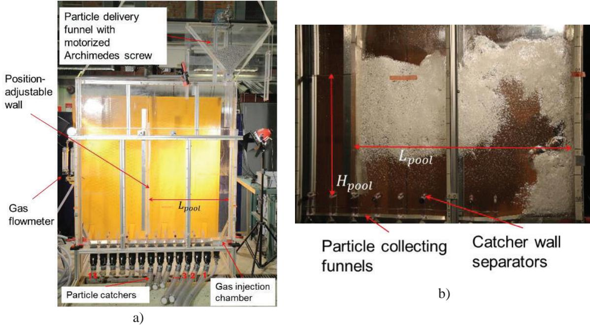
**Figure 2: PDS-P facility: general view (a) and test section in operation (b). The pool depth  $H_{pool}$  (b) is measured from the upper tip of the walls separating particles catchers.**
