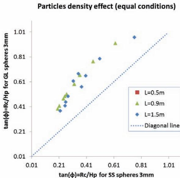
Figure 11: Particle density effect: comparison of the average spreading angle of the corresponding experiments performed at equal test conditions except for the density of the particles (glass vs stainless steel).
