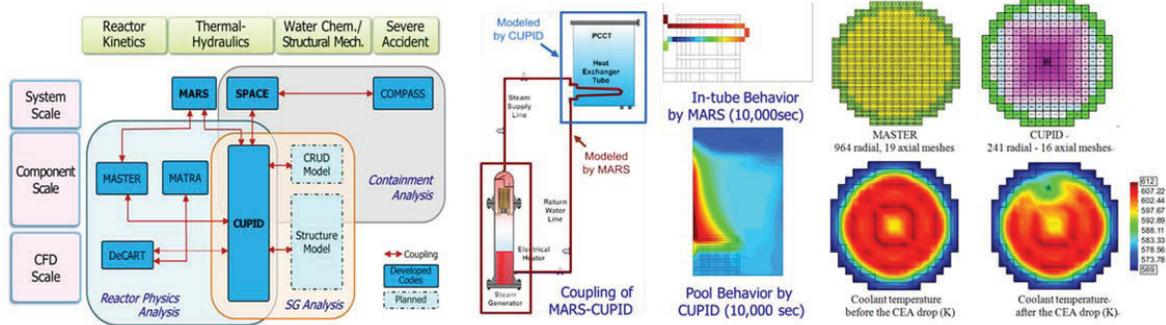
(a) Coupled System of Codes (b) Coupling of MARS-CUPID (c) Coupling of MASTER-CUPID
