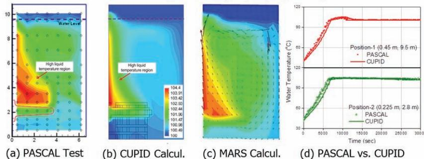
**Fig. 16 Thermal Mixing in a PCCT Pool: PASCAL Experiment vs. CUPID Calculation**
