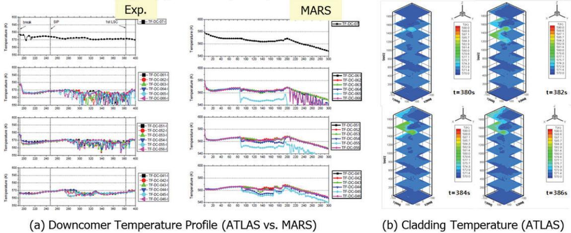
(a) Downcomer Temperature Profile (ATLAS vs. MARS) (b) Cladding Temperature (ATLAS)
