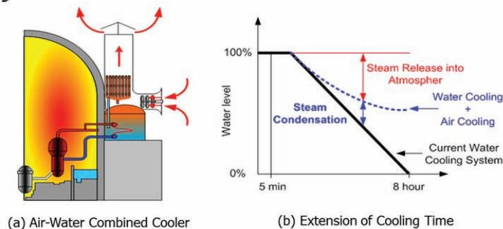
**Fig. 2 A Combined Cooling Concept for Coping with Prolonged SBO Condition**
