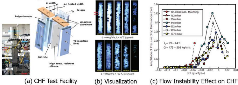
Fig. 4 Boiling Heat Transfer for Downward Flow in a Narrow Rectangular Channel
