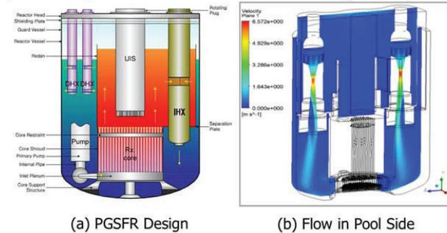
Fig. 6 PGSFR Design and CFD Analysis of Flow Behavior in a Pool
