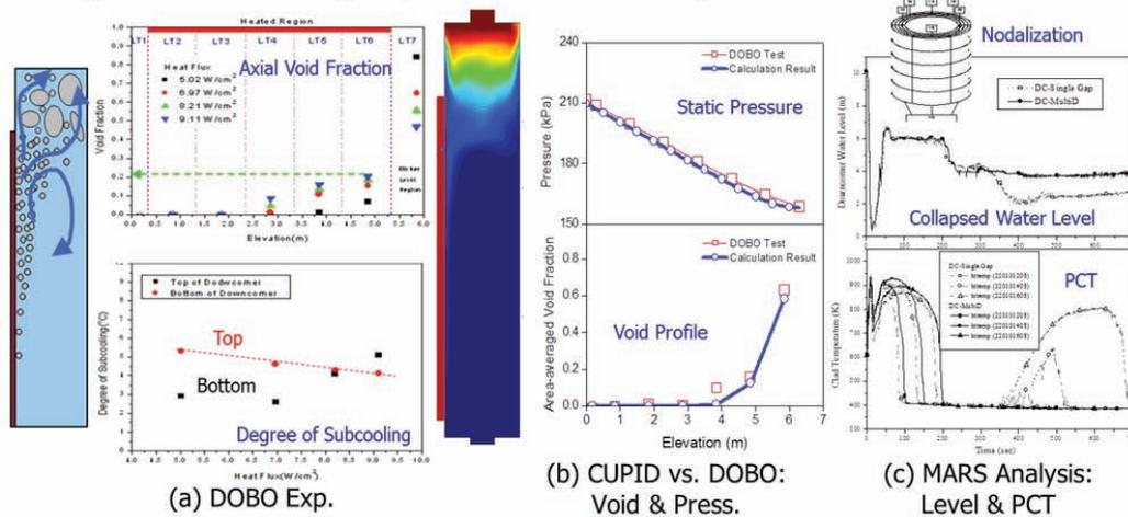
**Fig. 14 Subcooled Boiling Revealing Multi-dimensional Behavior in a RV Downcomer**
