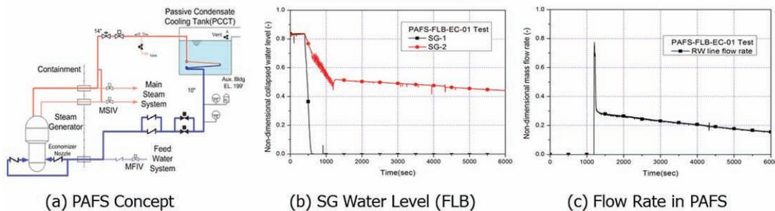
Fig. 1 PAFS Concept and its Actuation during a FLB Accident
