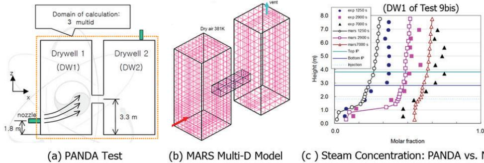
**Fig. 17 Mixing in a Containment: Comparison of PANDA Test with MARS Analysis**
