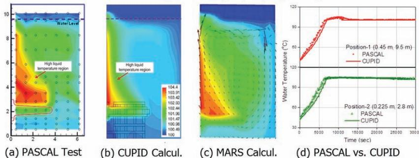
**Fig. 16 Thermal Mixing in a PCCT Pool: PASCAL Experiment vs. CUPID Calculation**
