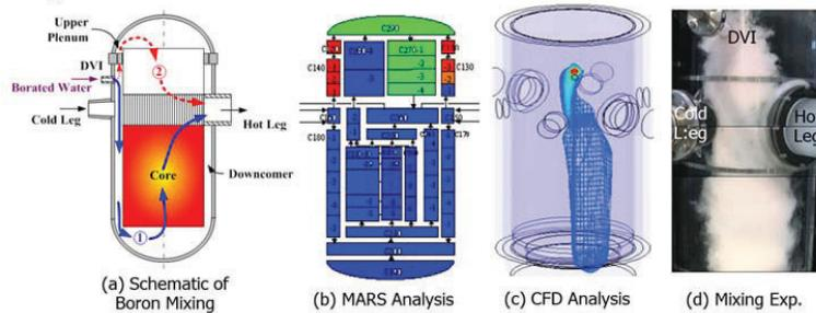
**Fig. 13 Mixing of Borated Water in a RV Downcomer**
