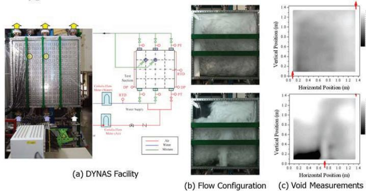
**Fig. 12 DYNAS Test for a Two-dimensional Two-Phase Flow**
