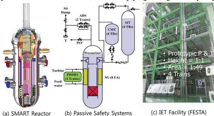
**Fig. 3 Passive Safety Systems in SMART and its Testing on the FESTA Facility**
