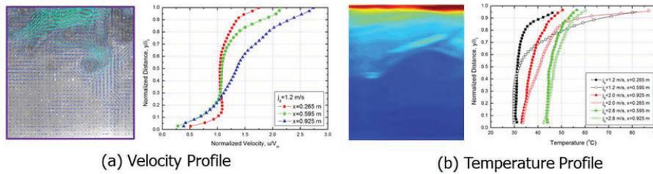
**Fig. 11 Velocity and Temperature Distributions Measured near the Condensing Interfaces**
