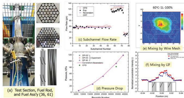
Fig. 5 Hydraulic Characteristics in Subchannels of SFR Fuel
