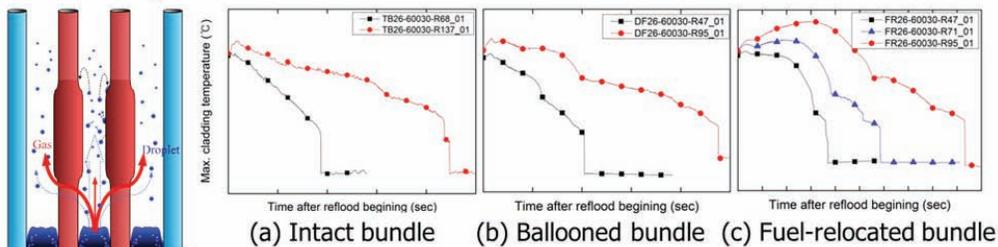
**Fig. 9 Effect of Ballooning and Fuel Relocation on the Reflood PCT**
