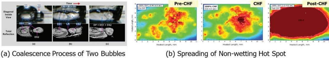
**Fig. 10 Coalescence Process of Bubbles and the Spreading of Non-wetting Hot Spot**
