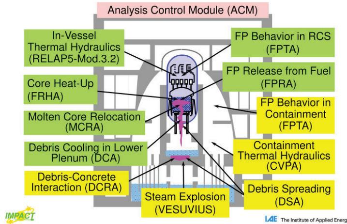
**Figure 5. SAMPSON : Severe Accident Analysis Code with Modular Structure.**
