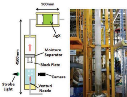
Figure 7. FCVS Test Facility at Hokkaido University [47].
