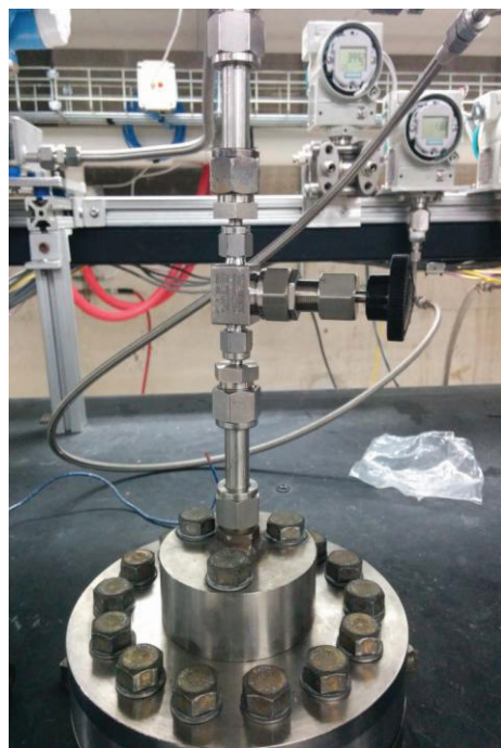
Figure 5. Test valve connected to test loop
