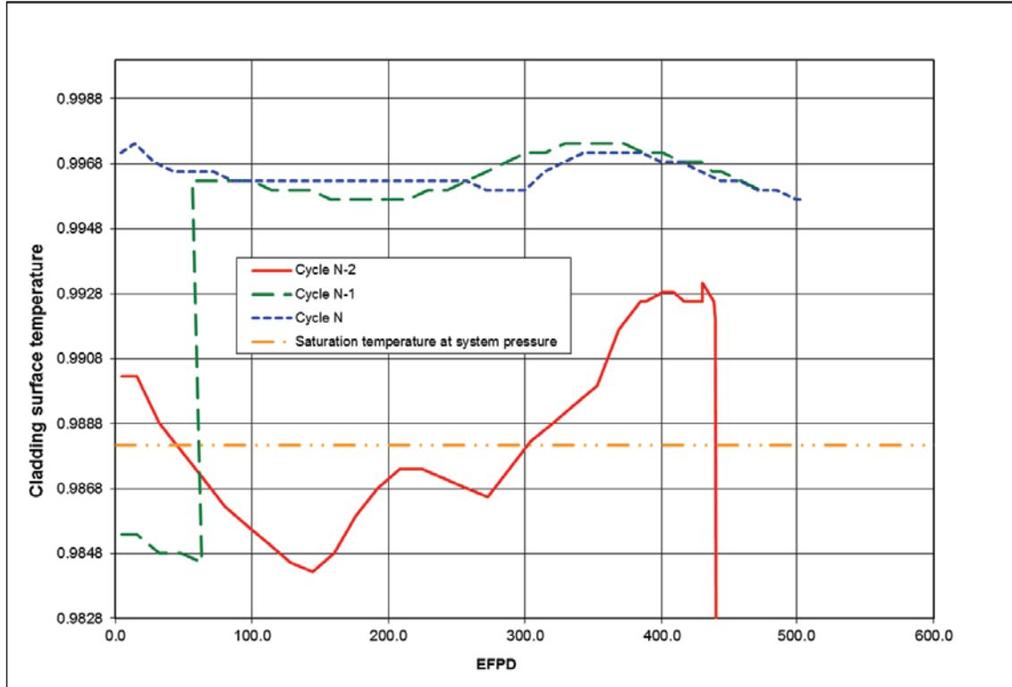
Figure 9: Normalized Clad Surface Temperature as a Function of EFPD for CE-14x14 Plant.
