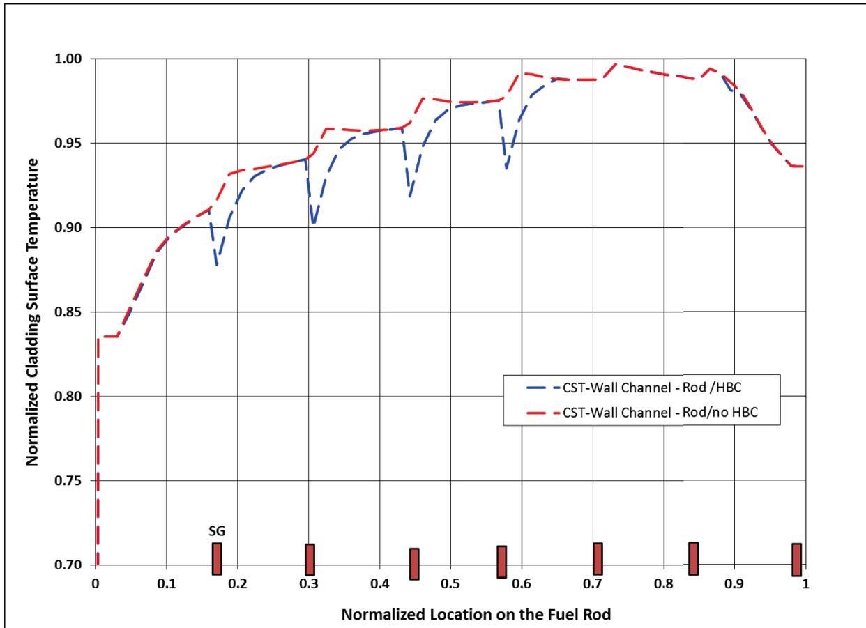
Figure 5: CST as a Function of Fuel Rod for HBC and Non-HBC Model.
