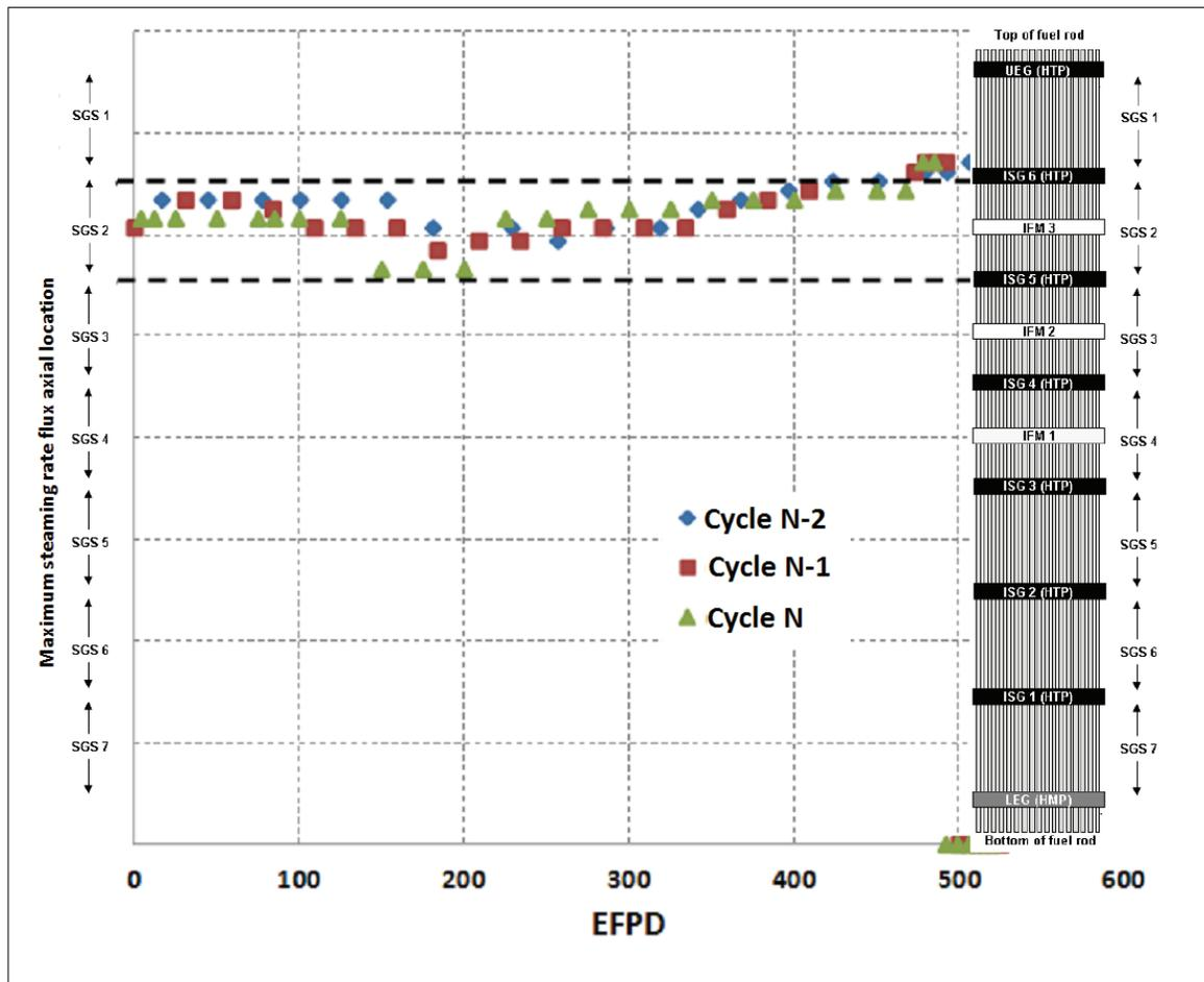
Figure 4: Axial Height of Limiting Key Decision Variable.
