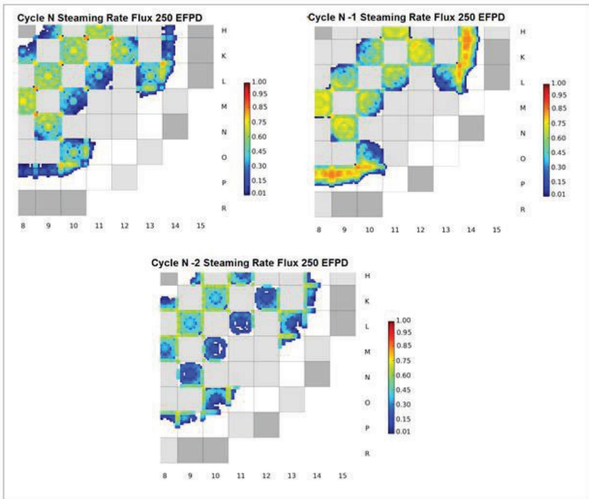
Figure 10: Steaming Rate Flux as a function of EFPD for B&W 177 Plant
