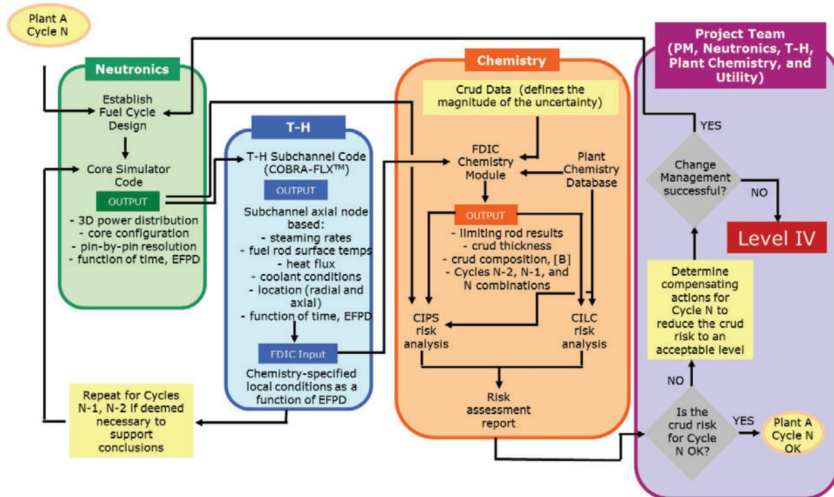
Figure 1: AREVA Level III Analysis Schematic
