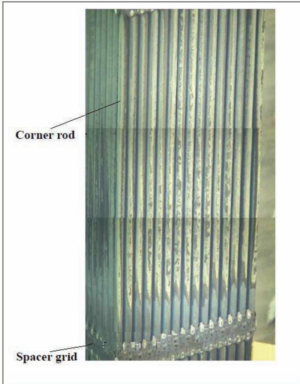
Figure 6: Crud Deposition Visuals from B&W 177 FA Plant.
