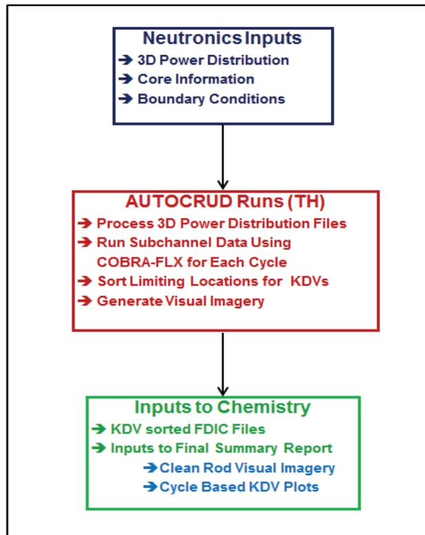
Figure 2: AUTO CRUD Process Schematic
