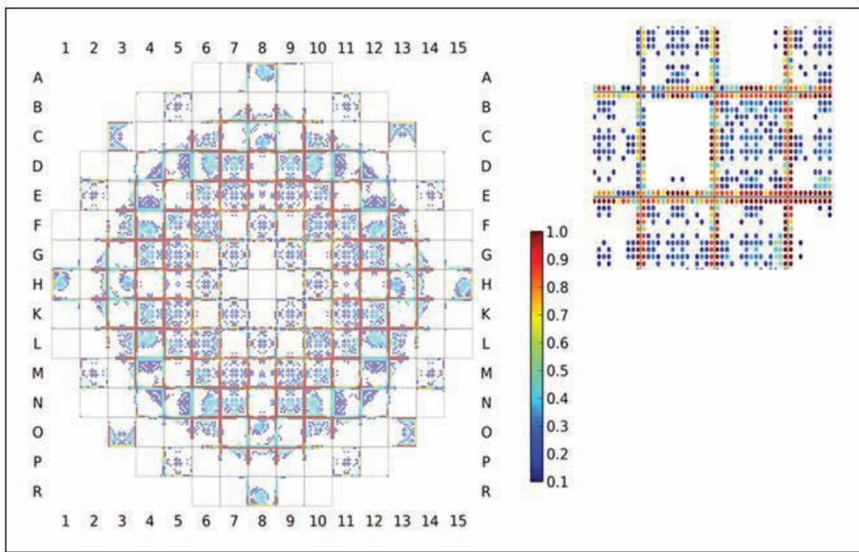
Figure 7: Lifetime Integrated Steaming Rate Fluxes for B&W 177 Plant.
