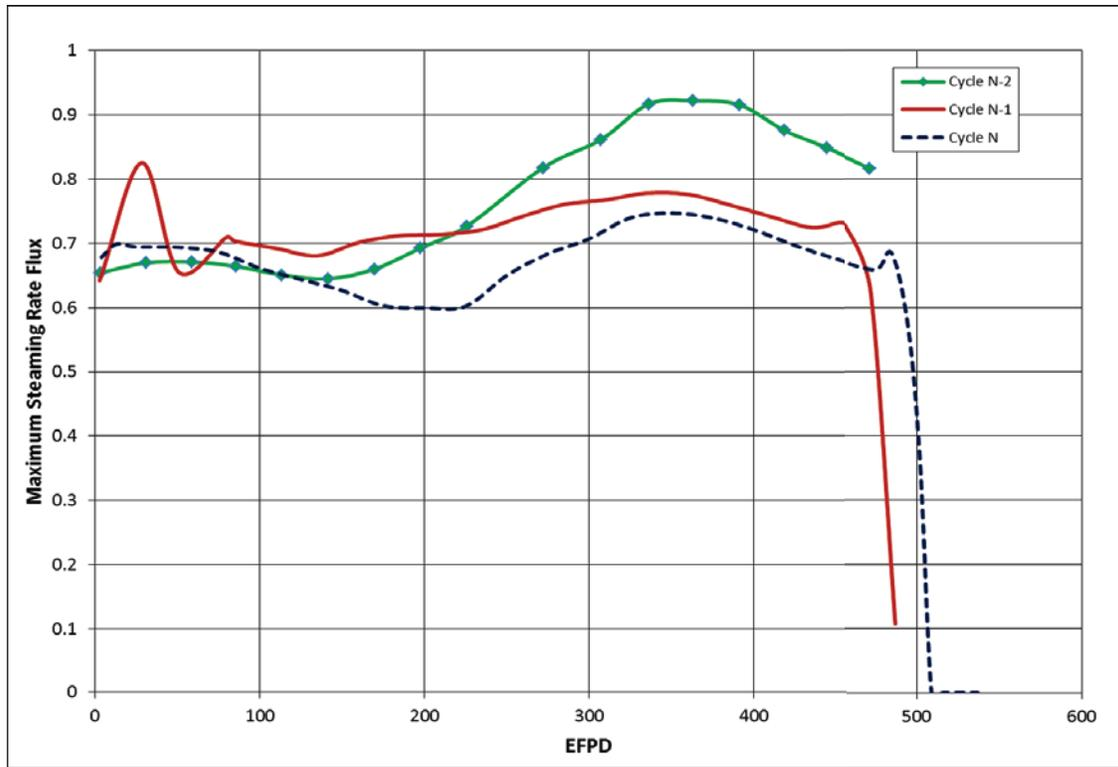
Figure 8: Normalized Steaming Rate Flux as a Function of EFPD for W-193 Plant.
