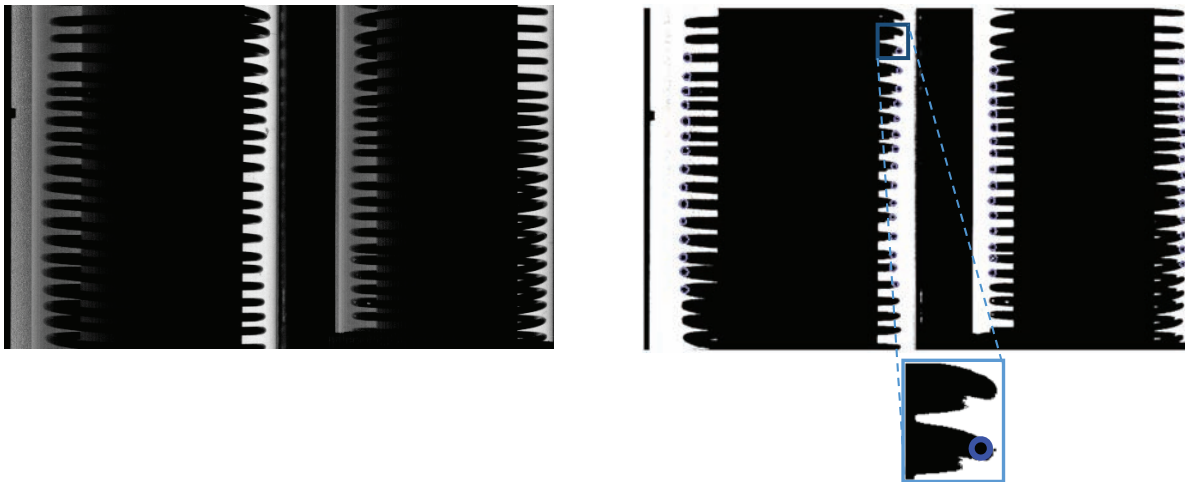
Figure 6. Raw image of coil (left), binary image with edge center locations mapped (right)
