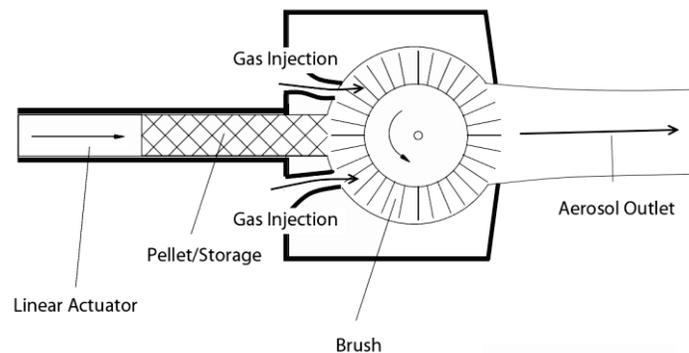
**Figure 4. Functional Principle of the PDB.**
