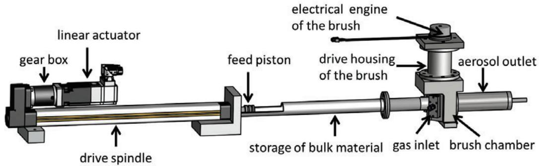
**Figure 3. Overall Technical Design of the PDB.**
