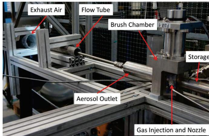
**Figure 7. Experimental Setup of the PDB for the Qualification of Tin Dioxide.**
