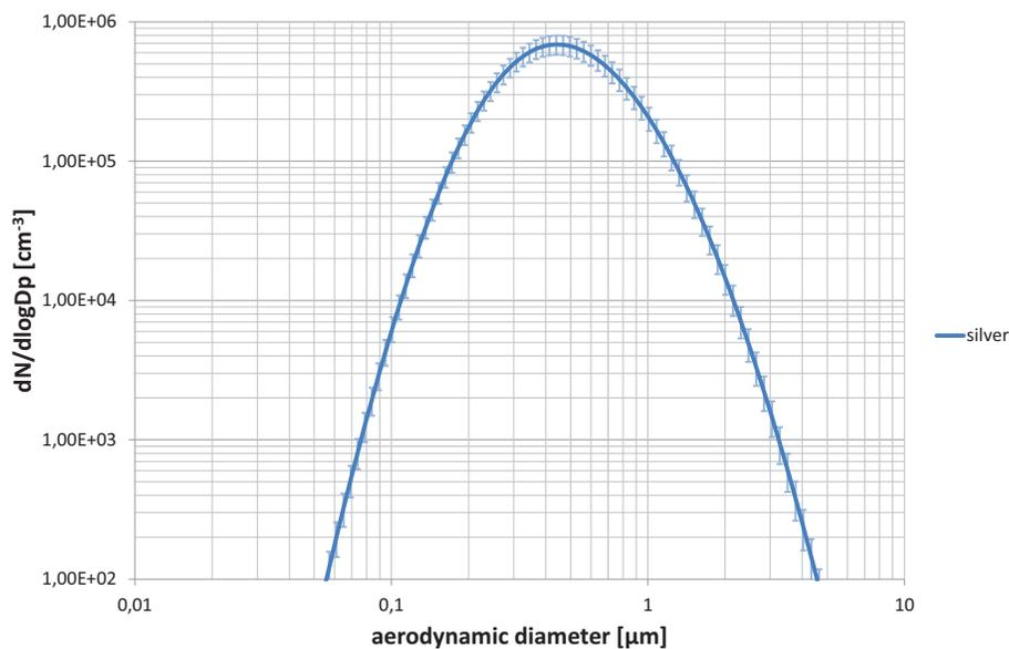
**Figure 15. Particle Size Distribution for a concentration of 1 g/m<sup>3</sup>.**
