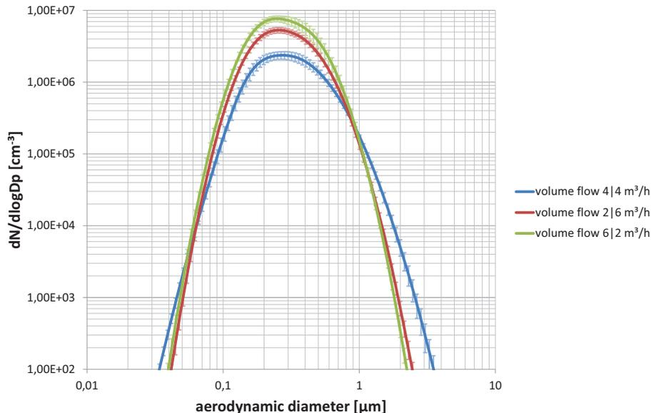
**Figure 11. Particle Size Distribution for a Total Volume Flow of 8 m<sup>3</sup>/h at Different Gas Injection Rates.**
