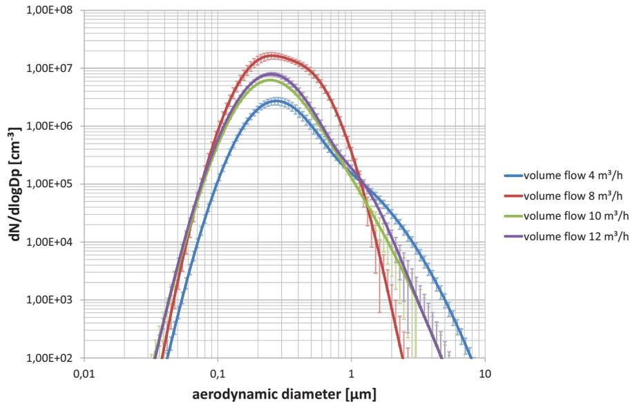
**Figure 10. Particle Size Distribution at Different Total Volume Flows.**
