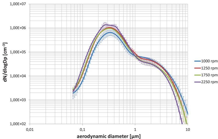
**Figure 8. Particle Size Distribution at Different Rotation Speeds of the Brush.**
