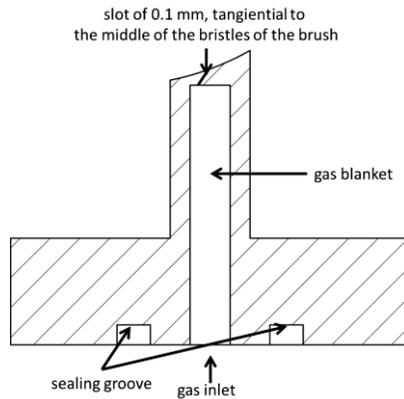
**Figure 5. Section Through the Gas Inlet Nozzle.**
