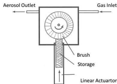
**Figure 1. Functional Principle of the RBG1000 from Palas GmbH [4].**
