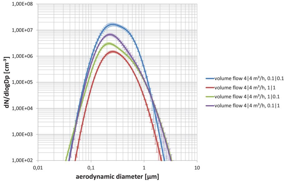
**Figure 12. Particle Size Distribution for a Total Volume Flow of 8 m<sup>3</sup>/h with Different Gas Injection Nozzles.**
