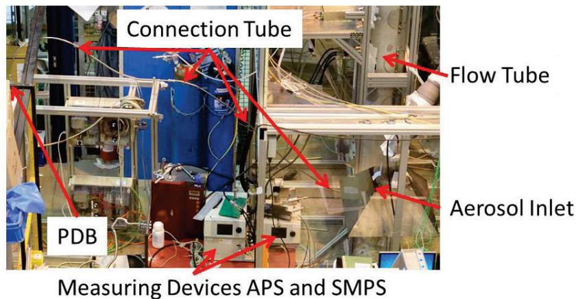
Figure 14. Experimental Setup of the PDB for the Qualification of Silver.
