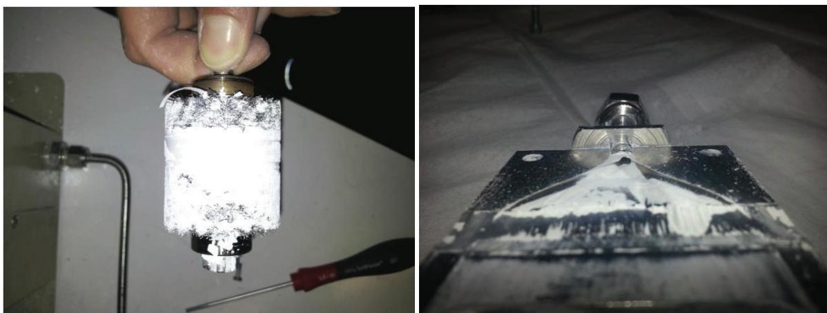
**Figure 2. Tin Dioxide Deposition on the Brush (left) and in the Nozzle and the Mixing Area (right) of the RBG1000.**
