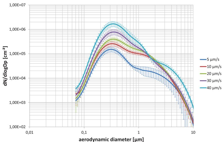
**Figure 9. Particle Size Distribution at Different Feed Rates.**
