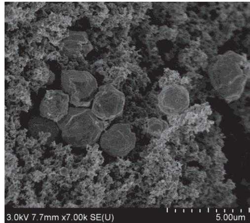
Figure 13. SEM Image of a Dispersed Compound Pellet of Tin Dioxide and Silver (5 w/o).
