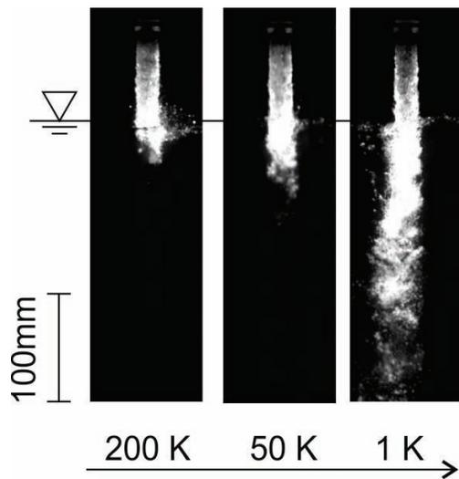
**Figure 11:** Instantaneous high speed camera images of plunging jet experiments at 50 bar and 1 kg/s injection mass flow rate for three different sub-cooling conditions.
