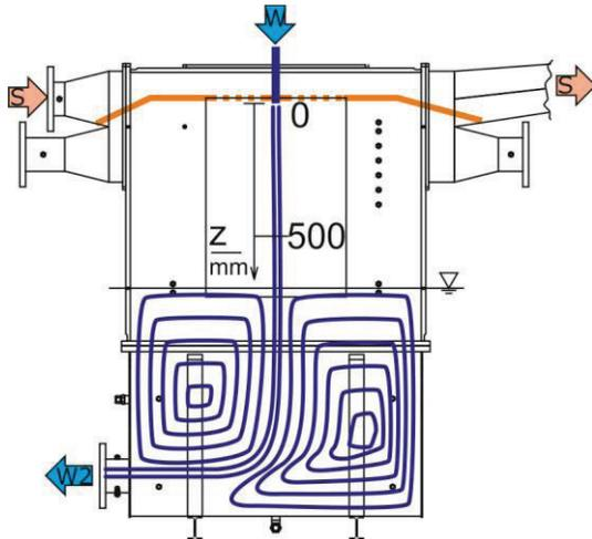
**Figure 7:** Flow conditions in terms of idealized streamlines (blue) for the jet flow experiments and steam flow guides (orange).
