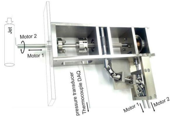
**Figure 8:** Thermocouple and dynamic pressure lance with gear for measuring profiles inside the condensing jet.
