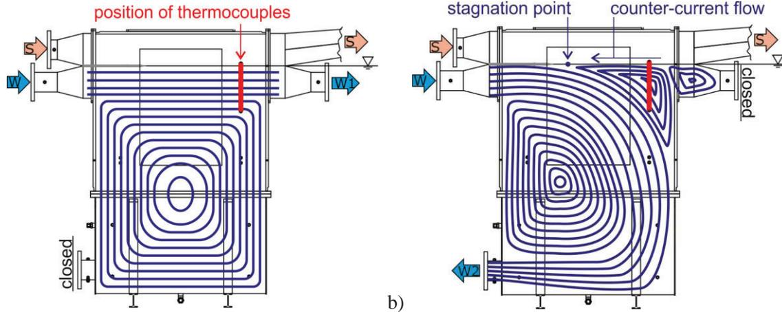
**Figure 4: Flow conditions in terms of idealized streamlines for (a) co-current and (b) partly counter-current stratified flow experiments. The red line shows the position of thermocouples presented in Figure 5 and 6.**
