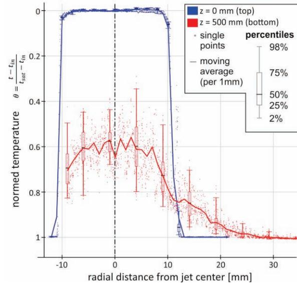
**Figure 10:** Normed temperature profile at two positions inside a condensing jet
