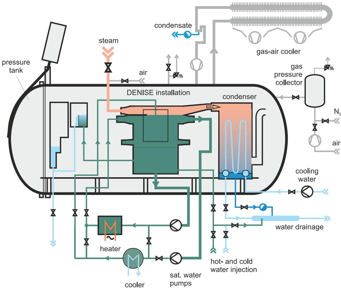
Figure 3: TOPFLOW pressure tank with DENISE installation
