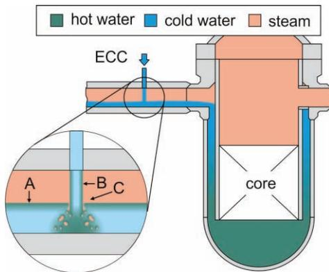
**Figure 1:** Pressurized thermal shock scenario with partly covered cold leg
