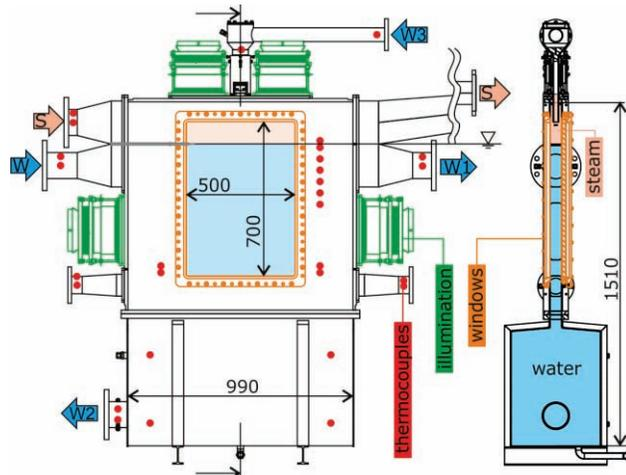
**Figure 2:** TOPFLOW-DENISE facility with flow directions of steam (S) and water (W)
