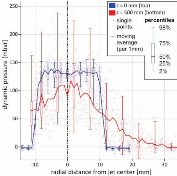
**Figure 9:** Dynamic pressure profile at two positions inside a condensing jet.
