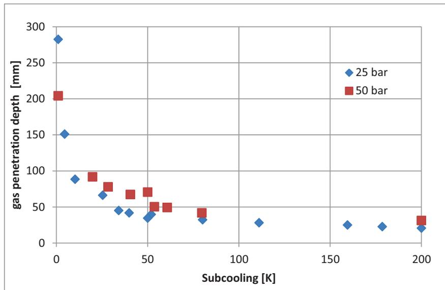
**Figure 13:** Gas penetration depth of plunging jet experiments with 1 kg/s jet mass flow rate at different pressures and inlet subcooling
