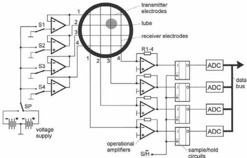
Figure 2. Scheme of conductance wire mesh sensor [5].
