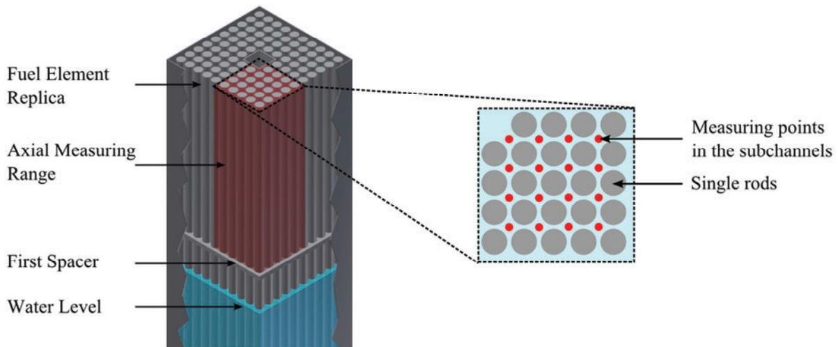
**Figure 1. Fuel element replica with measurement range (left) and measuring points (right).**
