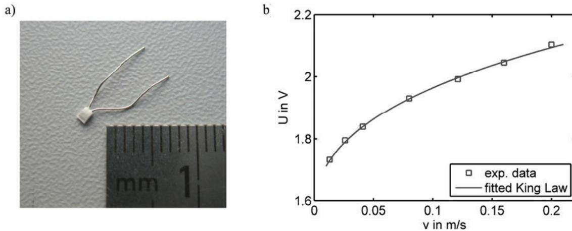
**Figure 4. a) Miniature PT100 sensor and b) calibration curve for CTA mode.**
