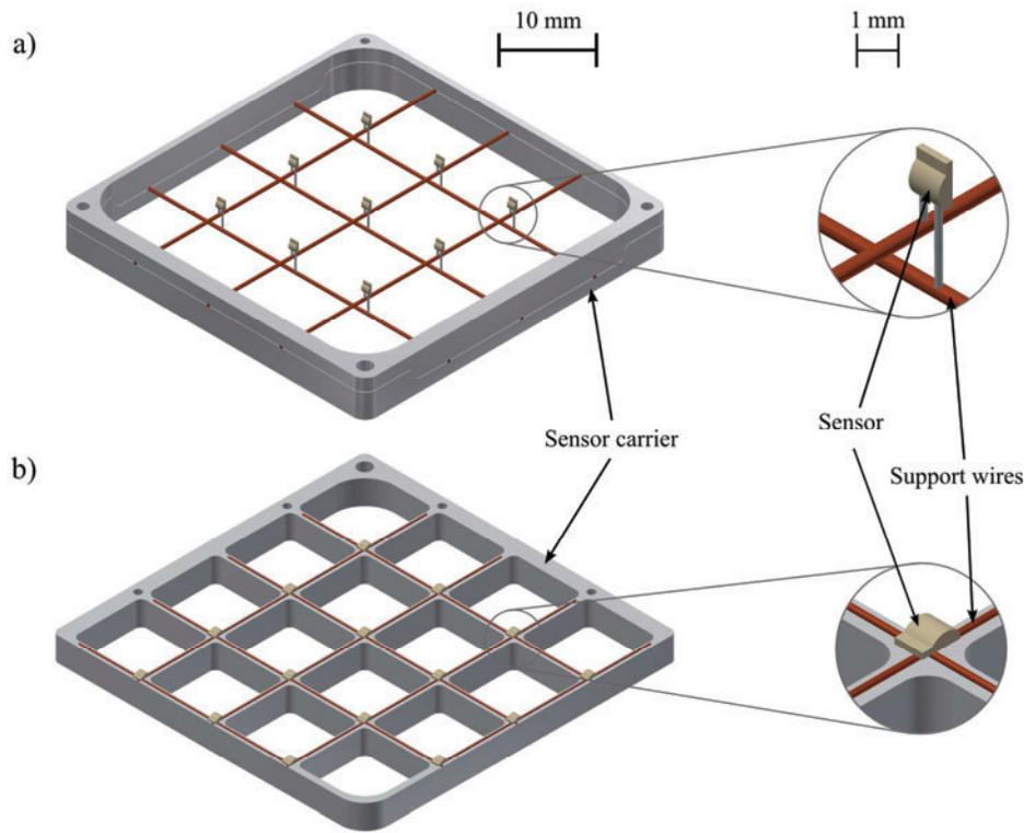
Figure 3. Design variants for the grid HFA sensor.
