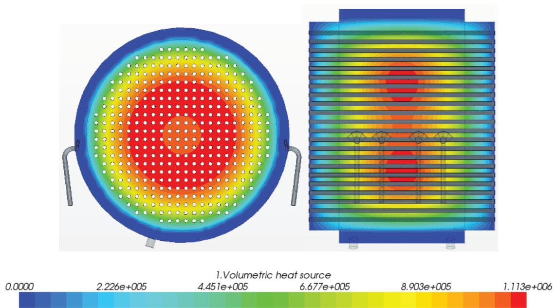
Fig. 6 Volumetric Heat Distribution in the radial and axial direction for CANDU-6 ( $W/m^3$ )
