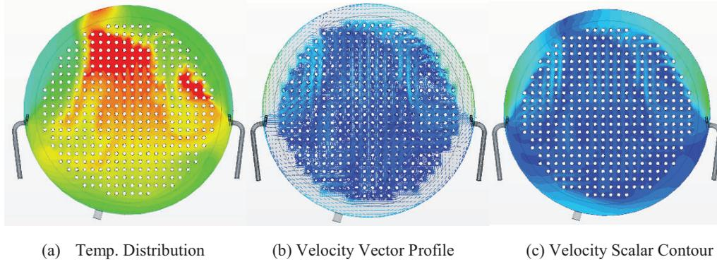
Fig. 7 Temperature and Flow Distribution at the Axially Middle Plane for CANDU-6 Moderator Circulation at a Full Power Steady State Condition (STAR-CCM+).
