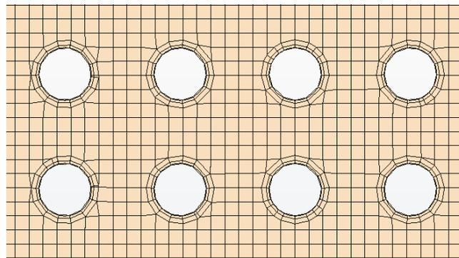
(b) Mesh Grid Adjacent to the Fuel Channels
