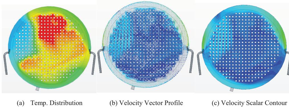
Fig. 8 Temperature and Flow Distribution at the Axially Middle Plane for a 1/4 Scaled-down MCT at a Steady State Condition with 0.5 MW (STAR-CCM+).
