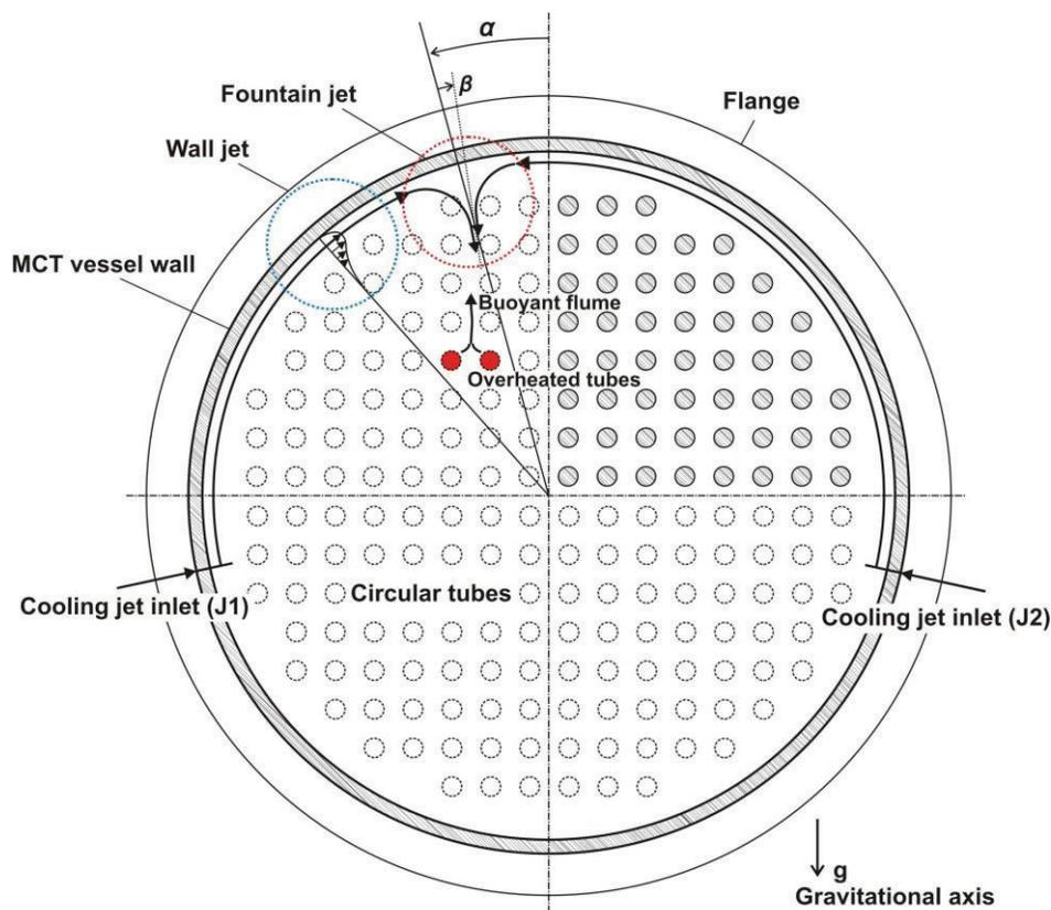
**Fig. 3** Schematic diagram of a moderator tank of a CANDU-6 depicting the inlet jet collision and resulting recirculating fountain flow.
