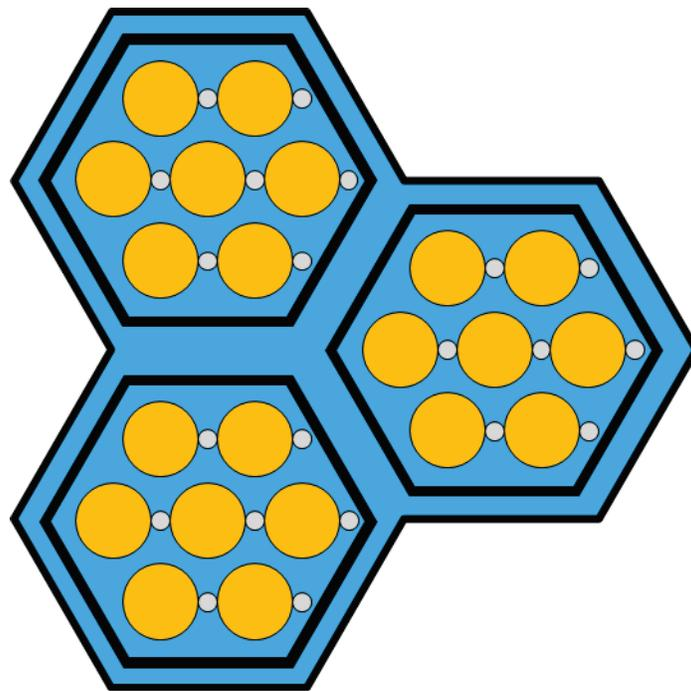
**Figure 3. Outline of the inter-wrapper flow experiment (KIT).**
