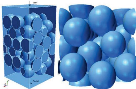
Figure 1. Schematic of the computational domain (left) iso-metric view (right) top view.
