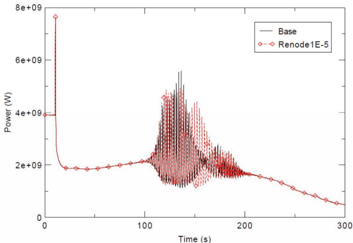
**Figure 2. Transient Power Responses for Base Case and Renode1E-5 Case.**
