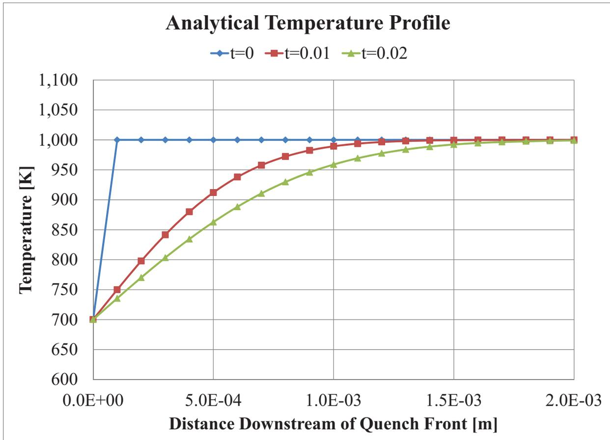
Figure 1. Analytical Temperature Gradient Downstream of Quench.
