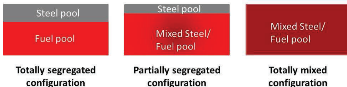
Figure 4: Various configuration of material repartition inside the upper or lower fissile zone.
