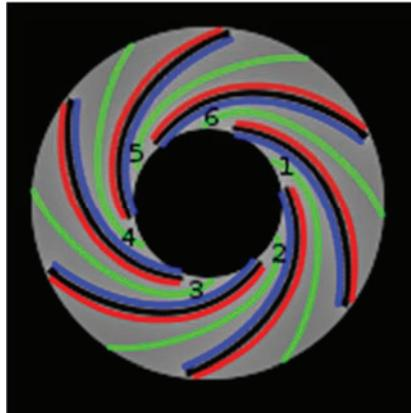
**Figure 5. Illustration of pressure-side streamlines (red), center streamlines (green) and suction-side streamlines (blue), which were selected for the analysis of the gas holdup profiles in the six impeller chambers.**
