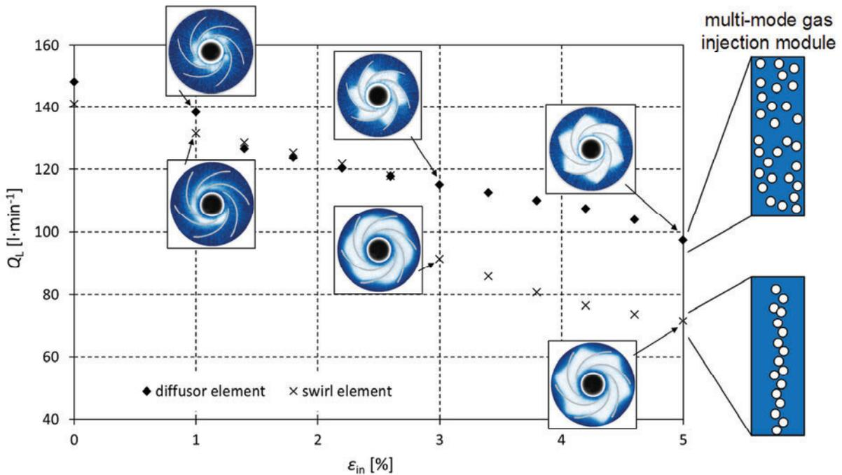
**Figure 4. Internal accumulated gas holdup pattern and pump performance depending on the inlet gas volume fraction and inlet flow regimes.**
