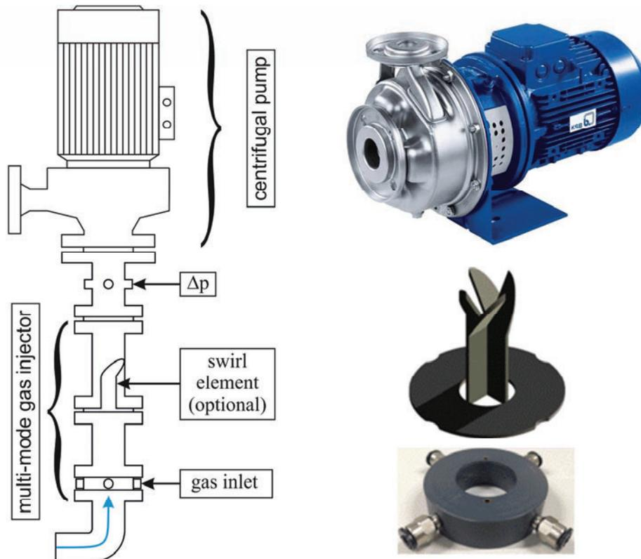
**Figure 1. Simplified scheme of the modular pump test section with multi-mode gas injection module and investigated centrifugal pump.**
