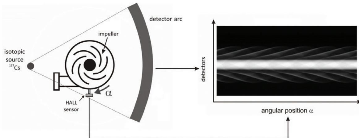
**Figure 2. Principle of time-averaging rotation-synchronized computed tomography scanning mode.**
