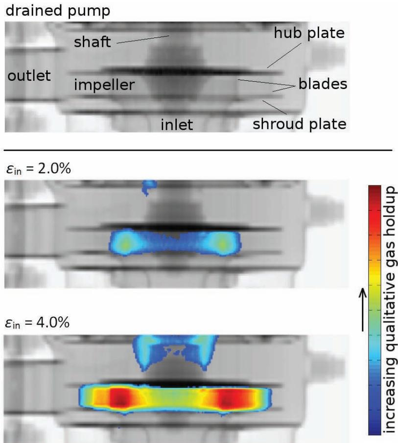
**Figure 3. Radiographies of typical vertical gas holdup formations near to the shaft and inside the impeller wheel, depending on two different inlet gas volume fractions. For better illustration all regions fully liquid are not represented in the radiographies.**
