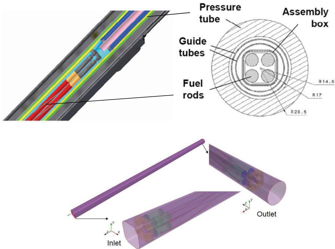
**Figure 1. (Top) SCWR-FQT test section: On the left a view inside the test section with the fuel rods in red and on the right a cross-cut through the active channel (Bottom) Selection of the computational domain.**
