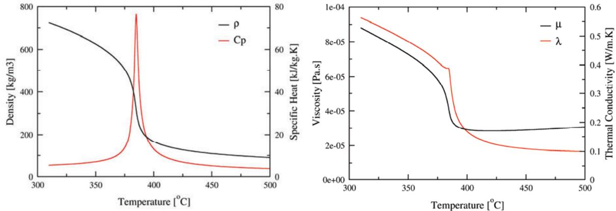
**Figure 2. Temperature dependent properties of SCW at 25MPa [11].**
