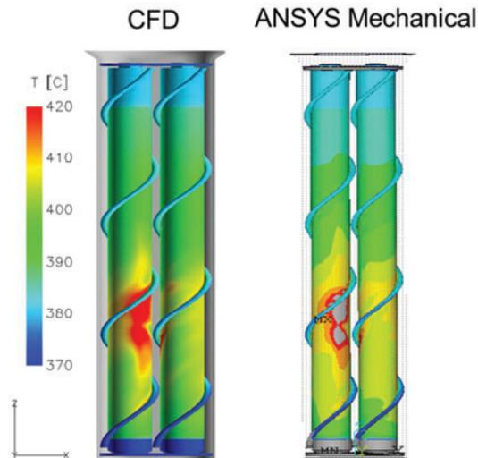
**Figure 6. Comparison of the temperature distribution from CFD and the temperature distribution in ANSYS after mapping.**
