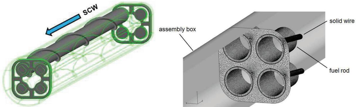
**Figure 3. CFD geometry and mesh. The picture on the left shows the geometry of one of the four wire-wrapped rods as well as the rod support plates at bottom and top. On the right, a cross section through the FQT fuel assembly with mesh.**
