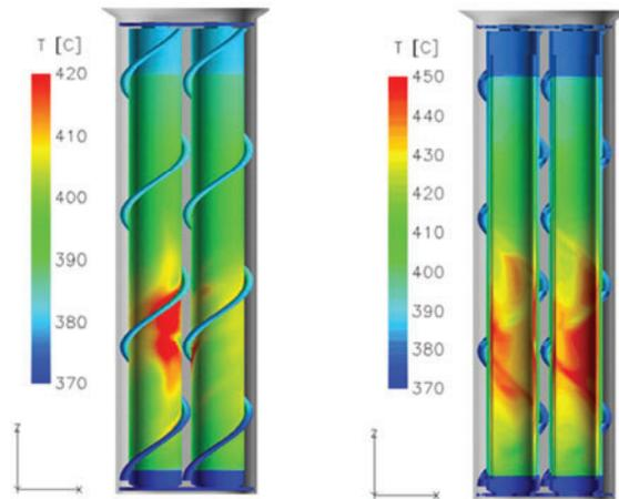
**Figure 4. Temperature distribution on outer (left) and inner surface (right) of the fuel rods**
