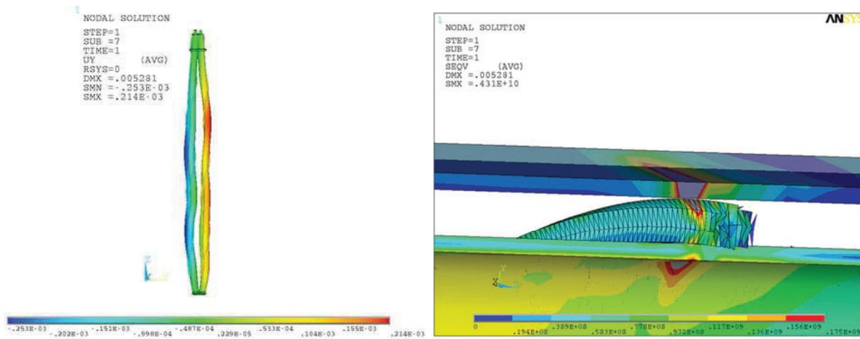
**Figure 7. Left, the thermal deformation due to non-uniform cooling (scaled with factor 400 for better visualization). Right, the localized stresses as the result of bending of the rods towards the assembly box.**
