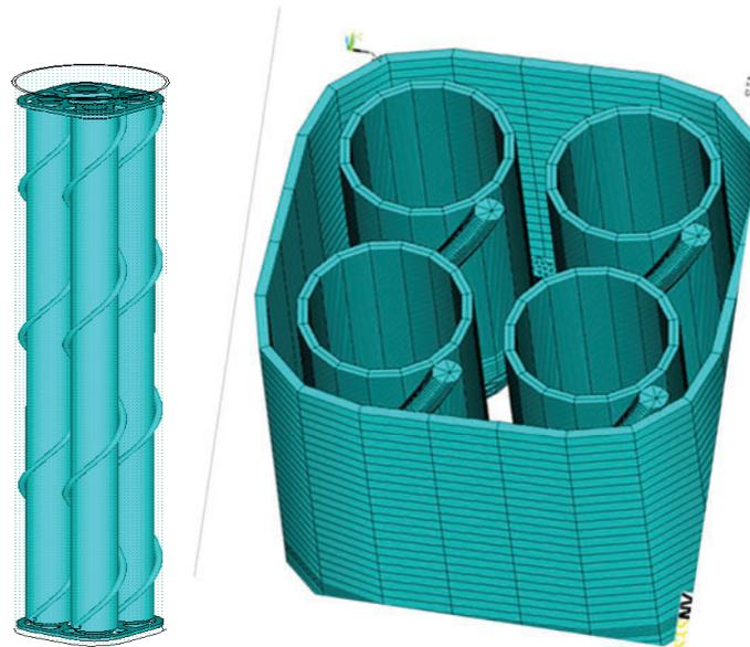
**Figure 5. Geometry and mesh for structural analysis.**
