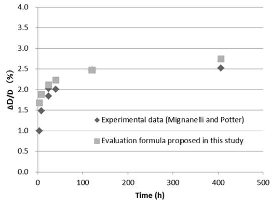
**Figure 3. Fuel pellet diameter increase due to FSRP formation at 700 degree C**
