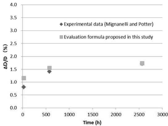
**Figure 4. Fuel pellet diameter increase due to FSRP formation at 650 degree C**
