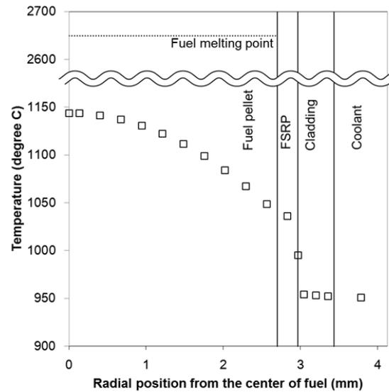
**Figure 7. Temperature distribution from center of fuel pin with FSRP layer of which thickness is 10% of fuel radius**
