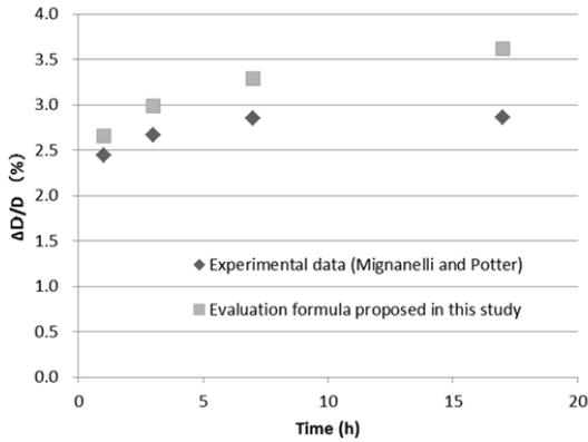
**Figure 2. Fuel pellet diameter increase due to FSRP formation at 800 degree C**
