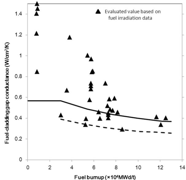
**Figure 8. Fuel-cladding gap conductance cited from the Monju licensing**
