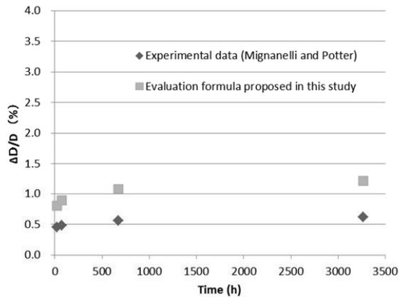
**Figure 5. Fuel pellet diameter increase due to FSRP formation at 600 degree C**
