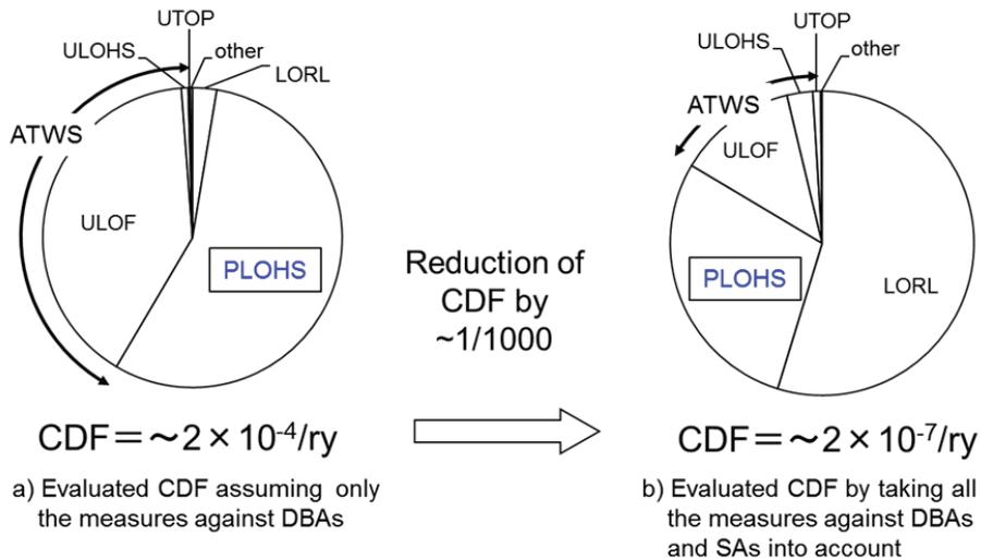
**Figure 1. Accident sequence groups identified based on the internal event PRA**
