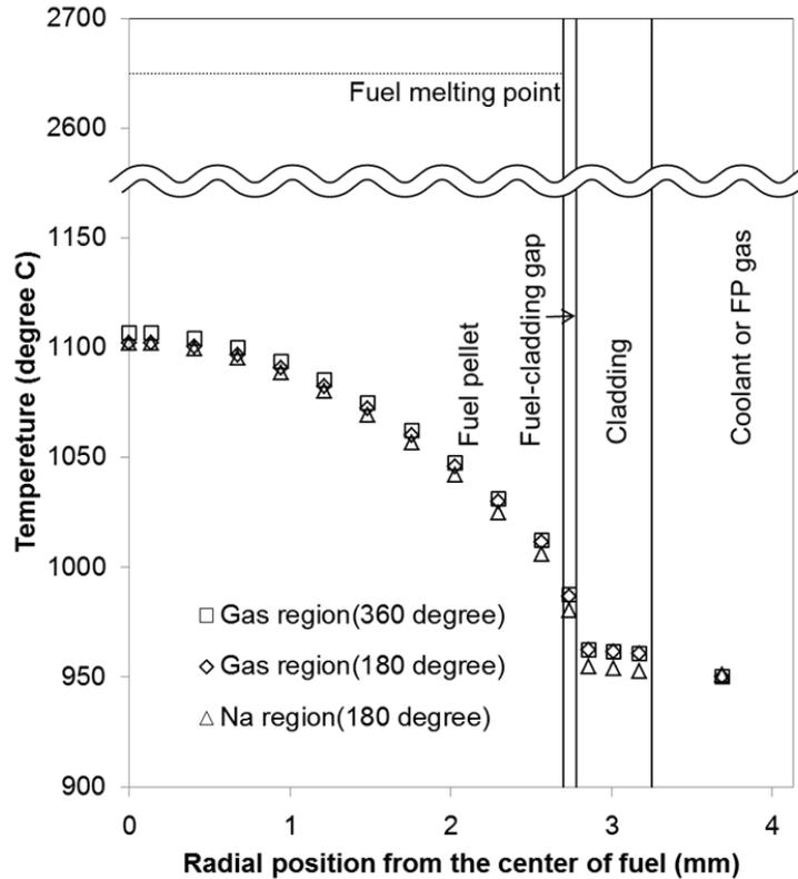
**Figure 11. Temperature distribution from the center of fuel pin during FP gas release from adjacent fuel pins**
