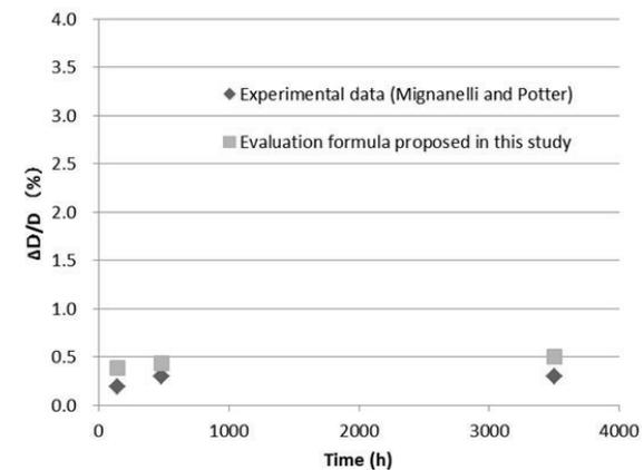
**Figure 6. Fuel pellet diameter increase due to FSRP formation at 500 degree C**
