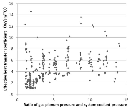
**Figure 10. Effective heat transfer coefficient between released FP gas from the failed fuel pin and cladding of adjacent fuel pin**
