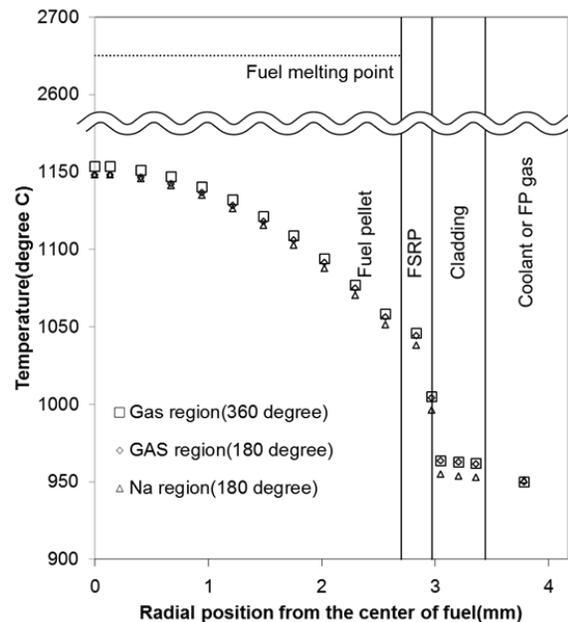
**Figure 12. Temperature distribution from the center of fuel pin with FSRP layer of which thickness is 10% of fuel radius during FP gas release form adjacent fuel pins**
