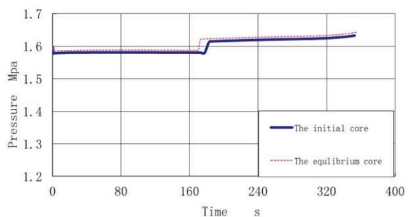
**Figure 7. The System Pressure Curve of the ATWS Induced by Station Blackout**
