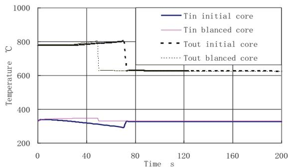
**Figure 17. The Core Inlet and Outlet Temperature Curve of the ATWS Induced by One control Rod Withdrawal**
