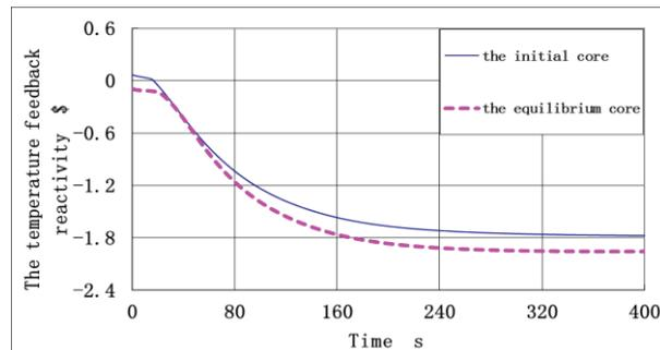
**Figure 25. The Temperature Feedback Reactivity Curve of the Last ATWS**
