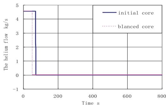
**Figure 16. The Main Loop Flow Curve of the ATWS Induced by One Control Rod Withdrawal**
