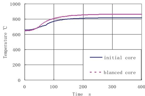
**Figure 14. The Fuel Average Temperature Curve of the ATWS Induced by One Control Rod Withdrawal**
