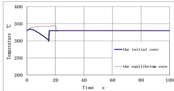
**Figure 23. The Core Inlet Helium Temperature Curve of the Last ATWS**
