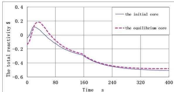
**Figure 21. The Total Reactivity Curve of the Last ATWS**
