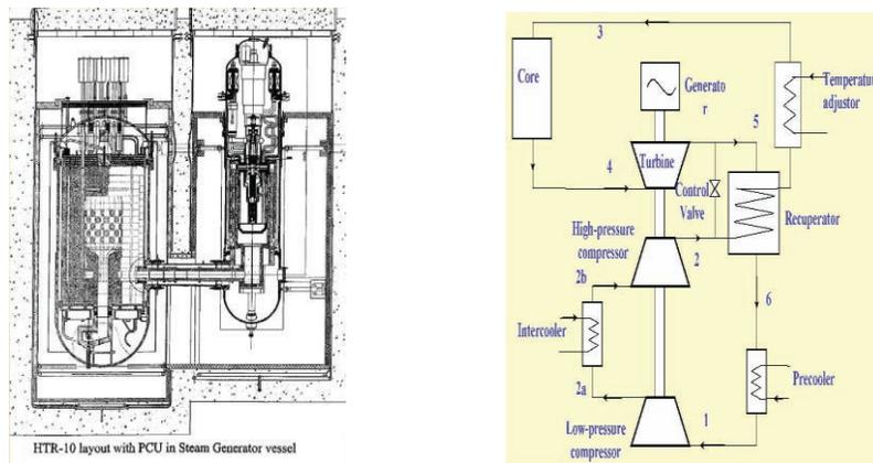
**Figure 1. The Layout and Schematic diagram of HTR-10GT**
