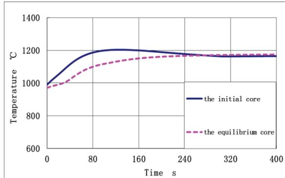
**Figure 19. The Fuel Peak Temperature Curve of the Last ATWS**
