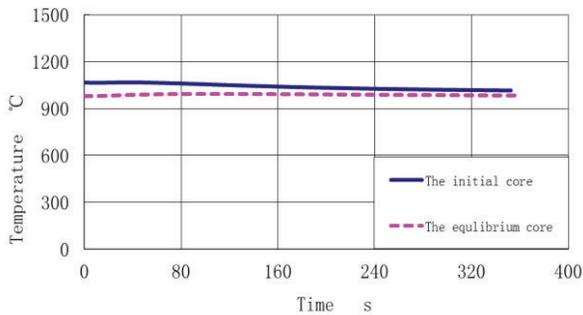
**Figure 6. The Peak Fuel Temperature Curve of the ATWS Induced by Station Blackout**
