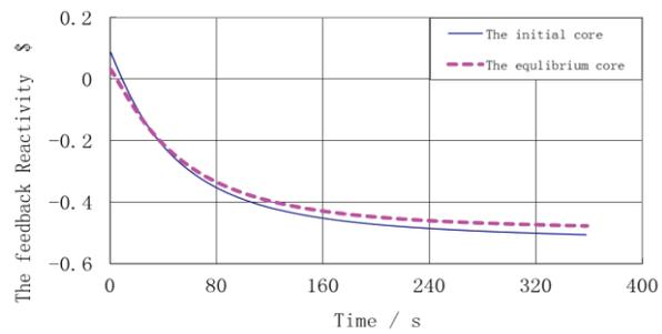
**Figure 5. The Feedback Reactivity Curve of the ATWS Induced by Station Blackout**
