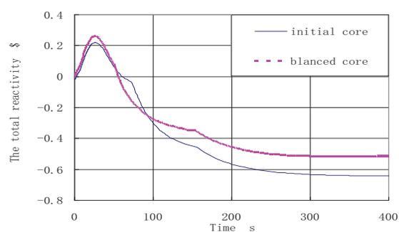
**Figure 15. The Total Reactivity Curve of the ATWS Induced by One Control Rod Withdrawal**
