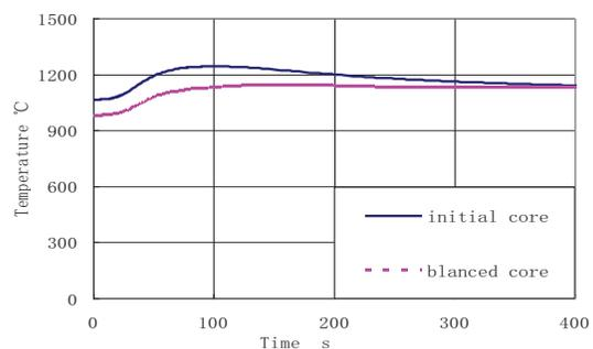
**Figure 13. The Fuel Maximum Temperature Curve of the ATWS Induced by a Control Rod Withdrawal**
