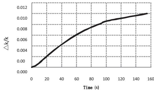
Figure 3. The Reactivity Inserted by a Control Rod Withdrawal
