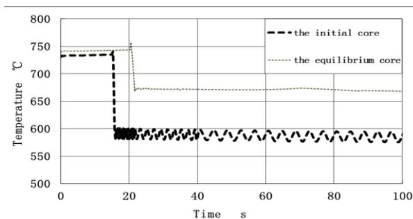
**Figure 24. The Core Outlet Helium Temperature Curve of the Last ATWS**
