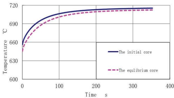
**Figure 8. The Mean Temperature Curve of the ATWS Induced by Station Blackout**
