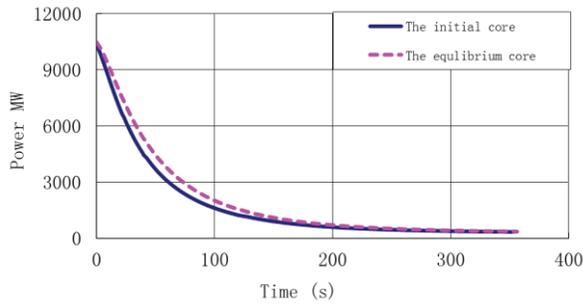
**Figure 4. The Power Curve of the ATWS Induced by Station Blackout**
