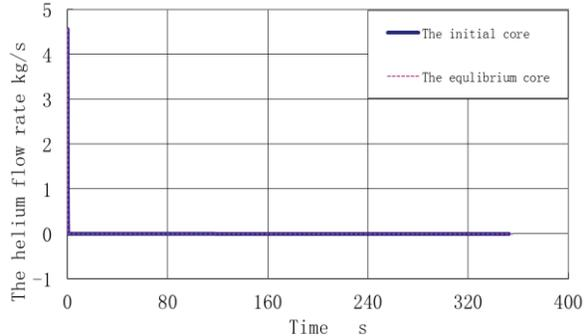
**Figure 9. The Helium Flow Rate Curve of the ATWS Induced by Station Blackout**
