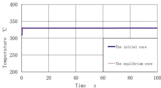
**Figure 10. The Inlet Temperature Curve of the ATWS Induced by Station Blackout**
