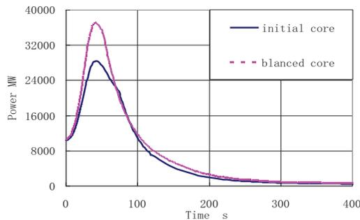
**Figure 12. The Power Curve of ATWS Accident Induced by One Control Rod Withdrawal**
