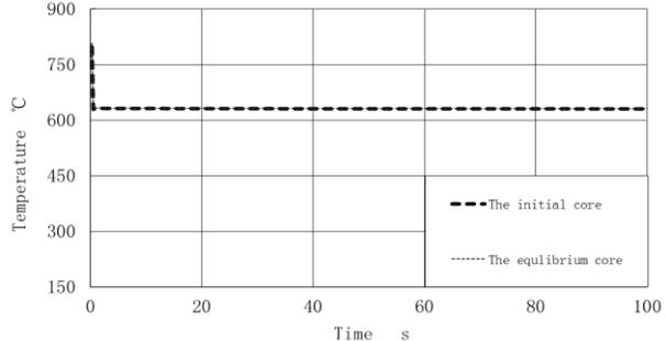
**Figure 11. The Outlet Temperature Curve of the ATWS Induced by Station Blackout**
