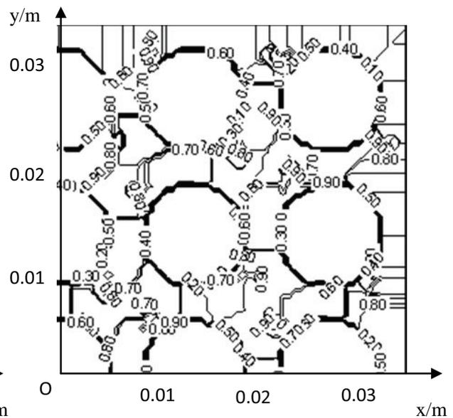
**Fig.15** Axial flow velocity on exit of mixing grid
