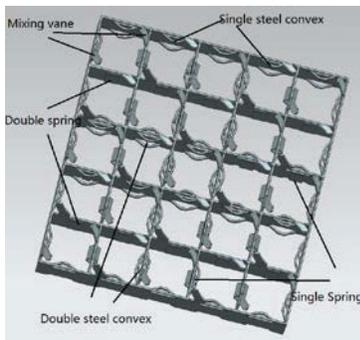
**Fig.1** Sketch of mixing vane fuel
