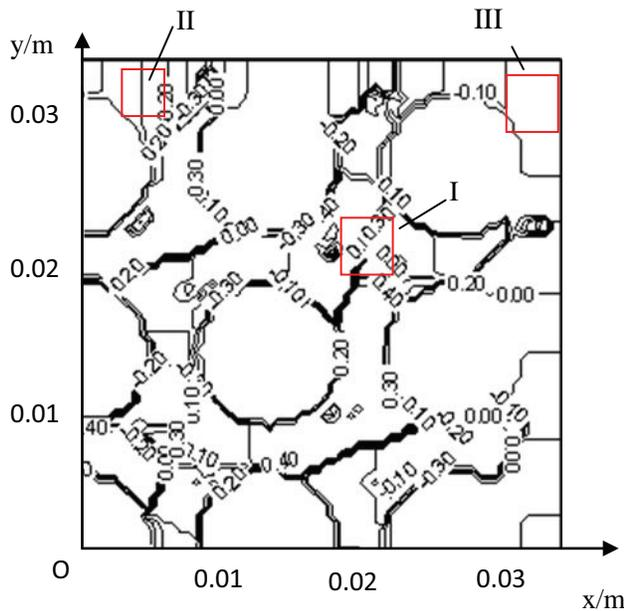
**Fig.14** Cross flow velocity on exit of mixing grid
