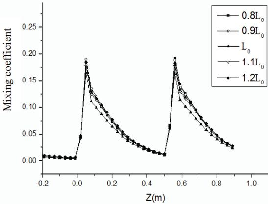
**Fig.18** Mixing coefficient for mixing vanes with different vane lengths
