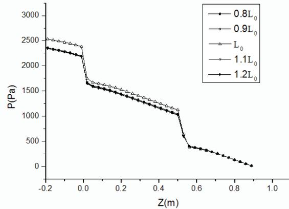
**Fig.19** Pressure drop for mixing vanes with different vane lengths
