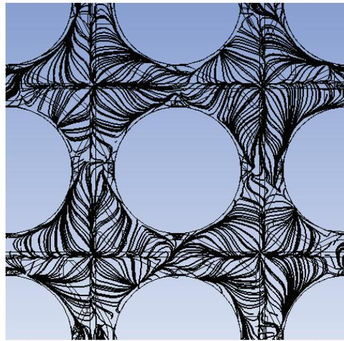
**Fig.12** Streamline of support grid exit.
