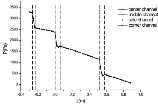
**Fig.7 Pressure drop in four channels.**
