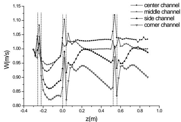
**Fig.10 Axial velocity in the four channels**
