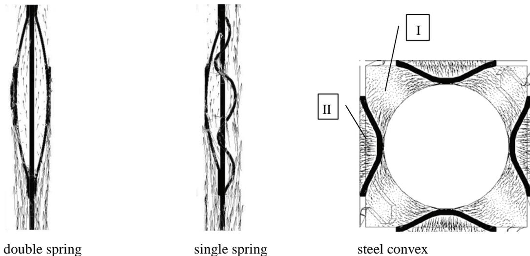
**Fig.13** Velocity vector of three structures of spacer grid and mixing grid.
