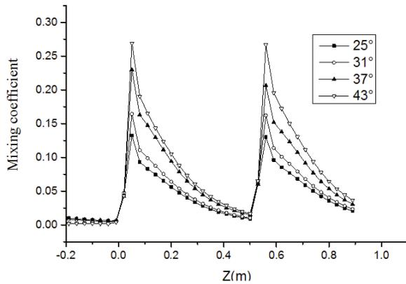
**Fig.16** Mixing coefficient for mixing vanes with different deflection angles mixing
