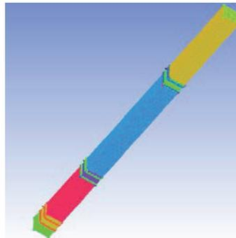
**Fig.2** Sketch and mesh of 5×5 fuel assembly
