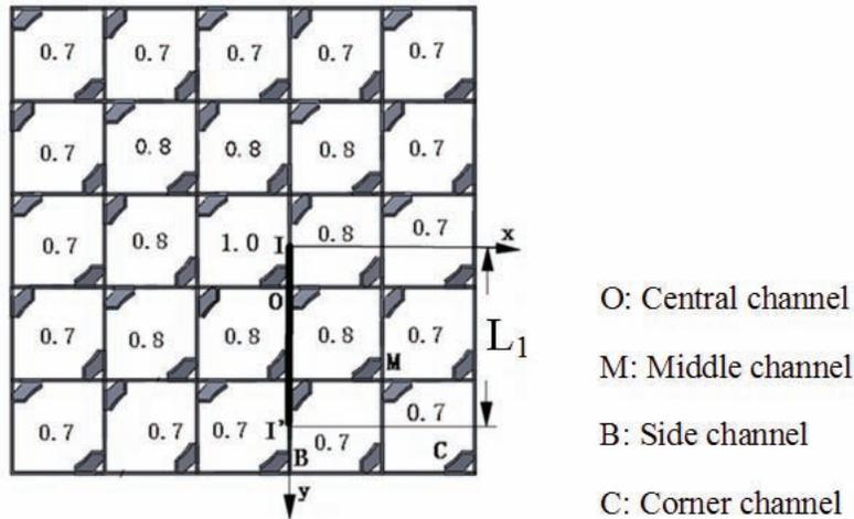
**Fig.6 Radial heat power of the 5×5 fuel assembly**
