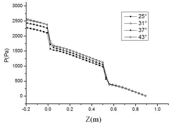
**Fig.17** Pressure drop of the fuel assembly for vanes with different deflection angles
