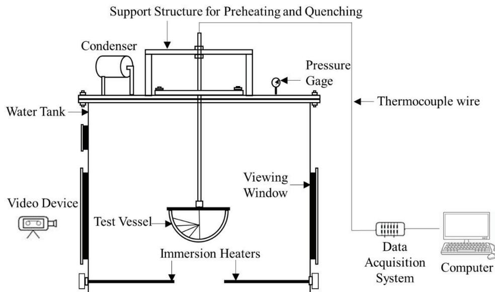
Figure 1. Schematic of the Quenching Setup in the SBLB Test Facility
