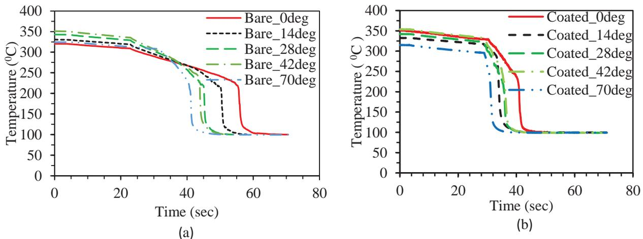
Figure 7. Local Boiling Curves Measured During Quenching (a) Bare Vessel and (b) Coated Vessel
