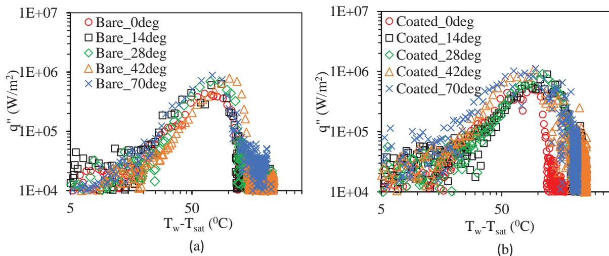
Figure 8. Boiling Curves at Different Angular Locations on a (a) Bare and (b) a Coated Test Vessel
