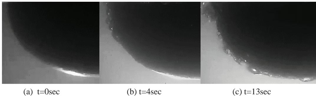
Figure 5. Quenching Phenomena Observed for the Bare Vessel
