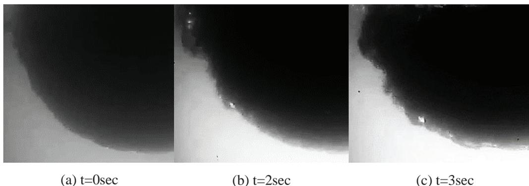
Figure 6. Quenching Phenomena Observed for the Coated Vessel
