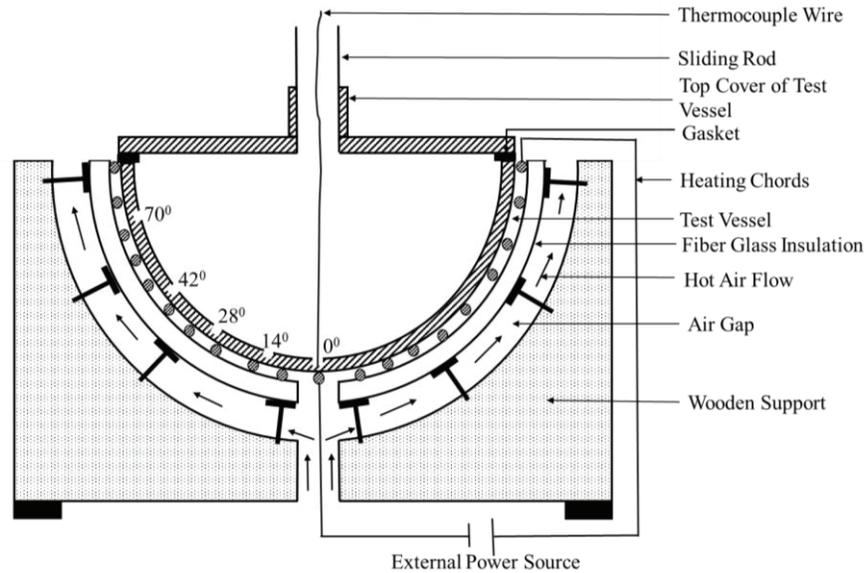
Figure 2. Schematic of the Test Vessel Being Preheated by the Customized Heating Mantle
