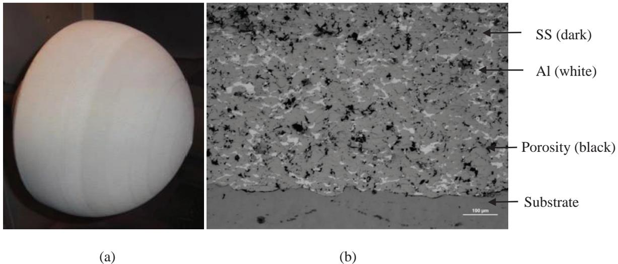
Figure 4. (a) Micro-Porous Coated Test Vessel and (b) Microscopic Image of the Coating at 100x
