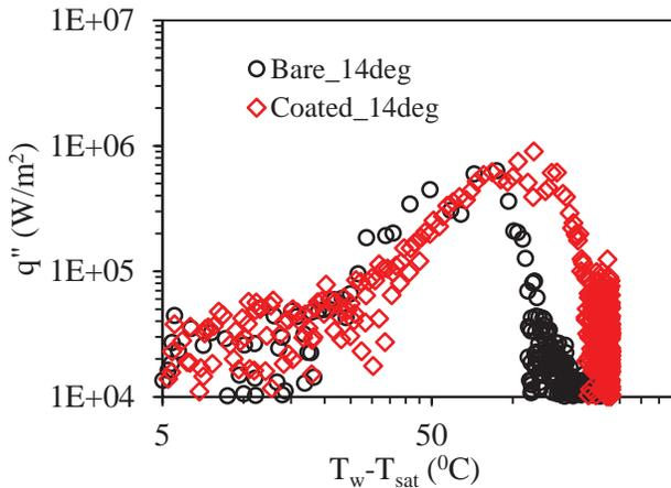
Figure 9. Comparison of the Boiling Curves between Bare and Coated Vessel
