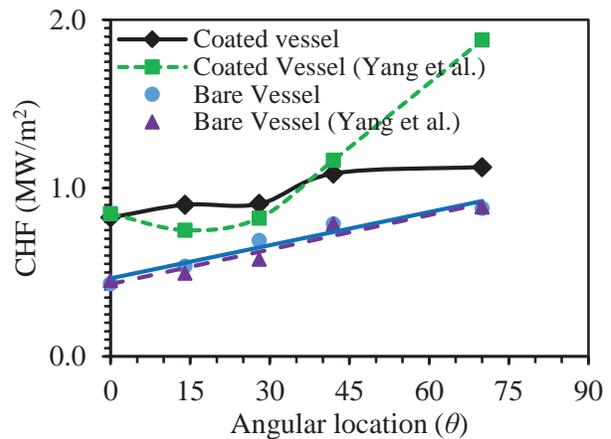
Figure 10. Variations of the Local CHF Limits on the Vessel Outer Surface
