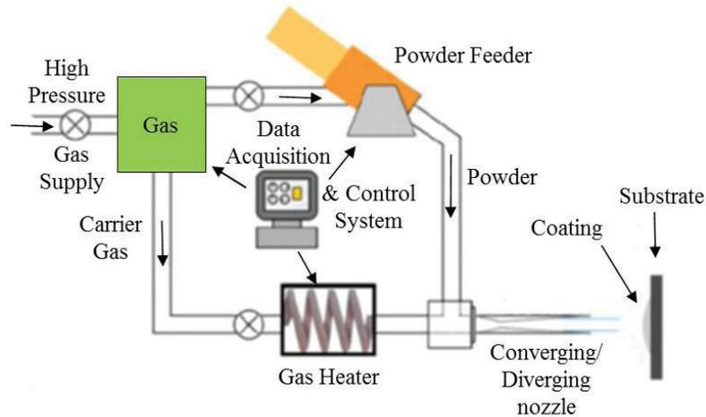
Figure 3. Schematic of the Cold Spray System
