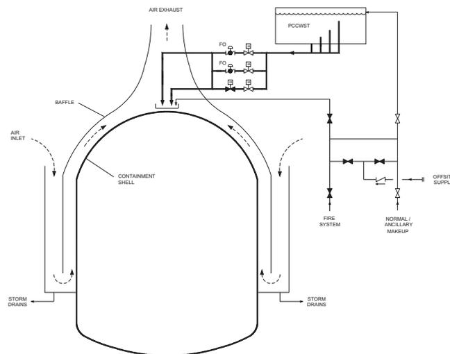
Figure 1. AP1000® Passive Containment Cooling System
