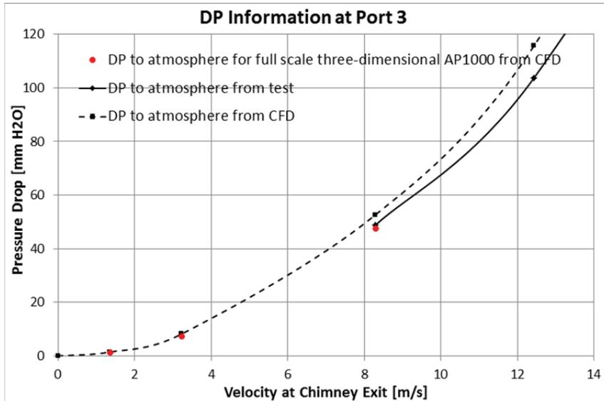
Figure 11. RAFT vs. CFD Comparison for Air Inlets
