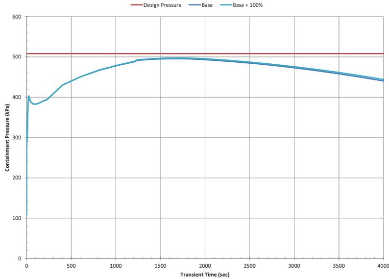
Figure 3. Containment Peak Pressure Sensitivity to Air Resistance – Large Break LOCA
