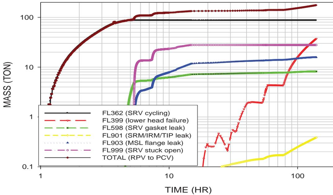
Figure 6. Integrated leakage masses from RPV to PCV
