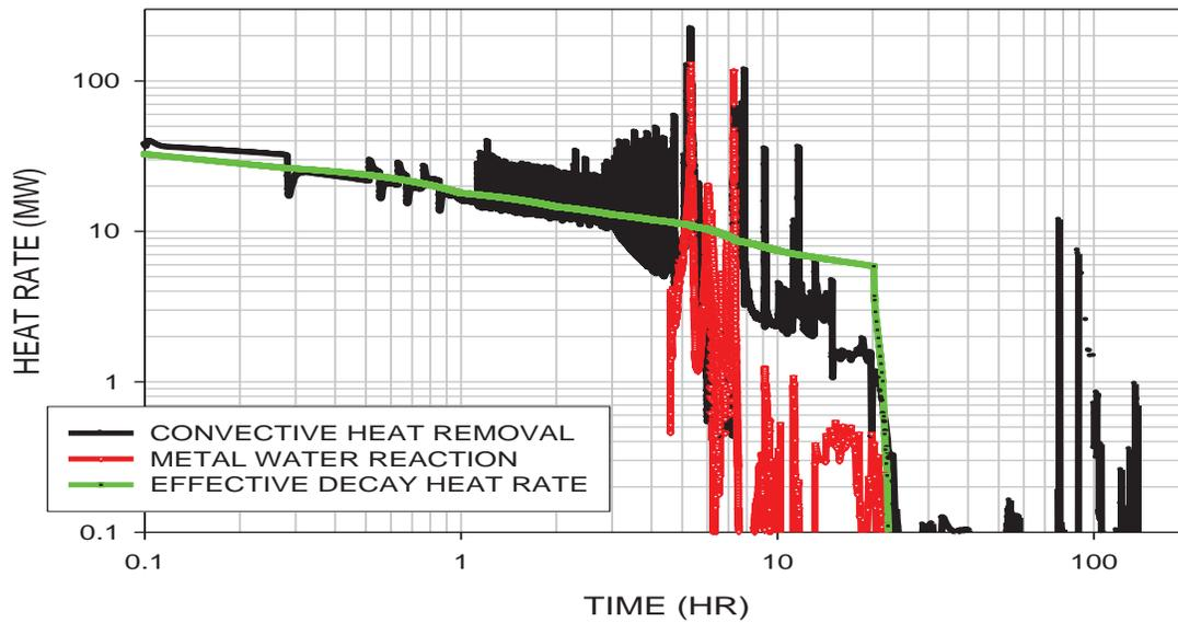
Figure 10. Heat balances at reactor core
