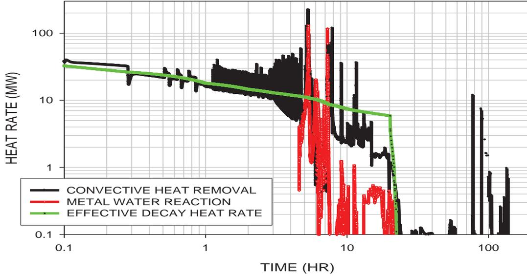
Figure 10. Heat balances at reactor core
