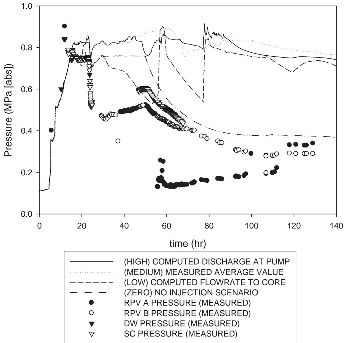
Figure 3. Calculated PCV pressures for 4 AWI scenarios and comparison with measured data
