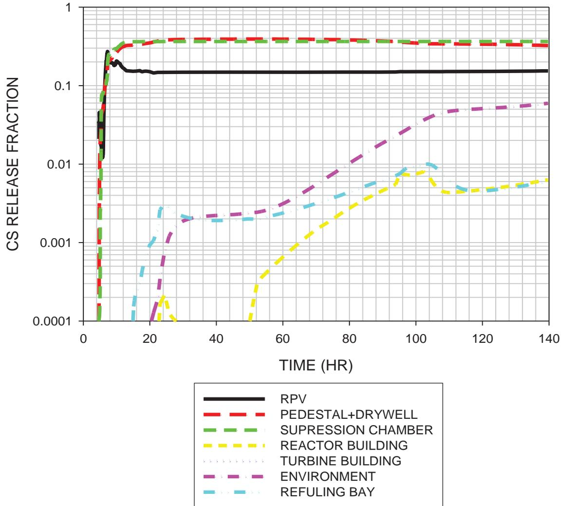
Figure 12. Cs Concentration in each Compartments (airbone + deposited on heat structures)
