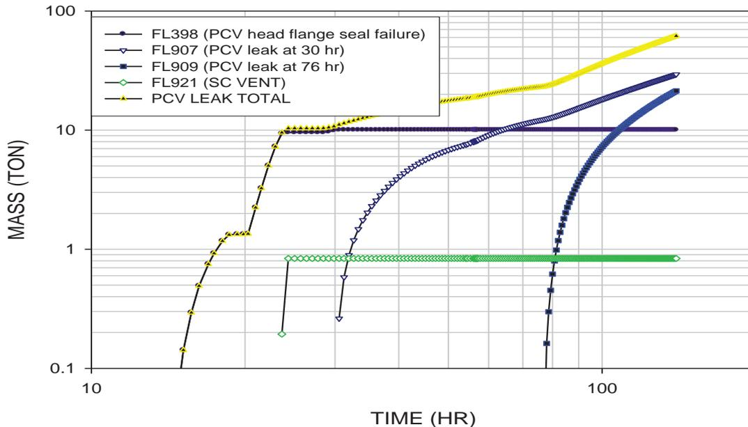
Figure 7. Integrated leakage masses from PCV to RB
