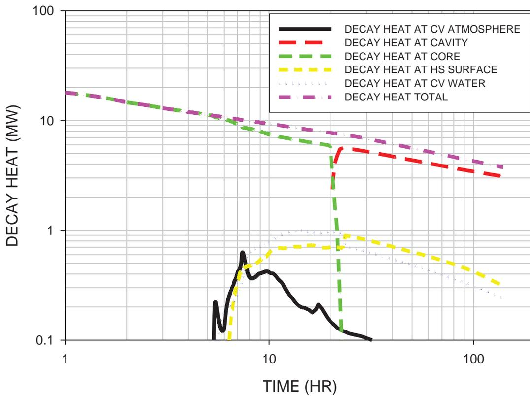
Figure 11. Distribution of decay heat to various places calculated by RN1 Package
