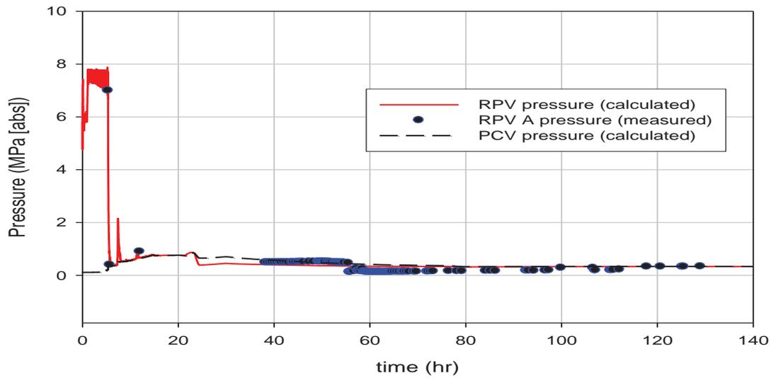
Figure 5. Pressure of RPV and PCV
