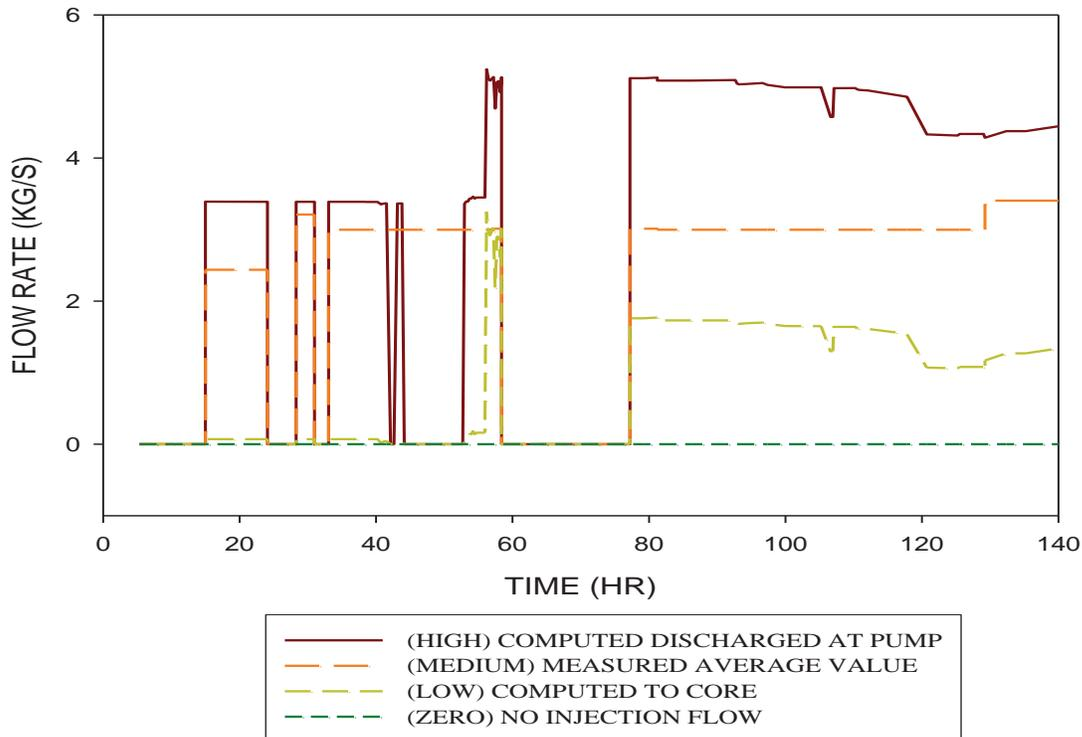
Figure 2. External water injection mass flow rate (kg/s)
