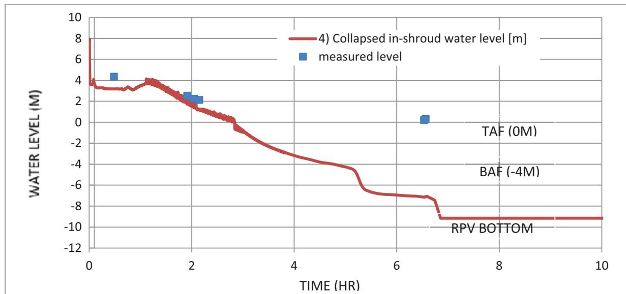
**Figure 4. Collapsed in-shroud water level (m)**
