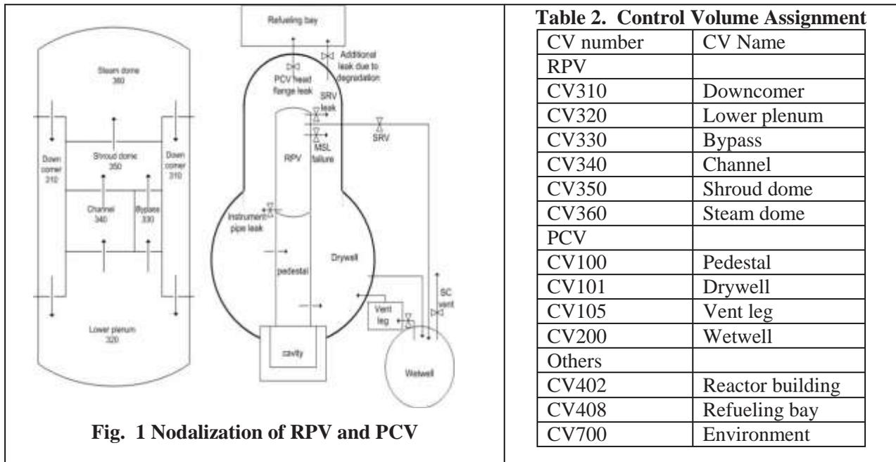
Fig. 1 Nodalization of RPV and PCV
