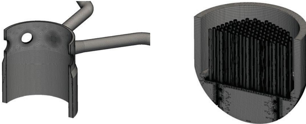
**Figure 3. Cross-sectional view of upper and lower RPV regions discretized with hexahedral cells.**
