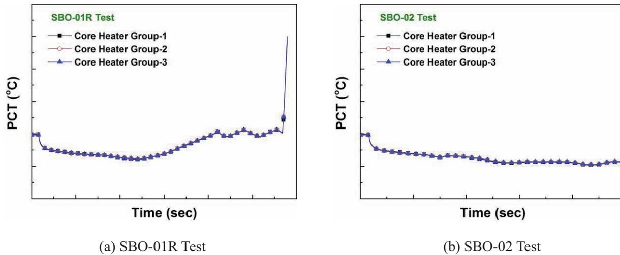
Figure 4. Variation of the core wall temperatures.
