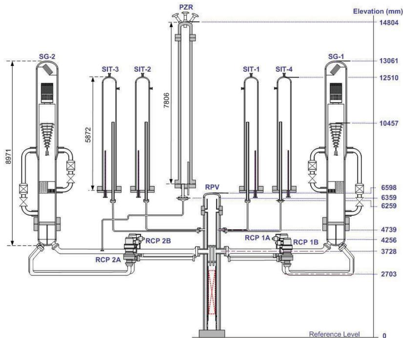
**Figure 1. Schematic diagram of loop connection of ATLAS.**
