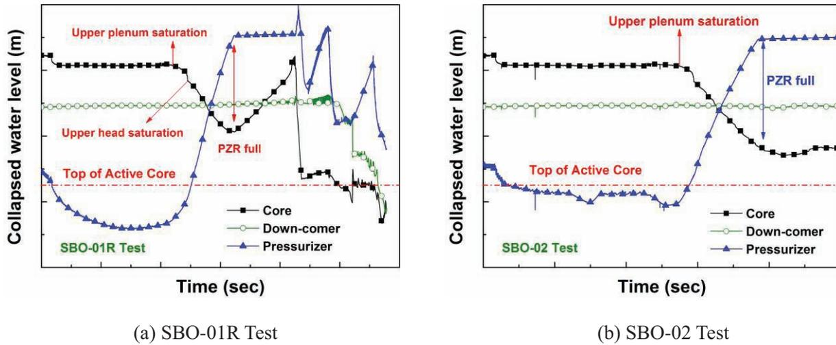
Figure 3. Variation of the collapsed water levels.
