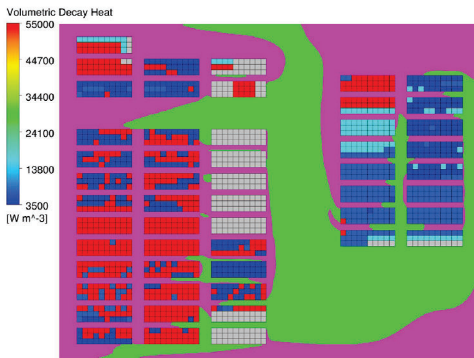
Figure 11. Developing Regions with a Downward Flow Direction (green) for a Complete Loss of Coolant. Flow with Upward Tendency Colored in Purple.
