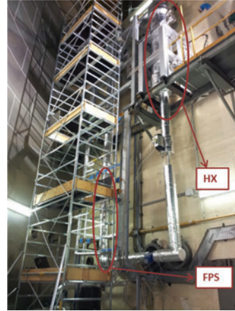
Figure 2.1: Configuration of the NACIE-UP facility
