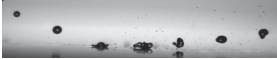
Figure 14: droplet-wall interaction in the bouncing regime (Weber < 40)
