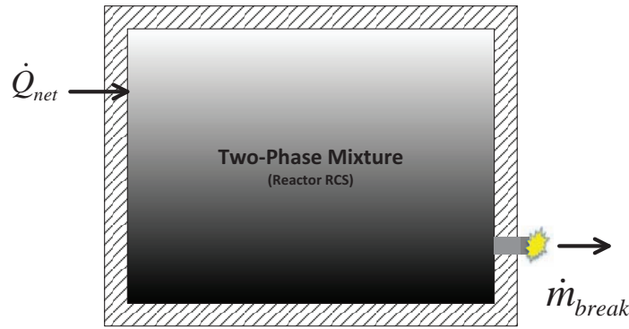
Figure 5. Schematic of control volume in the natural circulation phase.
